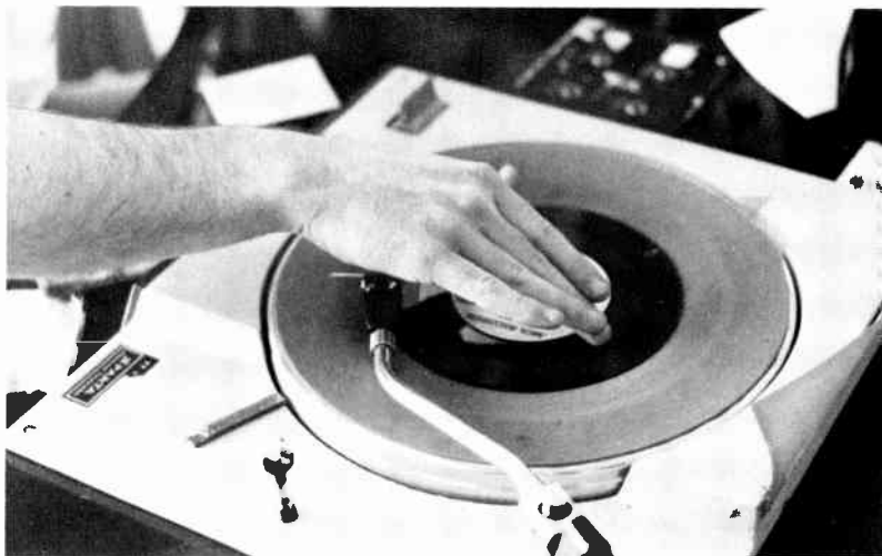
Figure 13.8 Cueing a 45-rpm record. Although disc jockeys frequently work exclusively with catted music, they should also be prepared to cue records on the turntable. (Courtesy KPLS, Santa Rosa, California)
