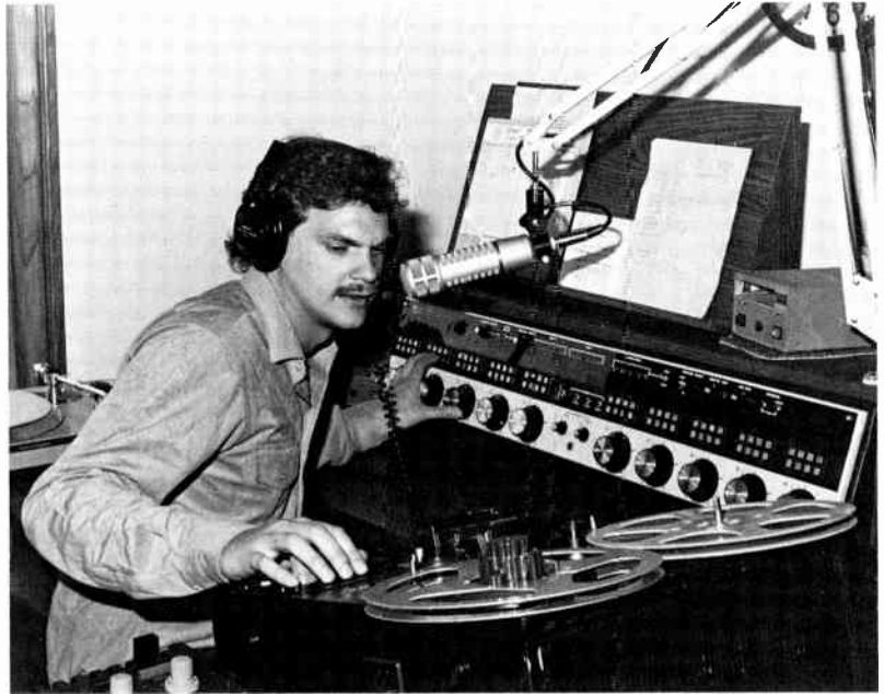
Figure 11.1 Production manager Joel Abrams prepares to record the voice portion of a commercial. He will later mix it with sound effects and music, then dub it to a tape cartridge. (Courtesy KTIM-FM, San Rafael, California)
