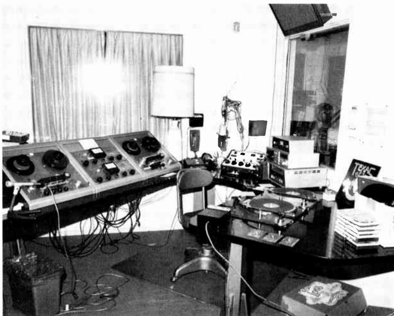
Figure 11.2 A well-arranged studio for the production of commercials. Equipment includes an RCA 77-DX microphone; Russco Cue-Master turntables; two Ampex reel-to-reel tape recorders; a Gates tape cartridge recorder and player; and a Sparta audio console. (Courtesy KPLS, Santa Rosa, California)
