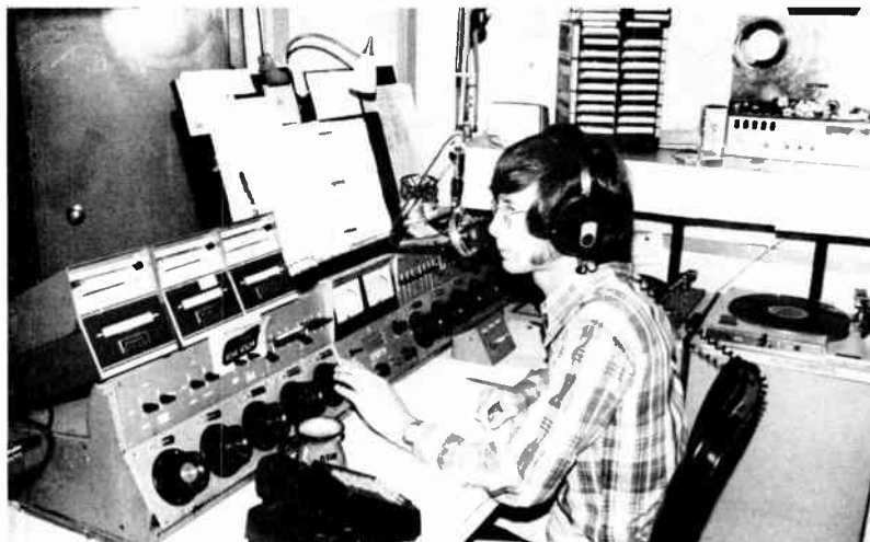
Figure 12.4 Clint Weyrauch, program director and air “personality” for KTIM, San Rafael, is shown during his regular air shift. He works a Gates stereo board, two Sparta turntables, and Sparta cart machines, and he speaks into an Electro-Voice 635A microphone. Before him are the running log (on counter top), and the copy or continuity book. (Courtesy KTIM, San Rafael, California)
