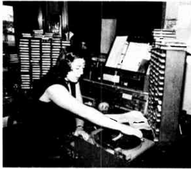
Figure 12.2 Janet Wooldridge cues-up a record on turntable 2, while turntable 1 plays the music being broadcast. (Courtesy KTOB-AM, Petaluma, California)
