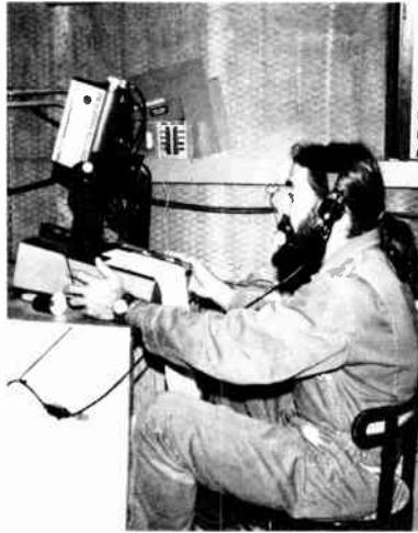
Figure 11.10 Greg Pace feeds a news script into a Q-TV “Video Prompter.” A vidicon camera transmits the script to the viewing device in front of the camera used by the newscaster. (Courtesy KPIX, San Francisco)
