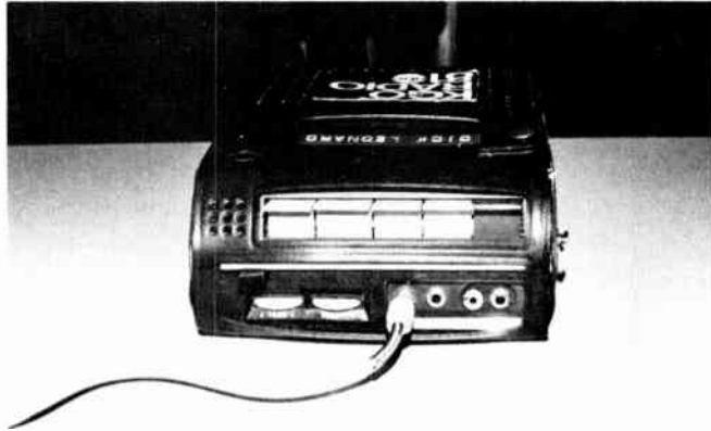
Figure 11.3 A cable, with a jack on one end and alligator clips on the other, connects a cassette recorder to the terminals of a telephone. This is one method of transmitting a story to a radio station.
