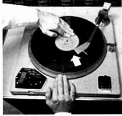
b. Spin the disc to find the first sound while holding the plate in place.
