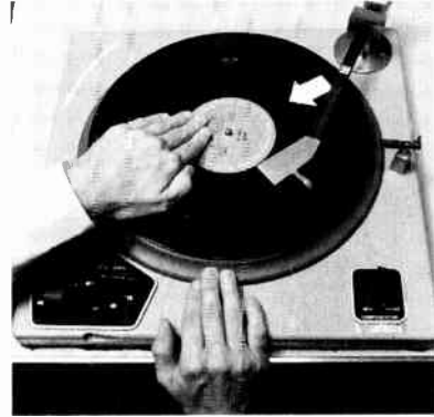
d. Backtrack the record. The turntable is in gear and all set to go.
