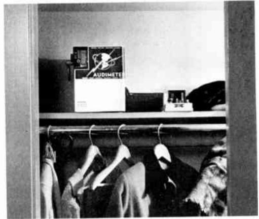
Figure 11-1 The Storage Instantaneous Audimeter (SIA) (left) has replaced the Audimeter (right), used for many years by A. C. Nielsen, which required the viewer to mail the information in. (Courtesy A. C. Nielsen Company)
