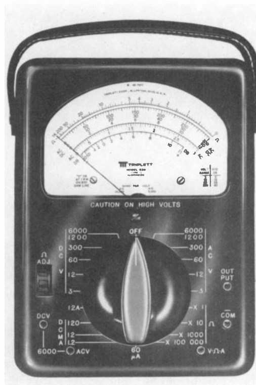
FIGURE 28-1 VOLT-OHM-MILLIAMMETER OR VOM. ACCURACY IS 2 PERCENT FOR DC MEASUREMENTS. (TRIPLET CORPORATION)
