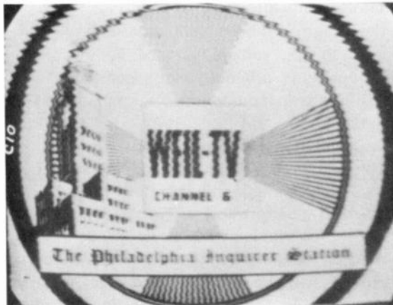
FIGURE 16-23 THE GEAR-TOOTH OR PIECRUST EFFECT IN PICTURE CAUSED BY HUNTING IN HORIZONTAL AFC CIRCUIT.
