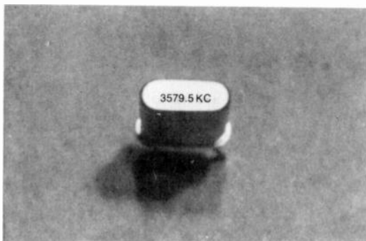
FIGURE 8-20 CRYSTAL FOR COLOR OSCILLATOR IN RECEIVER. HEIGHT IS 1 IN. FREQUENCY IS EXACTLY 3,579.545 kHz OR 3.579545 MHz.
