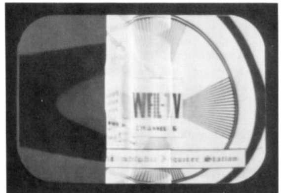
FIGURE 19-5 REDUCED WIDTH AND WIDE WHITE BAR AT LEFT, CAUSED BY OPEN B+ BOOST CAPACITOR.
