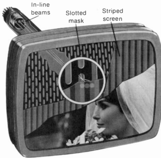
FIGURE 1-1 IMAGE ON FLUORESCENT SCREEN OF COLOR PICTURE TUBE IN TELEVISION RECEIVER. (RCA)
