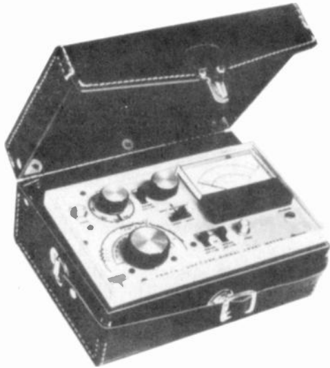
FIGURE 26-2 FIELD-STRENGTH METER. WIDTH IS 9 IN. (BLONDER-TONGUE LABORATORIES INC.)
