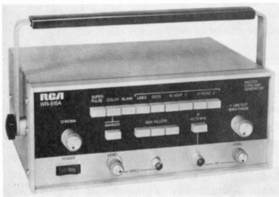
FIGURE 11-3 DOT-BAR SIGNAL GENERATOR. WIDTH IS 10 IN. (RCA)
