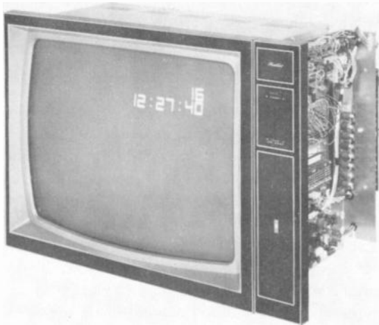
FIGURE 5-20 CHANNEL NUMBER 16, WITH EXACT TIME, REPRODUCED ON SCREEN OF PICTURE TUBE FROM ENCODED INFORMATION IN LINE 21 OF THE VERTICAL BLANKING INTERVAL. (HEATH COMPANY)
