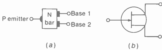
FIGURE 7-21 UNIUNCTION TRANSISTOR (UJT). (a) CONSTRUCTION. (b) SYMBOL.
