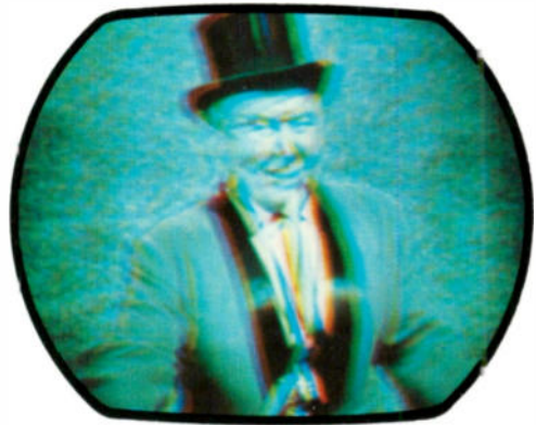
II COLOR FRINGING CAUSED BY POOR CONVERGENCE.
