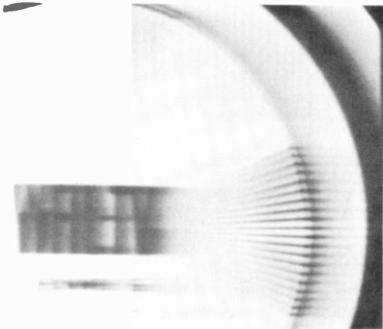
FIGURE 19-8 LOW-FREQUENCY SMEAR, WITH STREAKS AFTER LETTERING, CAUSED BY LEAKY COUPLING CAPACITOR IN VIDEO AMPLIFIER.
