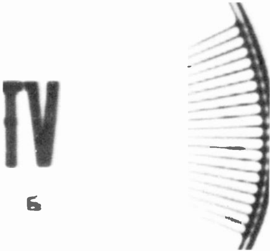
FIGURE 4-11 FAULTY INTERLACING. LINE DIVISIONS IN HORIZONTAL WEDGES ARE INTERWOVEN IN A MOIRÉ EFFECT.
