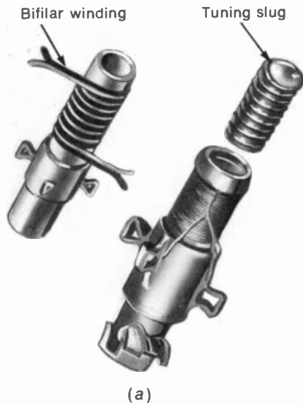
FIGURE 23-12 BIFILAR IF COIL. (a) PHOTO; HEIGHT ABOUT 1\frac{1}{2} IN.; (b) SCHEMATIC SYMBOL.
