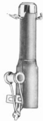
FIGURE 13-35 TYPICAL 4.5-MHz TRAP WITH L AND C . HEIGHT IS 1\frac{1}{2} IN.
