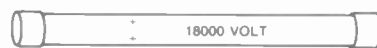
FIGURE 7-10 SILICON-DIODE STICK FOR HIGH-VOLTAGE RECTIFIER. LENGTH IS 3 IN. CATHODE END MARKED + FOR DC OUTPUT.
