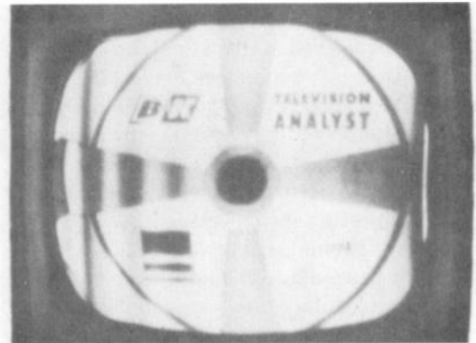
FIGURE 22-34 EXCESSIVE YOKE RINGING.
