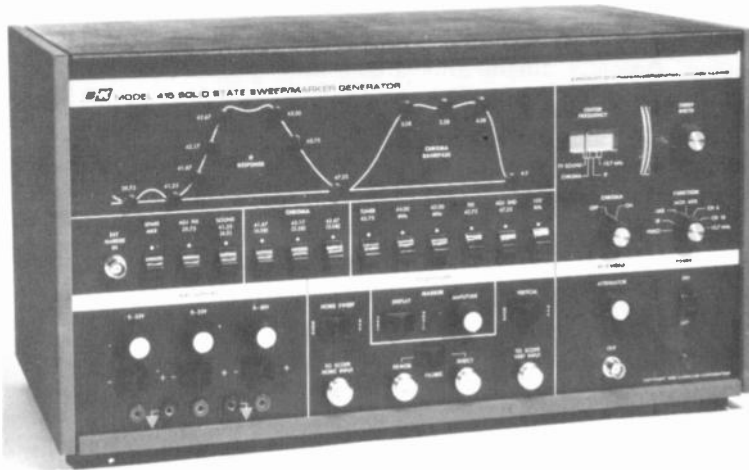
FIGURE 23-22 TYPICAL SWEEP GENERATOR FOR RF, IF, AND VIDEO RESPONSE CURVES. (B AND K DIVISION OF DYNASCAN CORP.)
