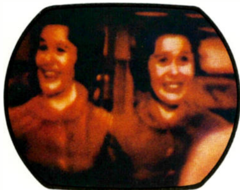
XIV SILVERY EFFECT IN HIGHLIGHTS OF PICTURE BECAUSE OF LOW EMISSION. ILLUSTRATED FOR RED GUN ALONE. (RCA)
