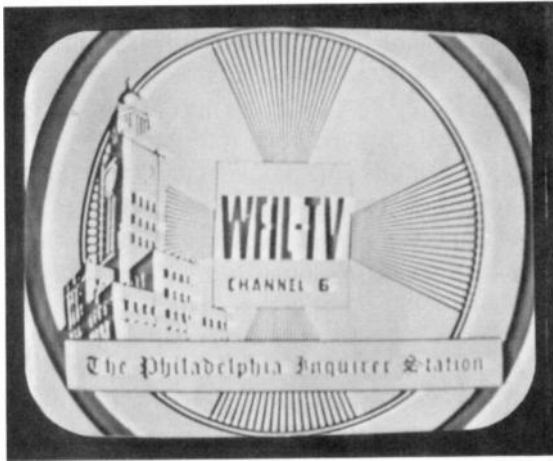
FIGURE 13-14 TEST PATTERN ILLUSTRATING LOSS OF LOW VIDEO FREQUENCIES. BACKGROUND IS WEAK, AND LETTERING IS NOT SOLID. SIDE WEDGES HAVE WEAKER INTENSITY THAN TOP AND BOTTOM WEDGES. (RCA PICT-O-GUIDE)
