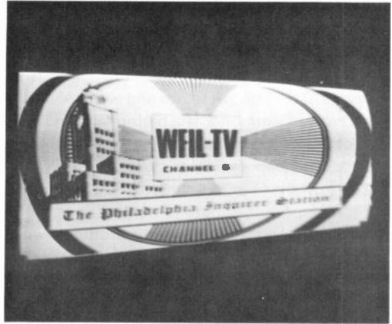
FIGURE 19-6 TRAPEZOIDAL RASTER, CAUSED BY DEFECTIVE YOKE.
