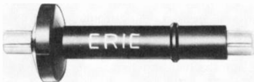
FIGURE 12-34 SILICON HIGH-VOLTAGE RECTIFIERS FOR COLOR RECEIVERS. (a) 30- TO 45-kV RATING FOR ANODE VOLTAGE OF CRT. LENGTH IS 4 IN. THIN END AT RIGHT IS CATHODE SIDE. (b) 5- TO 10-kV RATING FOR FOCUS VOLTAGE. LENGTH IS 2 IN. (ERIE TECHNOLOGICAL PRODUCTS, INC.)
