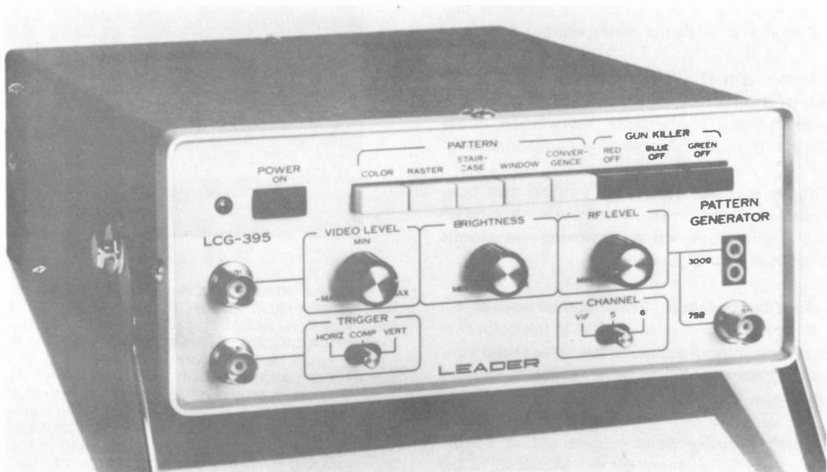
FIGURE 28-12 TYPICAL DOT-BAR GENERATOR. NOTE PATTERNS AVAILABLE FROM TOP ROW OF SWITCHES. (LEADER INSTRUMENTS CORP.)
