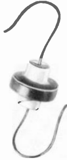
FIGURE 13-21 TYPICAL VIDEO PEAKING COIL. WIDTH IS 1/2 IN. L IS 180 \mu H.
