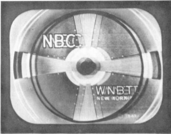
FIGURE 19-13 GHOST CAUSED BY REFLECTED SIGNAL AT ANTENNA.
