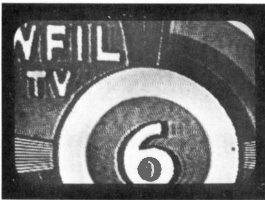
FIGURE 13-34 FINE HERRINGBONE WEAVE PRODUCED BY 4.5-MHz INTERCARRIER SOUND IN PICTURE.
