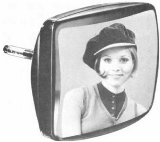
FIGURE 1-5 COLOR PICTURE TUBE TYPE NUMBER 18VATP22. THE P22 INDICATES SCREEN WITH RED, GREEN, AND BLUE PHOSPHORS. (ZENITH CORPORATION)
