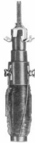
FIGURE 22-14 COIL FOR WIDTH OR LINEARITY CONTROL. L IS 2 TO 18 mH. R IS 14 \Omega .
