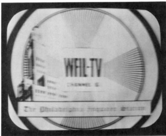
FIGURE 13-13 TEST PATTERN ILLUSTRATING LOSS OF HIGH VIDEO FREQUENCIES. NOTE LACK OF SEPARATION FOR THE LINES IN TOP AND BOTTOM WEDGES. ALSO, THEY HAVE WEAKER INTENSITY THAN THE SIDE WEDGES. (RCA PICT-O-GUIDE)
