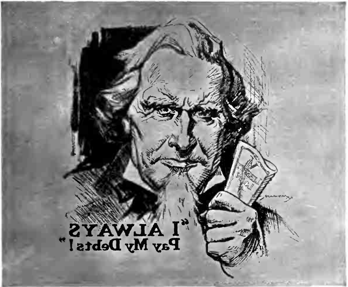
FIG. 4.—Zinc plate as it appears with the photographic image on it.
