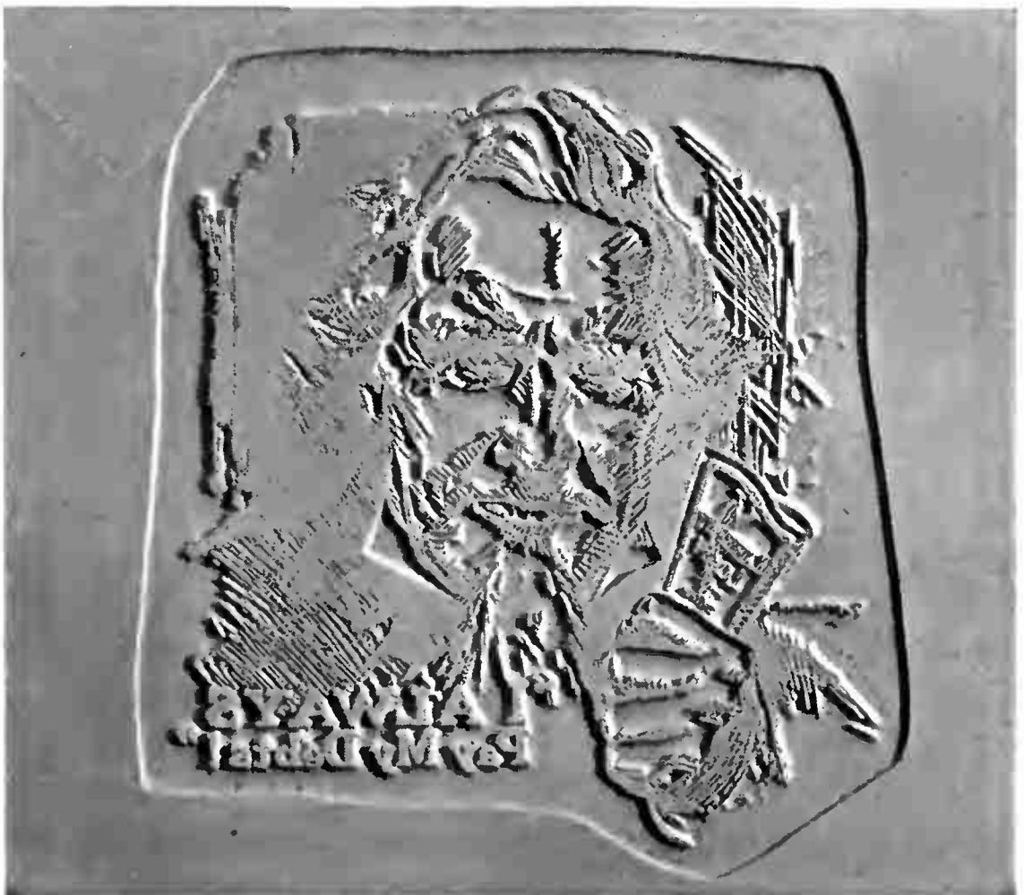
FIG. 5.—The zinc plate after receiving the acid bath.
