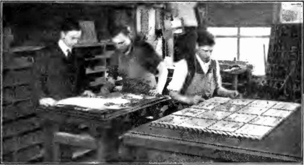
FIG. 10.—Magazine make-up scene. Plates are shown on a patent block.
