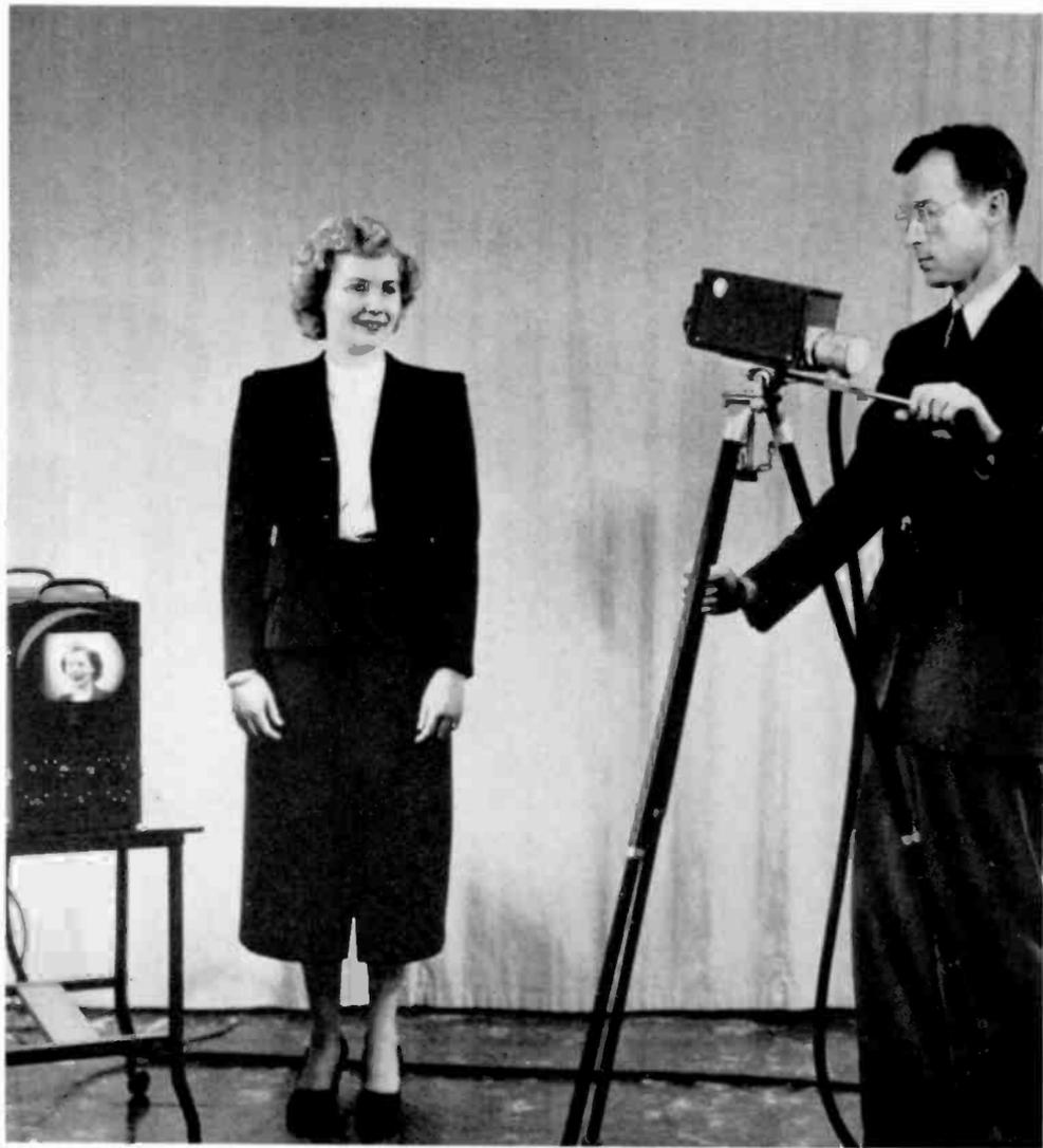
The Vidicon in use. Ensnared in a small camera, it produces the clear well-defined image seen in the portable monitor on the nearby table.
