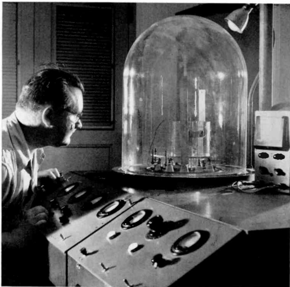
No other modern commercial industry leans so heavily on pure science as does television. Photo shows RCA scientist conducting an electronic research experiment on the evaporation of metals inside a vacuum chamber.
