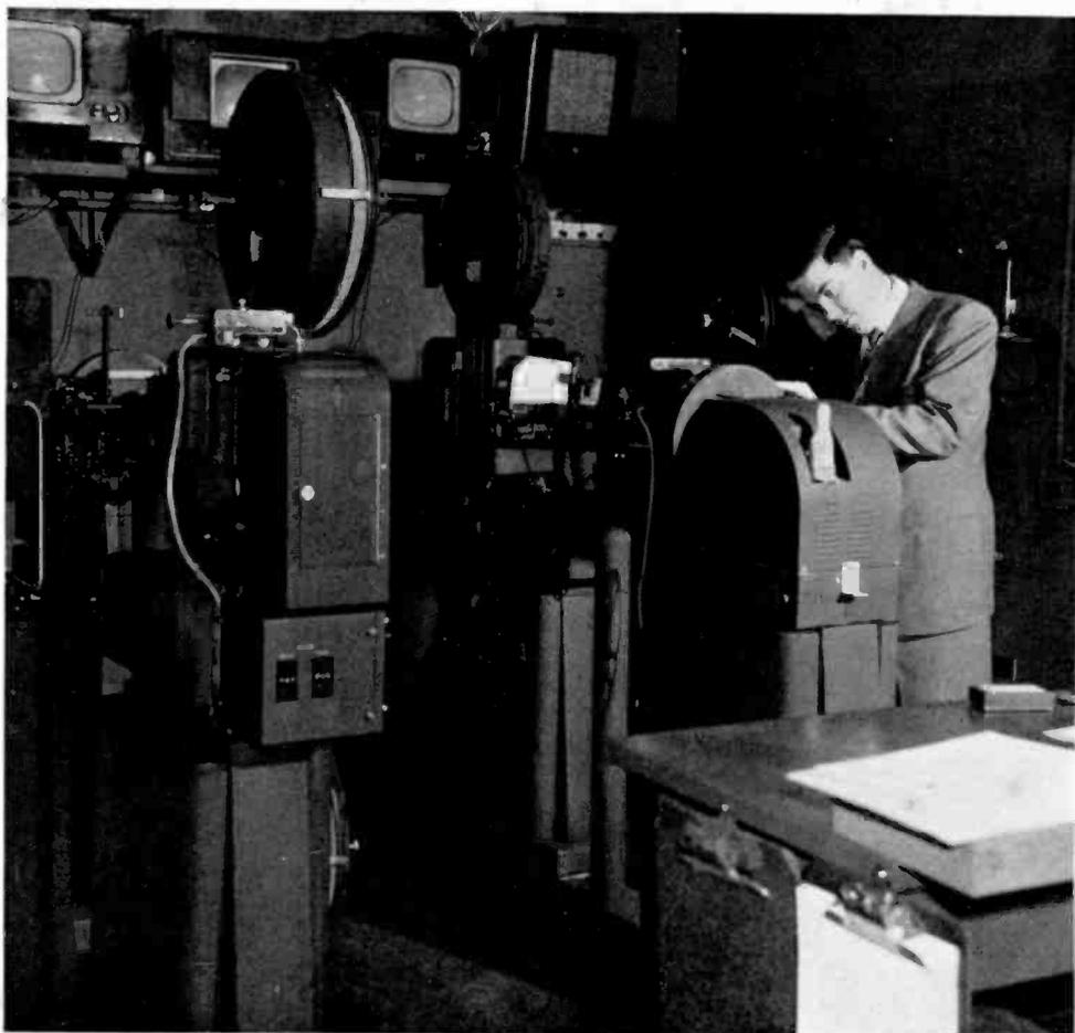
Kinescope recording equipment used in televising motion-picture film. Much fine entertainment and information are provided on our TV screens through the medium of film, new and old.
