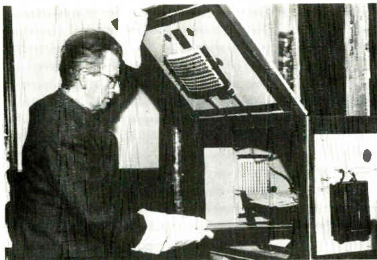
Baird in his Sydenham garage heat-treating hand-made cathode ray tubes, 1944.
