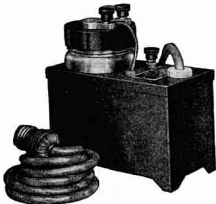
FIG. 13.—Globe Silite trickle charger. This charger uses the new metallic glass element, silite, adapted to storage batteries preferably not over 60 ampere hour capacity. This combination will meet the requirements up to six or eight tube sets which are not used on an average of more than four hours a day. Charges at .6 to .75 ampere rate and may be used with either 4 or 6 volt batteries.
