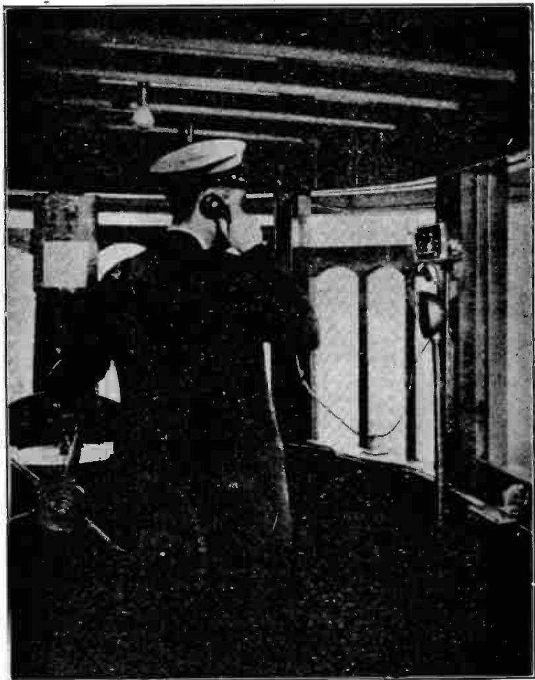
FIG. 4—Marine Radio Telephone Control equipment within easy reach of the pilot. (Courtesy Western Electric Co.)
