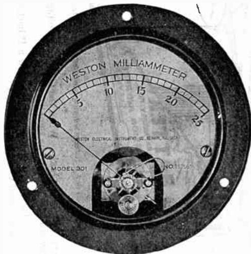
FIG. 3.—Weston plate or grid milli-ammeter for measuring the plate current of vacuum tubes. It will give a deflection for steady or pulsating direct current and will indicate the average value of a pulsating current. Superimposed upon the steady plate current is the current due to the modulation which is an alternating current and will cause the total plate current to be a pulsating current varying at the same frequency as the modulation current. The milli-ammeter will again indicate the average value of this current and if the tube be working at a point where it rectifies, this average value will not be the same as the value of the unmodulated steady plate current and therefore fluctuate with the modulation. For perfect reproduction, amplifying tubes should not rectify and no variation in the indication of the milli-ammeter should occur. In practice however, on account of the properties of vacuum tubes, some rectification will result, but by properly adjusting the grid bias, a minimum fluctuation in the plate current may be obtained consistent with good quality and volume.
