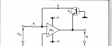
Fig. 1. Simple logarithmic circuit.
