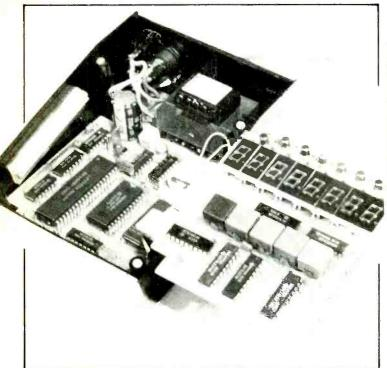
The instrument, based on a Z80 processor with 2K of ram, uses low-cost components thhroughout. The same hardware could be used to implement a general i/o controller, for example in a security installatioon or central heating system.
