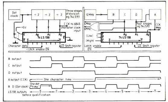
corresponding dot time. A switch selects output activity during either the high or low pulse of the dot clock. Alternative qualifying signals may be applied to the enable inputs.
