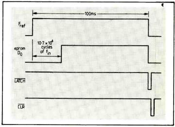
the count to be recognized which in turn controls a gate between the incoming signal and the frequency counter. For example, if an offset of 10.7MHz is required then all locations from 0 to 106 are filled with zeros and remaining locations are left at FF.
