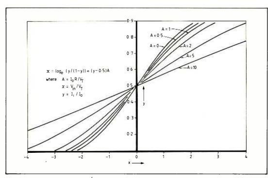
Fig. 8. Linearized long-tail pair transfer characteristic.
