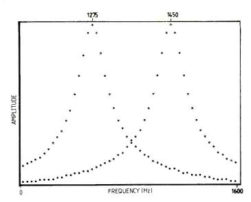
Fig. 5. Actual response of bandpass filters for 170Hz shift (50 bits per second) using the new tone standard as predicted by computer modelling.
