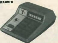
This unit provides simple, reliable programming of up to 8 EPROMS simultaneously. It has been designed for ease of operator use — a single 'program' key starts the self check — blank check program - verify sequence.
