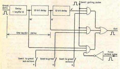
Fig. 4. Coupling between manuals is achieved by lengthening delays so that delayed data occurs at the right place in the scan.
