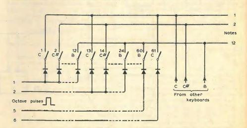
Fig. 2. Identical notes are wired together on one side of matrix, with all 12 notes in each octave wired together via diodes on the other side.
