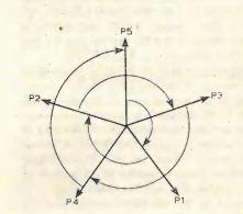
Fig. 3. Spoke diagramfor a 5-phase oscillator, m=5, n=2. Phase separation is 72° and the sequence is P5-P3-P1-P4-P2.
