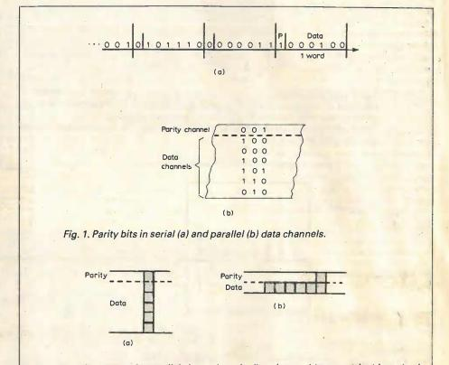
Fig. 2. Checking area of a parallel channel can be 'bent' to enable one parity bit to check serial data as in (b).
