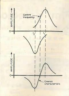
Fig. 4. Derivation of overall characteristic of Round-Travis f.m. detector.
