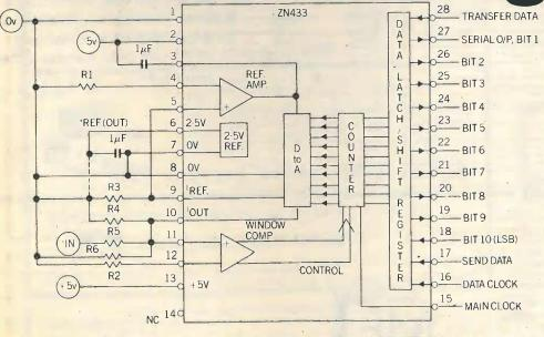
ZN433 is a monolithic 10-bit tracking ADC with onchip 2.5 volt precision reference and is ideal for continuous tracking of analogue signals.
