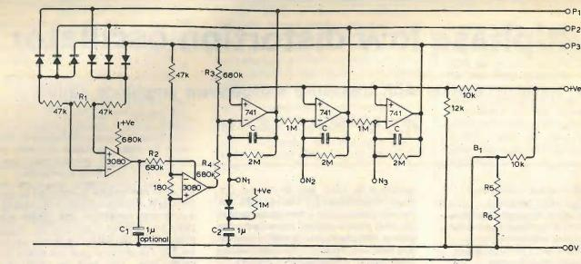
Fig. 4. Three-phase oscillator. f=0.3Hz with C=0.47μF.
