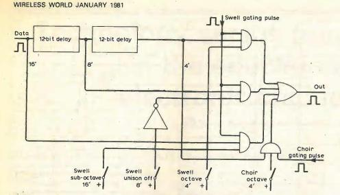
Fig. 3. As scanning is sequential note-by-note and octave-by-octave, 12 pulses separate keys an octave apart, and octave coupling is achieved using 12 pulse data delays.
