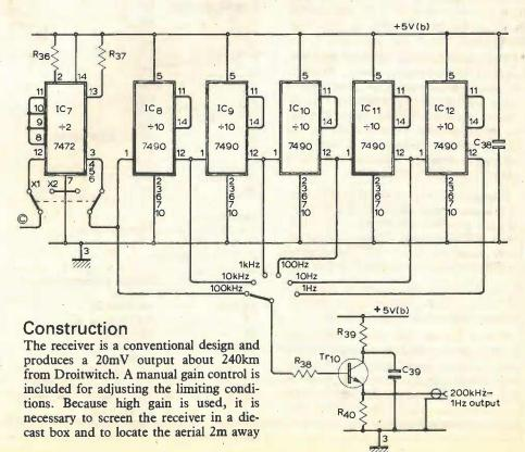
Adjustment of the receiver should be carried out using an oscilloscope to observe the waveform before the limiting stages. The aerial trimmer and each tuned stage is set to resonance so that the a.m. envelope is at a maximum. If the envelope amplitude is unstable and does not exhibit normal modulation variations, the receiver is probably oscillating and the feedback source should be investigated. The gain control is adjusted to give 10V pk-to-pk free from amplitude variations?
