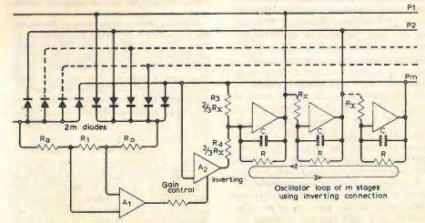
Fig. 1. Oscillator of m phases.
