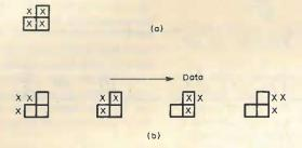
Fig. 3. Two, three and four errors, distributed as at (a) are detected, since the parity check gives an odd result at some point as the data stream passes the checking area. The pattern at (b) is not detected, because the parity remains even at any position.
