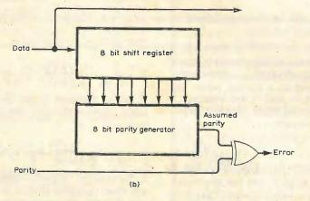
Fig. 4. Logic diagram of parity generation and checking.
