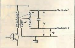
Fig. 5. Method of deriving the two diode inputs in Seeley-Foster and ratio detectors.
