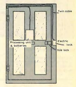
Fig. 2. If the Yale and solenoid locks are mounted as shown here, the door can be opened either by using the key or the combination-lock keyboard.
