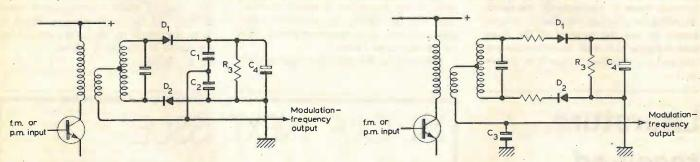
Fig. 10. The circuit of Fig. 9 (b) modified so as to give a measure of a.m. rejection.
