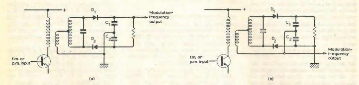
Fig. 9. Simplified circuits for (a) balanced and (b) unbalanced forms of ratio detector with no provision for a.m. rejection.
