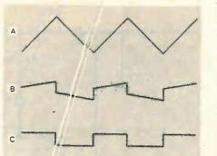
Fig. 5. The effect of adjusting  $RV_2$  for differential balance. Triangular-wave input at (a) shouled produce square-wave output, as at (c).
