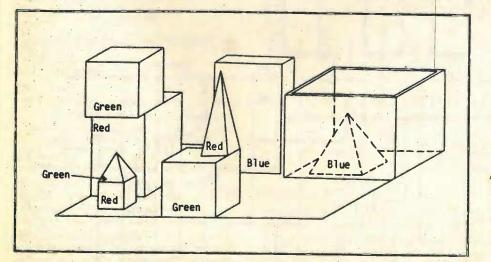
Fig. 3. Winograd's simple world for understanding natural language. A screen displays these blocks, each of which has a word printed on it indicating a colour.
