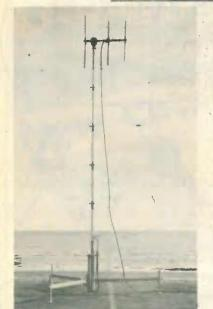
Telescopic air operated Clark Mast Type QT4m/HP mounted on portable tripod.
