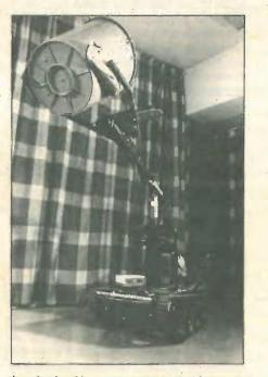
In robotics Al systems are needed for recognising objects. This mobile robot developed at Warwick University has sensory equipment enabling it to avoid obstacles and to seek out, approach and grasp an object such as the plastic bin shown.
