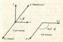
Fig. 2. Vector diagram for second oscillator stage.
