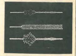
Traces illustrating loudspeaker-room interaction with or without an equaliser. The middle trace is the input tone burst. At the bottom is the room response without an equaliser; at the top the response with an equaliser. Note how the equaliser fails to compensate for envelope distortion and hence timbre and character. (Timebase 20ms/div.)
