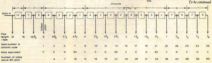
Normal (unison) pitch is delayed by two octaves Fig. 6. Shift register can be tapped at necessary increments and simple gating controls appropriate frequencies from generators or pipes. (See part 2, Fig. 7, for simplified control system.)
