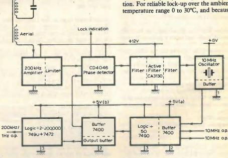
Fig. 1. Block diagram.
