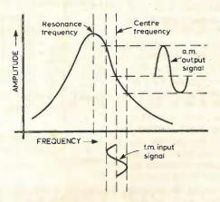
Fig. 2. Simple f.m. slope detector.
