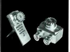
Adaptors are available to convert the block terminals or coaxial sockets of the B201 to the 14mm International Standard connectors, GR900. These permit the B201 calibration to be referred to internationally recognised standards.
