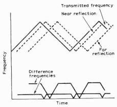
Fig. 1. Transmitted and received signals in an f.m.-c.w. radar. Near target produces low difference frequency and a distant target a higher difference frequency.
