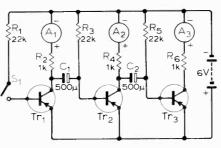
Circuit for demonstrating astable multivibrator action. Meters are 0-10mA types.
