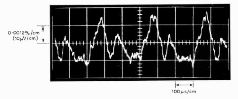
Fig. 5. Null method of assessing amplifier distortion shows distortion products to be well down in the noise. Deflection of 4cm represents 0.003% peak distortion at 10 watts (3kHz,  $15\Omega$  load).
