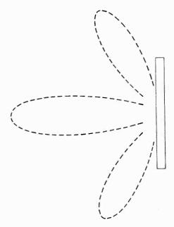
Fig. 3. Example of unwanted lobes due to physical spacing between units.
