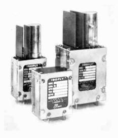
noiseless in floating circuit application. Novel construction of the transformer, and special mounting of the rectifiers, filter elements, and regulator, plus electrostatic shielding, greatly reduce the generation and transference of noise, while providing good isolation between the output circuitry and the combination of input and ground (core case and primary shield). Aveley Electric Ltd, Arisdale Avenue, South Ockendon, Essex.
