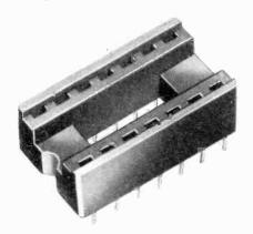
phosphor bronze, gold plated over nickel. Typical contact resistance is  $5m\Omega$  for type Z,  $10m\Omega$  for type Y. Price range from 15p for 500 up. Jermyn Industries, Vestry Estate, Sevenoaks, Kent.
