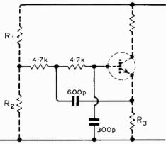
Fig. 1. Low-pass filter for use when noise is a problem. Existing components are shown dotted.
