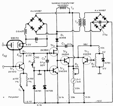
Fig. 4. Diagram of the automatic balance circuit.
