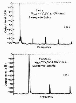
Fig. 4. Spectra made with a wave analyser showed no difference between spectra of outputs from oscillator and amplifier. Plots were made with (a) 1kHz and (b) 10kHz signals and were identical at all three power levels.
