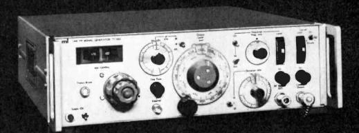
The TF 2012 is the first of 'the quiet ones' – a series of signal generators designed to embody all the features needed for the accurate evaluation of narrow band mobile FM receivers. It is a signal generator with sufficiently low sideband noise to permit – with ease – the exacting two and three signal generator tests required by the licensing authorities on advanced mobile equipment. It has extremely low microphony and its frequency
