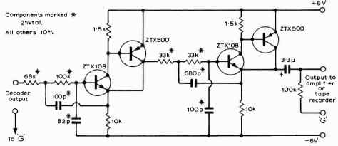
Fig.1 Decoder earth may be 0V or -6V depending on supply rail choice. Filter earth 'G' is independent and therefore may be either.
