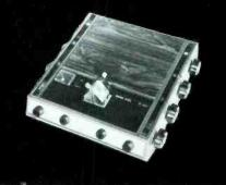
Precision RF Bridge measures capacitance to 0.1% accuracy, conductance to 0.2%. Operation centred on 1MHz but high performance is maintained from 100kHz to 5MHz. Plug-in source/detector units. AC or battery operation.
