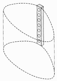
Fig. 2. Idealized distribution pattern for line-source system.
