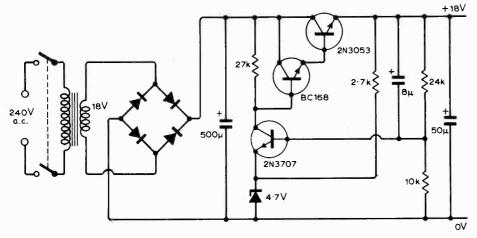
Fig. 6. The circuit of the power supply unit.
