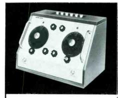
Radio Frequency Bridge with its Low Impedance Adaptor reads a wide range of L, C and R values at frequencies from 15kHz to 5MHz, generally to 1%. Special Adaptors, Q601 series, for measuring transistor parameters. Two or three-terminal connections, balanced or unbalanced.
