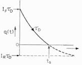
Fig. 15. Variation of excess minority charge with time. Switch opens at q = 0.
