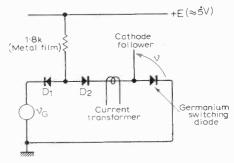
Fig. 11. Practical circuit for opencircuiting test on germanium switching diode. Diode current and voltage waveforms are observed with a current transformer and a high-impedance cathode follower feeding a sampling oscilloscope.
