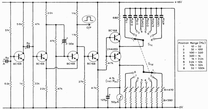
Fig. 5. Frequency meter and square-wave shaper.
