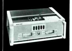
Universal RF Bridge measures real and quadrature terms of any immittance to 1%. without frequency dependence, from 100kHz to 10MHz. Includes standards of R, C and L. Unique magnetic potentiometers give exceptional linearity and stability.
