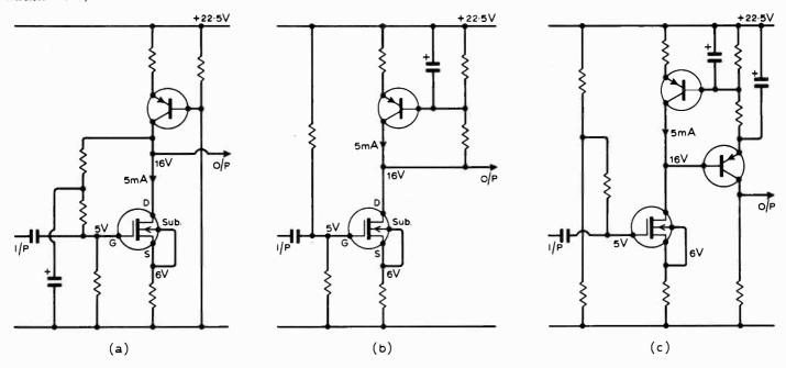
Fig. 2. (a and b) Two ways of stabilizing the voltage on the collector and drain of the constant current transistor and m.o.s.f.e.t. (c) the solution employed.
