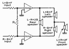
A method of using a derived centre channel to produce four channels (Dynaco patent No. 3,417,203).
