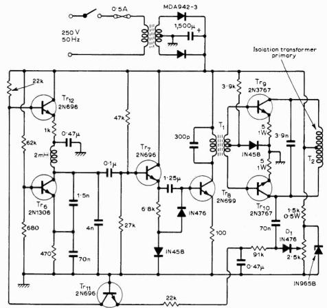
Fig. 5. Circuit diagram of the power oscillator. The 70nF capacitor is  $C_1$ .
