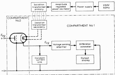
Fig. 3. Block diagram of the valve voltmeter, showing the two internal compartments.
