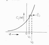
Fig. 6. Non-linearity of depletion capacitance  $C_j$  can be linearized by finding average volume of  $C_j$  graphically.
