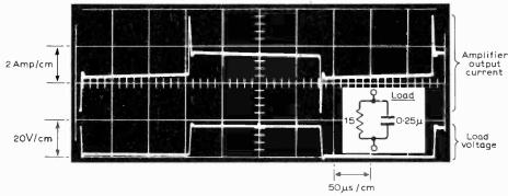
Fig. 9. Performance with a capacitative load. Capacitor in feedback loop effectively reduces maximum rate of change of voltage across load. Overshoot is much less when fed from a pre-amplifier.
