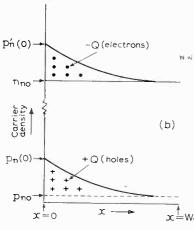
Fig. 3. (a) In long-base diode ( $W_N \gg L_H$ ) excess minority carriers recombine before reaching contact and curve decays exponentially. (b) Injected holes (charge +Q) in n region are matched by injection of electrons to amount -Q.
