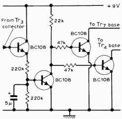
Fig. 2. Circuit to switch-off the decoder when a mono signal is being received.
