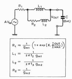
Fig. 8. Power amplifier equivalent circuit. Simple analysis shows output impedance is controlled by main feedback loop, but in practice  $R_6$  generates another loop effectively placing a damping resistance across the apparent output inductance.
