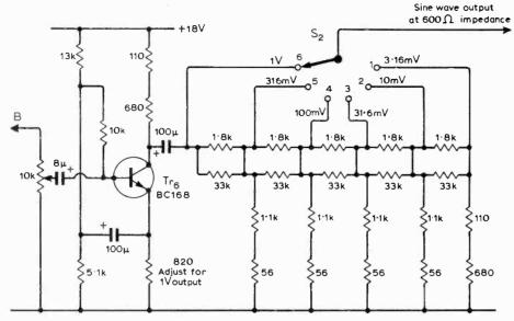
Fig. 4. Output attenuator circuit.
