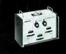
VHF Admittance Bridge covering 1MHz - 100MHz measures conductance from 0 — 100 millimhos and susceptance from —230pF to +230pF, with an accuracy of 2%. Two or three-terminal connections, balanced or unbalanced. Adaptor Q801A for transistor parameters.
