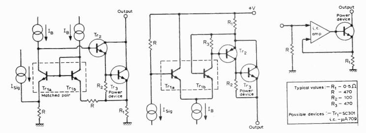
Fig. 11. Proposals for integrated components in output sub-amplifier.
