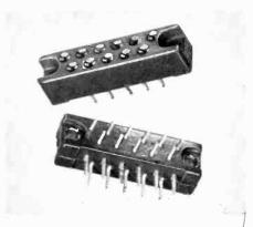
$10 m \Omega$  max. and an insulation resistance of  $1000 m \Omega$  at 500 V d.c. The body moulding of the connectors is of an epoxy resin. Pins are of gold-plated brass and the sockets are manufactured from gold-plated beryllium copper. Henry & Thomas Ltd, Yeo Street, Bow Common, London E.3.
