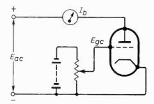
Fig. 1. Basic circuit diagram showing the principle of the voltmeter.
