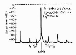
Fig. 6. Result of feeding 5kHz and 200Hz signals in a 16:1 power ratio into amplifier. Intermodulation products  $f_1 + f_2$  and  $f_1 - f_2$  are 90dB below 200 Hz signal. Other spectral lines are due to generator distortion.
