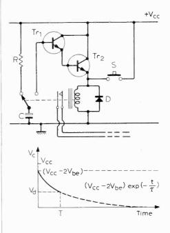
Normally C is charged to  $+V_{cc}$  until switch S is momentarily closed. This causes the relay to 'pull-in' and C is connected to the base of the super- $\alpha$  pair,  $Tr_1 Tr_2$ , which form a very high impedance emitter-follower. C discharges slowly due to base current, and the voltage at the emitter of  $Tr_2$  falls from  $V_{cc}$ - $2V_{be}$  to  $V_d$ , the relay 'drop-out' voltage, at which point the relay
