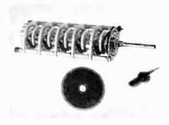
to five positions. Contacts are placed 20° apart. Contact springs and terminals are silver plated. Up to 20A can be handled at 12V, and switching life is typically 25,000 cycles minimum. Ultra Electronics (Components) Ltd, Fassetts Road, Loudwater, Bucks.
