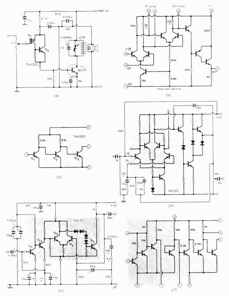
Fig. 1. Typical commercial a.f. low-level amplifier monolithic microcircuits: (a) TAA 320 two-stage m.o.s.f.e.t. input pre-amplifier in 2W crystal pickup record player; (b) TAA 263 three-stage general purpose 7V pre-amplifier; (c) TAA 310 four-stage high-gain pre-amplifier in tape playback system; (d) MC 1303P five-stage dual pre-amplifier; (e) PA 230 four-stage low-level amplifier in 'flat' pre-amplifier; (f) TAA 370 five-stage high-gain pre-amplifier.
