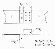
Fig. 2. Charge distribution in depletion region.
