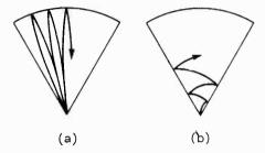
Fig. 2. Two azimuth scanning systems (a) mechanical and (b) electronic. In the electronic system scanning is achieved by using an aerial whose radiation pattern changes with frequency.
