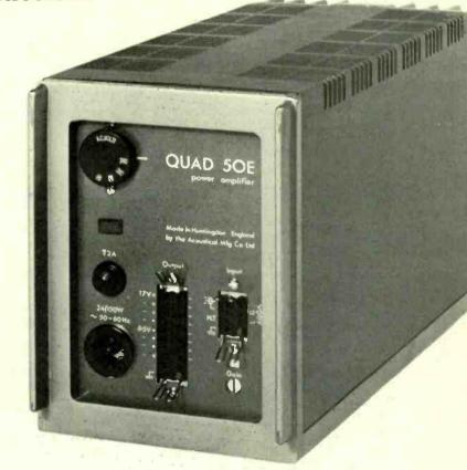
**INPUTS** – 0.5 Vrms unbalanced with provision for an optional plug-in transformer for bridging 600 ohms lines. **OUTPUTS** – isolated providing 50 watts into almost any impedance from 4 to 200 ohms. **DIMENSIONS** –  $12\frac{3}{4}$ " x  $6\frac{1}{4}$ " x  $4\frac{1}{2}$ "
