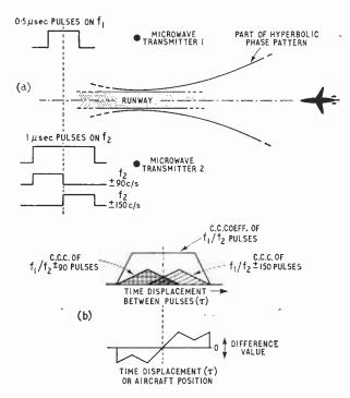
Fig. 1. Principle of R.A.E.'s correlation-protected I.L.S.: (a) localizer transmission; (b) cross-correlation in aircraft receiver.
