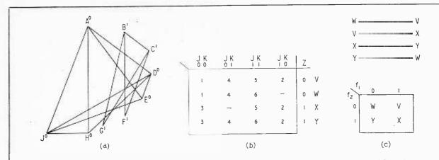
Fig. 13. (a) Merger diagram for Fig. 12, each line connecting two rows which could be merged. (b) Merged flow table. (c) Transitions and transition map.
