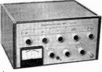
RC oscillator with a frequency range of lc/s to IMc/s shown by Alcate!.
