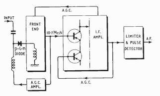
Fig. 3. Wide dynamic range of 120 dB of the Fisher TFM-1000 tuner is achieved by use of three a.g.c. loops, one using a p-i-n diode.
