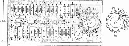
Fig. 5. Suggested layout for amplifier 2 and range switch panel.
