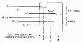
Fig. 2. Arrangement of voltage drives to cathodes and grids of threegun, shadow-mask colour picture tube to ensure that grid-cathode on each gun sees only appropriate R, G, or B drive voltage on colour transmission and only luminance, Y, on monochrome transmission.
