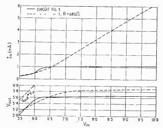
this case it was set to  $1 \text{ mA. } R_1$  is necessary for "starting" the circuit, otherwise with low leakage in Tr3 there may be no current in Tr1 and Tr2 (see reference to "bistable" action, September, 1966).
