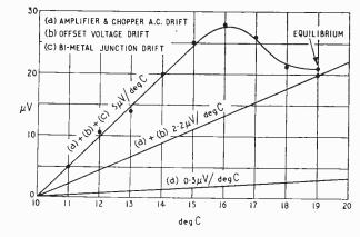
Fig. 2. Temperature characteristic of Fig. 1 circuit when subjected to a sudden rise of 9 deg C ( $R_s$ --1 k  $\Omega$ ).
