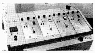
**Insertion of sound effects** into television and sound programmes is simplified by this "programme effects generator" just introduced by the B.B.C. The effects are recorded in specially developed matchbox-size tape cassettes, each giving 30 seconds playing time. Four reproducing channels are provided. Tape playing speed can be continuously varied, for example to alter the pace of footsteps.
