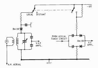
Fig. 2. Local-distant switching on the new Goodmans tuner can give a gain reduction of 20 dB.
