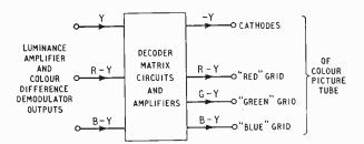
Fig. 3. Function of colour decoder section in converting three video signals Y, R-Y and B-Y into four corresponding signals, Y, R-Y, G-Y and B-Y needed to drive colour tube.
