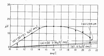
Fig. 3. Effect of substituting a thermistor for R4 in Fig. 1 and subjecting circuit to a 11 deg C rise  $(R_s = 1 k \Omega)$ .
