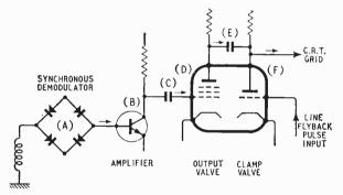
Fig. 6. Basic arrangement for preserving d.c. levels in colourdifference decoder channel.
