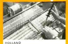
Ersin Multicore 5 Core Solder is used for soldering printed circuit boards by N. V. Eminent, Bodegraven, Holland.
