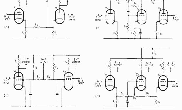
Fig. 4. Colour matrix basic decoder circuits that have been used in American commercial receivers: (a) double-triode, cathode-matrixing; (b) three-triode, anode-matrixing; (c) double-pentode, screen-matrixing; (d) three-triode, cathode-matrixing.
