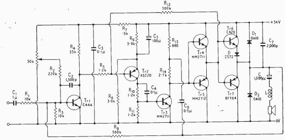
Circuit of SW class D amplifier using configuration 2.
