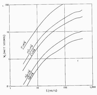
Fig. 2. Energy-storage capacity of currently available aluminium electrolytic capacitors.
