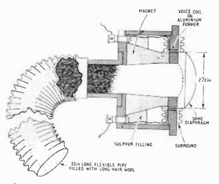
Fig. 1. KEF's new mid-range loudspeaker with absorbent load.
