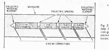
Fig. 2. Four-element latching digital phase shifter.
