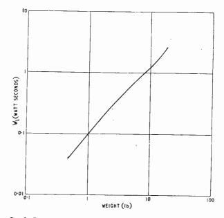
Fig. 5. Energy-storage capacity of an inductor (about 0.1 watt sec/lb)
