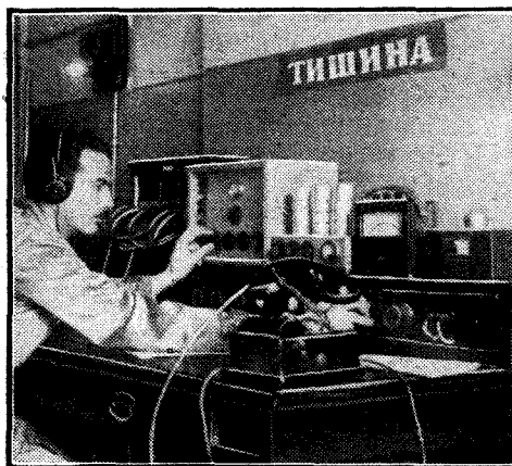
RADIO-BELGRADE II. —A low-powered short-wave transmitter, adapted to the needs of broadcasting by the Government Press Department, and used for the transmissions of programmes intended for countries outside Yugoslavia.
