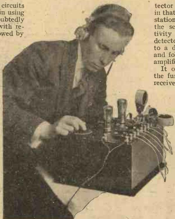
When the H.F. and Detector Circuit is in use, note that the two coils should be kept at right angles.
