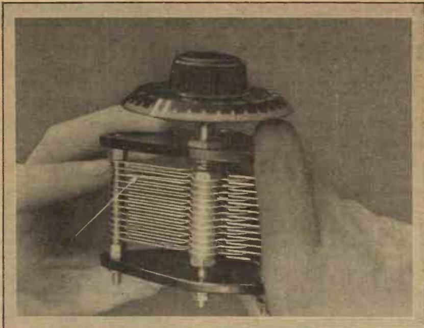
ones as it revolves. The easiest way to discover whether this is happening is to turn the moving plates to the maximum capacity position, and then hold up the condenser as shown in our third photograph with a sheet of white
