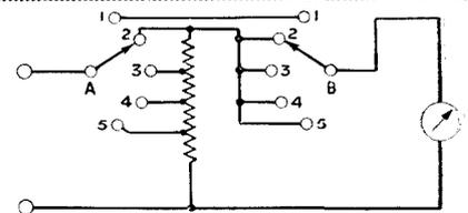
Fig. 3a. This is a more satisfactory means of switching shunts across a milliammeter.
