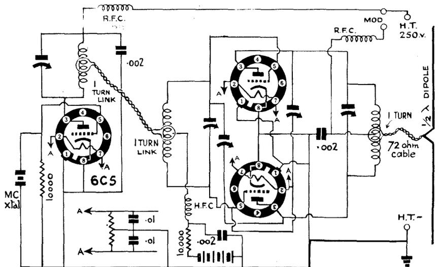
Here is the complete circuit for the transmitter. It consists of a triode crystal oscillator link coupled to two neutralised triodes in push-pull.
