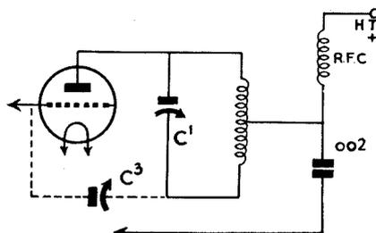
Fig. 1. Simplest radio frequency amplifier using a neutralised triode valve.
