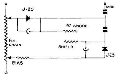
Fig. 2.—Double Modulation circuit employing metal rectifiers
