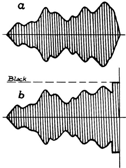
Fig. 1a.—A modulated carrier wave in which black corresponds to full amplitude.
