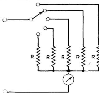
4a. A good method of constructing a multi-range voltmeter.
