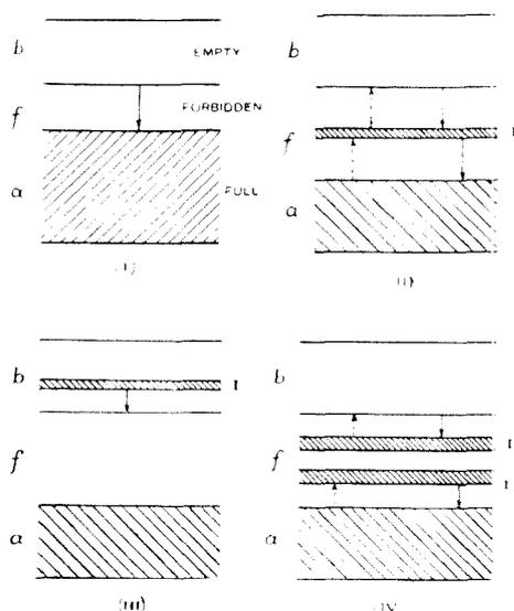
Fig. 2.—Electronic energy bands in fluorescent solids. The downward pointing arrows indicate transitions leading to fluorescence emission and the shaded bands marked  $I_1$ ,  $I_2$  and  $I_3$  are new levels introduced by impurities.
