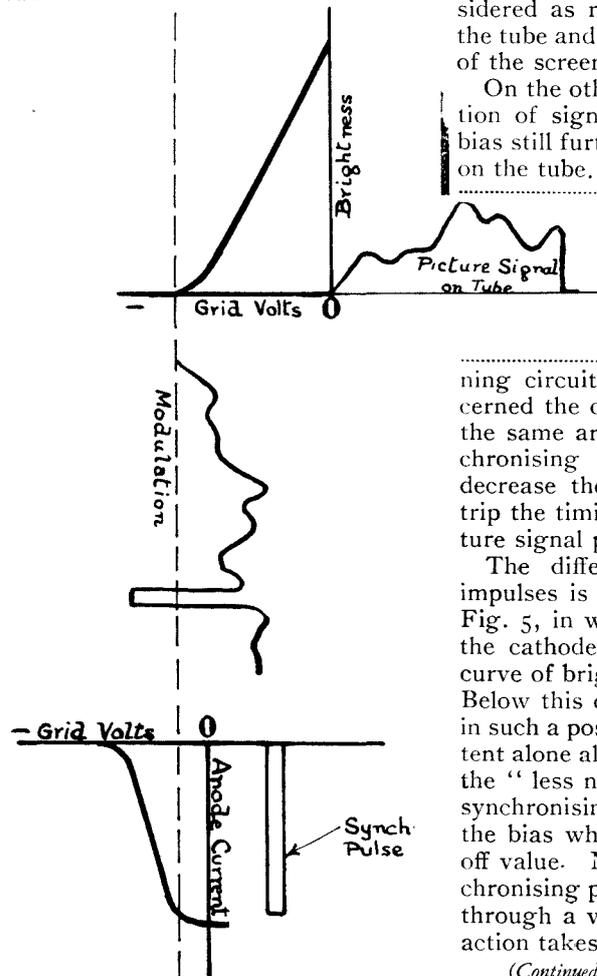
Fig. 5.—How the picture signal is separated from the synchronising pulse. At the top the signal is applied to the tube characteristic as shown, while the separating valve characteristic (bottom) only passes the synchronising pulse.
