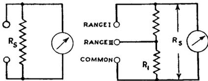
Fig. 1a. Extending the range of a milliammeter by a shunt. 1b. Another method of extending the range of a milliammeter.
