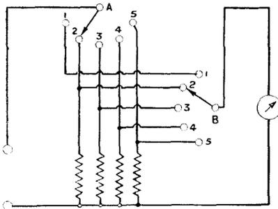
3b. Yet another efficient way of shunt switching.
