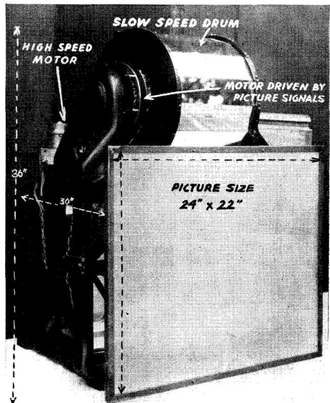
*A view of the chassis of the Scophony home receiver which can be contained in a cube approximately 30 inches square.*
