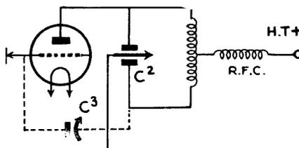
Fig. 2. A neutralised triode with split stator condenser omitting the fixed by-pass condenser.
