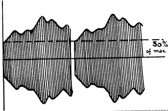
Fig. 4.—The present signal radiated by the B.B.C. in which the carrier drops to zero to provide the synchronising impulse.
