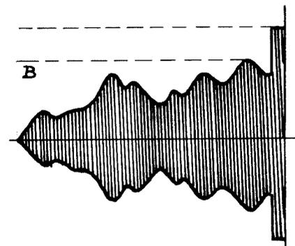
Fig. 3.—The method of distinguishing between signal and synchronising pulse used in the French system.
