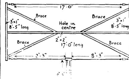
Fig. 6.—Rotary beam aerials only become practicable on 10 metres and under. Full dimensions of this aerial are given in this illustration.
