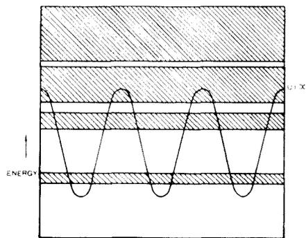
Fig. 1.—Possible energies (indicated by hatching) for an electron moving in a simple periodic field.
