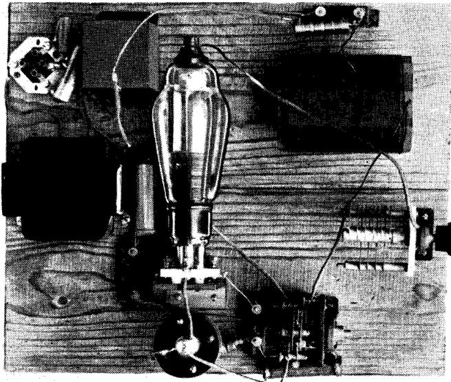
*If the valve is mounted in this way the bulk of the connecting leads are kept short. The valve socket in the top left corner is for the power supply.*
