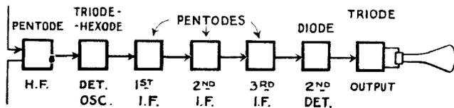
*Fig. 3.—Schematic diagram showing the stages in a vision receiver.*
