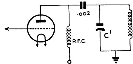
Fig. 5. This circuit prevents D.C. voltage being applied to the condenser, C1. The efficiency depends on the R.F. choke.
