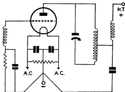
Fig. 6. To obtain smooth operation take all earth returns to a common point as shown.
