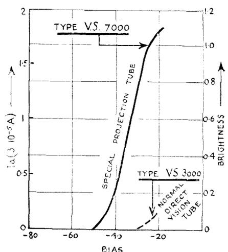
Fig. 3. Characteristics of projection tube.
