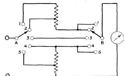
5. The switching arrangements in Figs. 3b and 4b can be used to form a combined voltmeter and milliammeter in this way.
