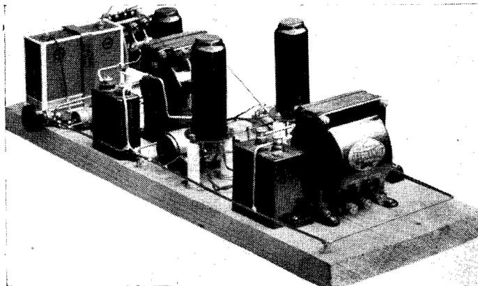
volts. This voltage is fed into the primary of a conventional transformer and is stepped up to 250 volts.
