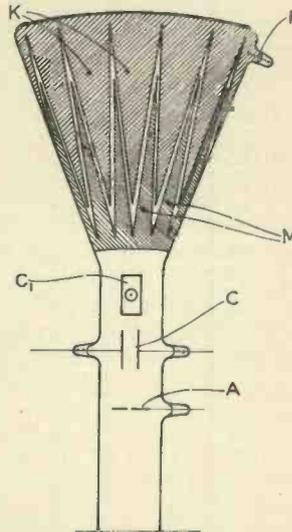
[Cathode-ray tube with serrated metallic coatings.]
