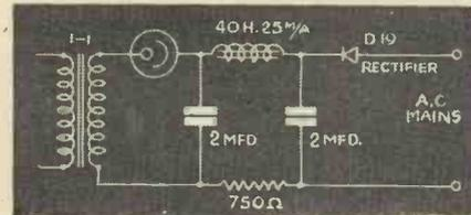
Fig. 5. Circuit of exciter unit for provision of extra H.T. from the mains.
