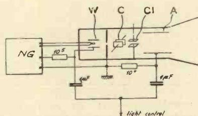
The Ardenne system of connections for cathode-ray tubes.
