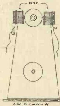
Fig. 3. This drawing shows an alternative and simpler method of fitting the gear directly.
