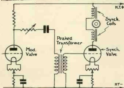
Fig. 1.—Circuit showing the usual synchronising arrangements employed with a mechanical receiver.
