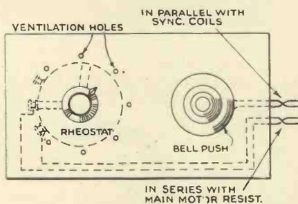
Fig. 2.—Details of a motor control panel.
