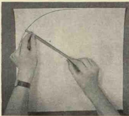
This photograph shows how the trammel is used to scribe the disc and the radial positions of the scanning holes.
