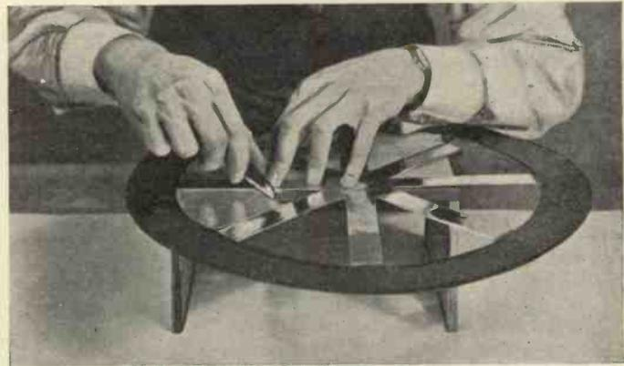
The spokes can be cut out with a sharp knife if the portion to be cut is rested along the edge of a piece of wood.
