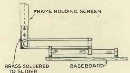
Fig. 3.—A cheap improvised focusing arrangement.
