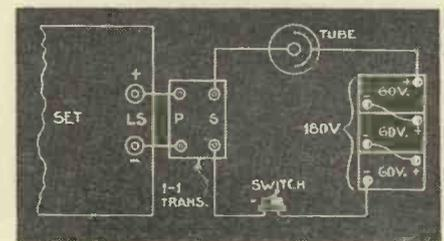
Fig. 3. A method of using a separate high-tension supply
