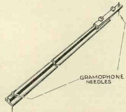
A sketch of the simple adjustable trammel used for marking out the disc.
