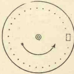
*This diagram shows the spiral arrangement of the holes in the disc.*
