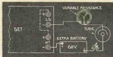
Fig. 2. A simple method of increasing the high-tension
