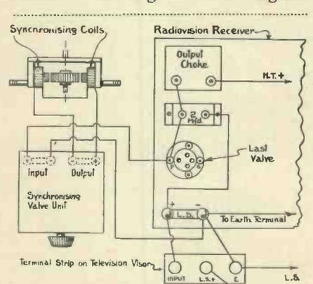
Fig. 5. The method of connecting the amplifier to the radio receiver.
