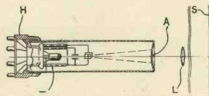
A novel construction of cathode-ray tube with an inwardly curved end.
