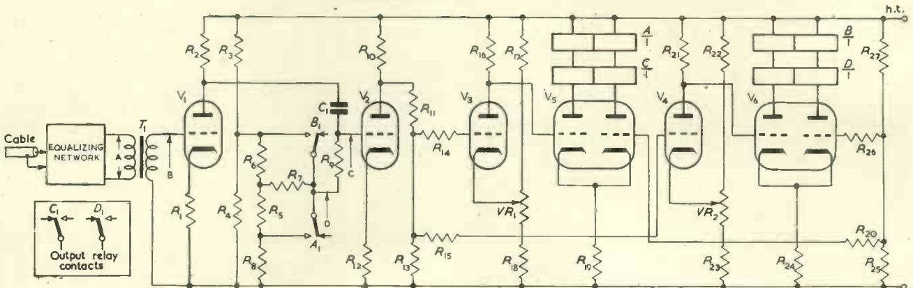
be amplified also. This interference, which is normally of very low frequency, is known as the "earth current," and undergoes daily cyclic variations. In the moving-coil system the signal bias caused by an earth current is automatically detected and corrected. The method by which this is done is fairly complicated, but the corrector is highly effective and is able to compensate for all but the very rapidly changing earth currents which sometimes occur during magnetic storms.
