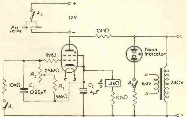
Fig. 6. Circuit used to provide automatic artificial respiration
