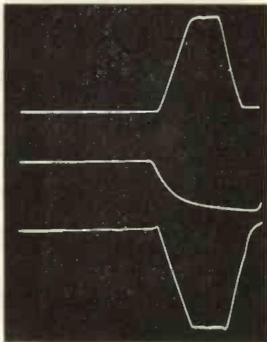
Fig. 10. 1.25  $\mu$ sec push-pull generator waveforms displayed on a 10  $\mu$ sec horizontal timebase
