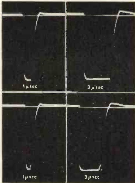
Fig. 3. Gating pulses of 1 and 3  $\mu$ sec duration
