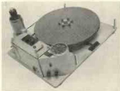
Velodyne and Ward-Leonard controls. The circuit is such that there is a high degree of stabilization against changes in supply voltage.
