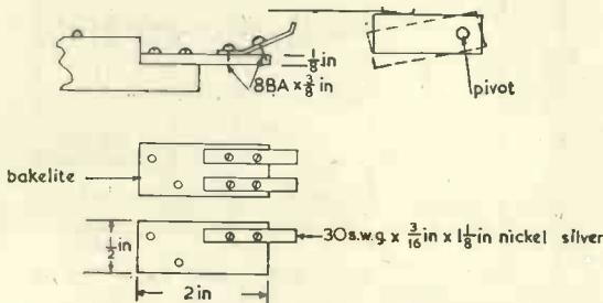
Fig. 14. Octave coupler key wipers and contact wires.
