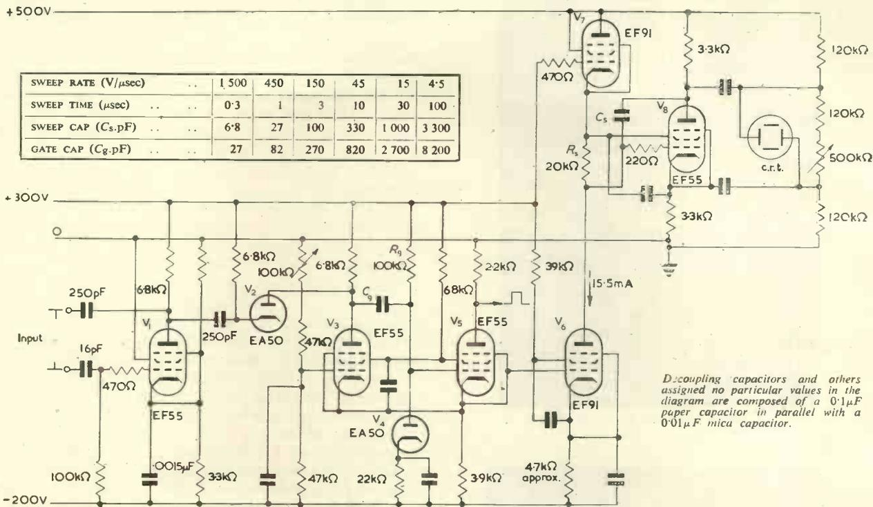
Fig. 6. Push-pull feedback sweep generator
