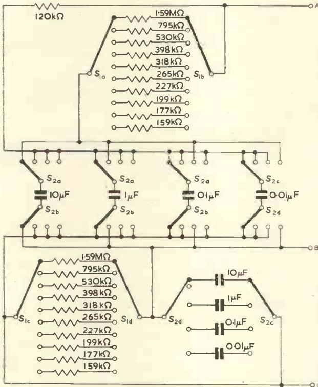
Fig. 5. Circuit of frequency control network
