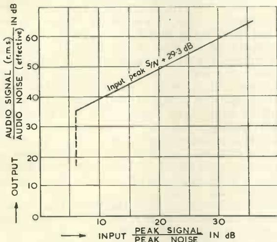
Fig. 2. Theoretical signal-to-noise ratio in p.l.m.
