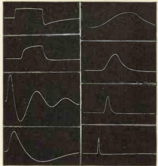
Fig. 11. Some blocking oscillator waveforms displayed on the push-pull generator sweeps
