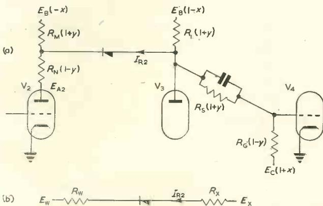
Fig. 11(a). Limits for checking lowest grid potential of a conducting valve
