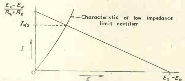
Fig. 12. Construction for determining  $I_{R2}$
