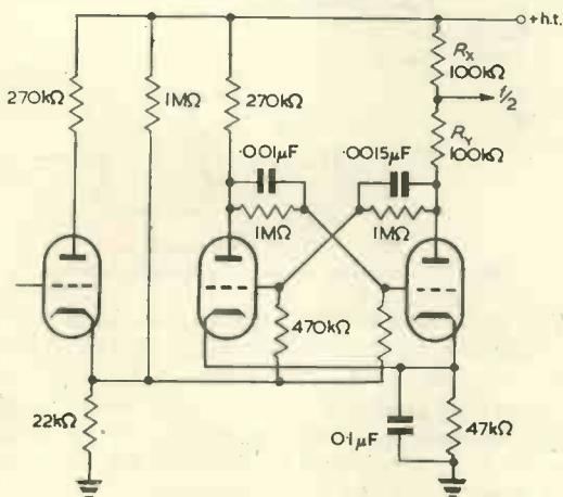
values of  $R_X$  and  $R_Y$  can be adjusted to set the level. The divided signals can be injected into the grid of the 6BA6 valve and another way of doing this is to tap the unison, 8ft and 16ft signals into a potential divider between the grid of this valve and earth, at points found by trial. These points are switched to isolate any particular pitch not required.
