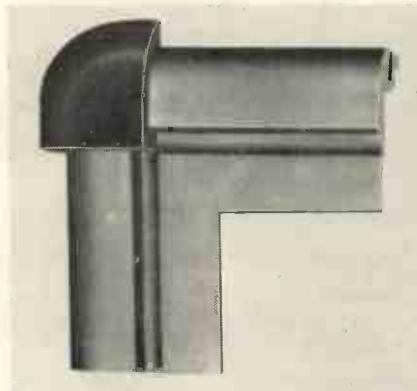
As will be seen from the illustration the triple-pronged corner-connector corresponds in section with that of the frame-member. Thus these two units interlock precisely and simply. Allowance is, of course, made for screw tapping or similar fixing: and the rebated edge on the frame-member provides for a clean flush fitting of panels of any suitable material.
