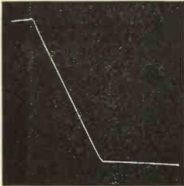
Fig. 9. 1.25  $\mu$ sec. 450V sweep, from push-pull generator, 1 000 sweeps superimposed
