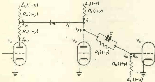
Fig. 9. Limits for determining  $R_M$  and  $R_N$
