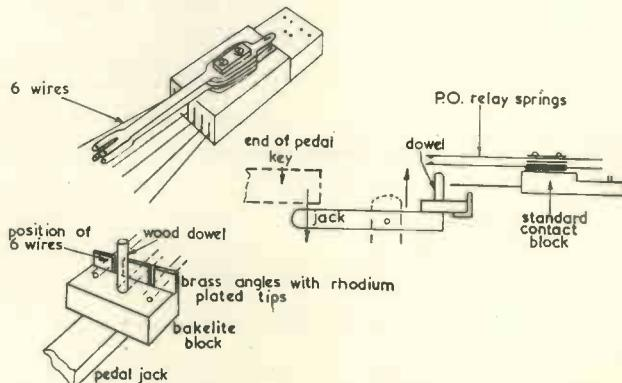
Fig. 21. Pedal generator, coupler and attack control contacts
