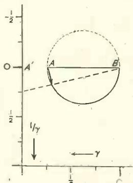
Fig. 5. Alternative scales for the locus of  $1/(1+j\gamma)$
