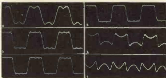
Fig. 8. (a) Synthesis of square wave: Fundamental+3rd harmonic; (b) Fundamental+3rd and 5th harmonics; (c) Fundamental+3rd, 5th and 7th harmonics; (d) Fundamental+3rd, 5th, 7th and 9th harmonics; (e) As (d) but with fundamental amplitude reduced; (f) As (d) but with fundamental suppressed.
