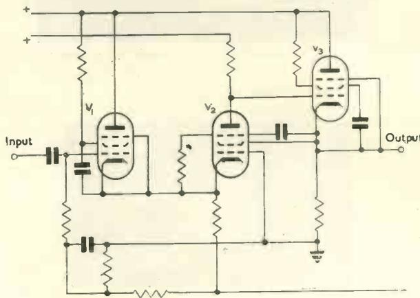
impedance for the input signal, while  $V_2$  provides a cathode-follower output capable of driving the screen and suppressor grids of  $V_1$  to follow the rise of its anode voltage, in order to allow the latter to rise at the maximum possible rate once the valve has been cut off by the rising edge of the input waveform.
