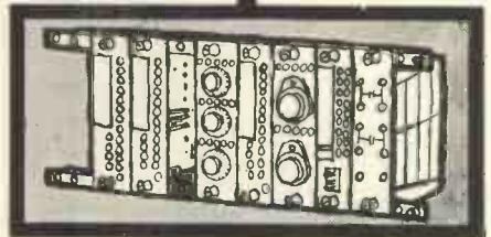
(Inset above). A problem board assembled externally to the computer, ready for patching.
