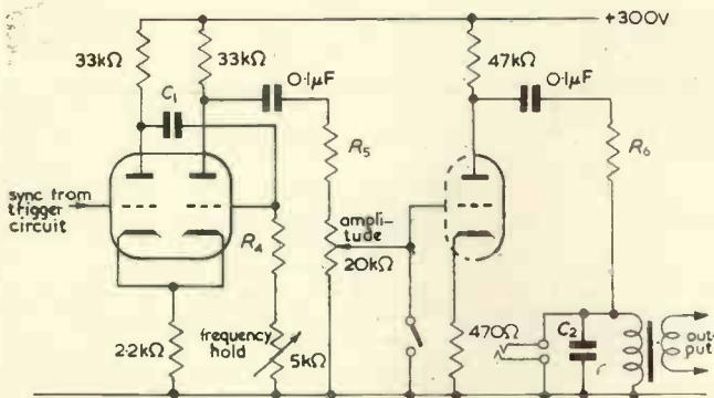
Fig. 4. Harmonic multivibrator and output stage
