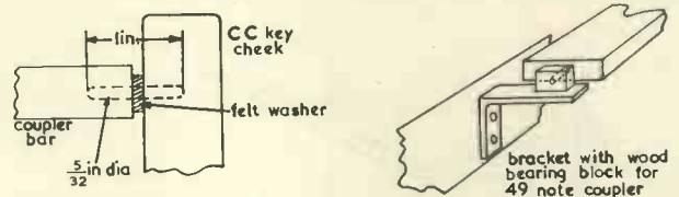
Fig. 15. Coupler bar mounting details
