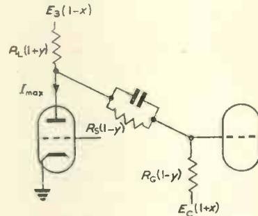
Fig. 7. Limits for determining  $E_{A3}$
