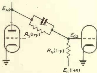
Fig. 8. Limits for determining  $E_{G_2}$
