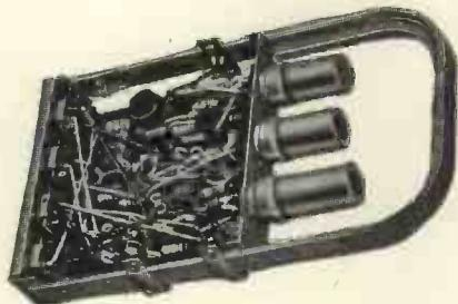
'Duralumin' is used in the construction of the 223 plug-in units which form the main feature of the 402 computer.
