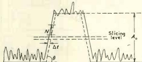
Fig. 1. Time shift of the pulse edges due to noise voltage
