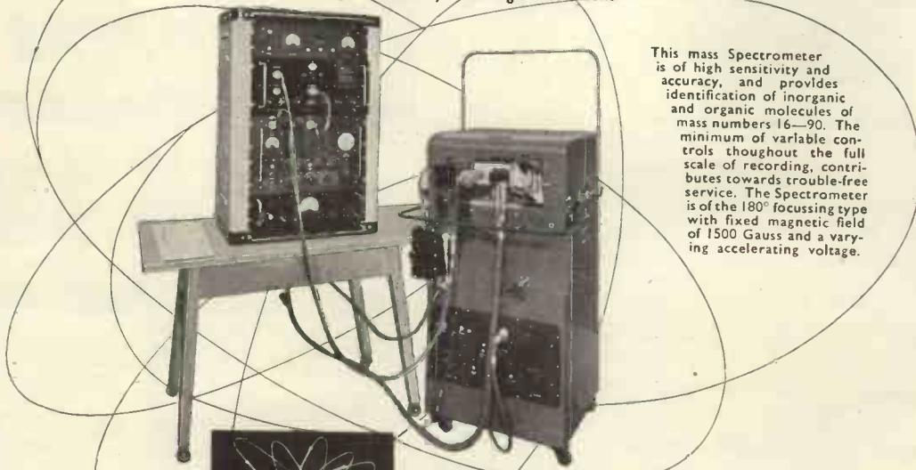
This mass Spectrometer is of high sensitivity and accuracy, and provides identification of inorganic and organic molecules of mass numbers 16—90. The minimum of variable controls throughout the full scale of recording, contributes towards trouble-free service. The Spectrometer is of the 180° focussing type with fixed magnetic field of 1500 Gauss and a varying accelerating voltage.
