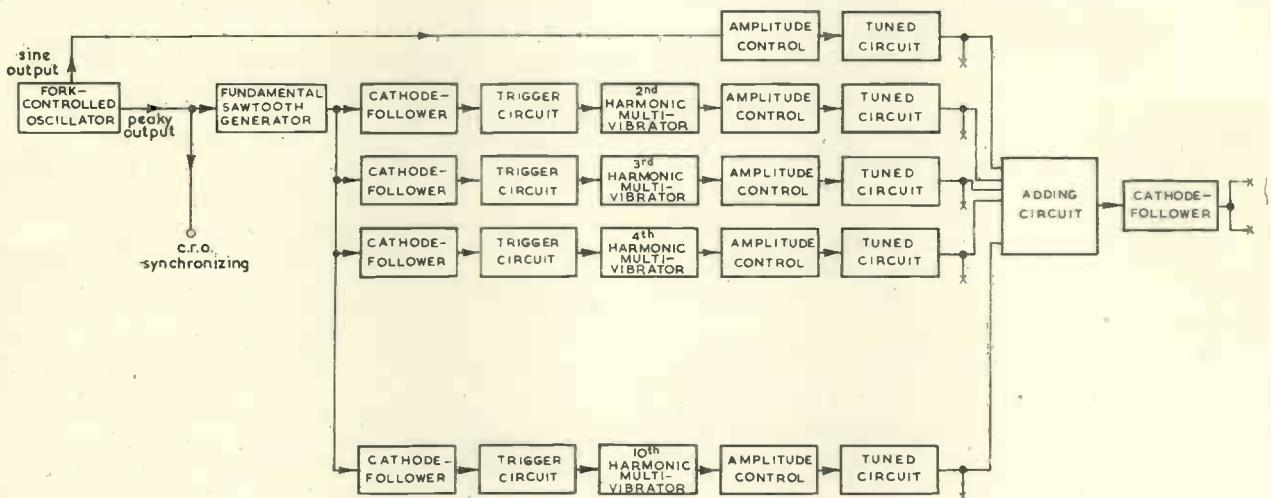
Fig. 1. Arrangement of the synthesizer
