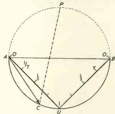
Fig. 6. The use of the minus-unity point as a pole for the frequency and period scales
