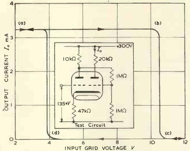
Fig. 3. Measured transfer characteristic of Schmitt-Trigger circuit
