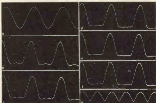
Fig. 7. (a) Fundamental; (b) Fundamental+2nd; (c) Fundamental+2nd+4th; (d) Fundamental+2nd+4th+6th; (e) Fundamental+2nd+4th+6th+8th; (f) Fundamental+2nd+4th+6th+8th+10th; (g) Half-wave rectified sine-wave with fundamental suppressed
