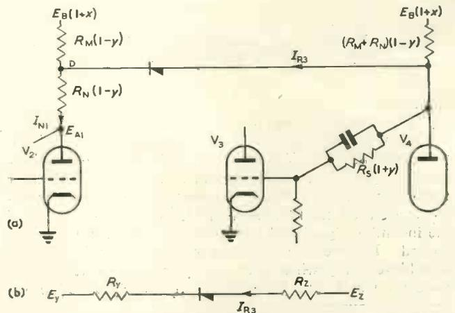
Fig. 13(a). Limits for checking minimum effective anode load resistance
