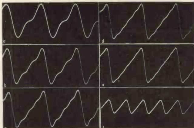
Fig. 9. (a) Fundamental+2nd; (b) Fundamental+2nd+3rd; (c) Fundamental+2nd+3rd+4th; (d) Fundamental+2nd+3rd+4th+5th; (e) Fundamental+harmonics up to 6th; (f) Fundamental and odd harmonics suppressed from sawtooth
