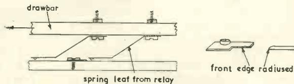
Fig. 23. Alternative arrangement using sliding contacts
