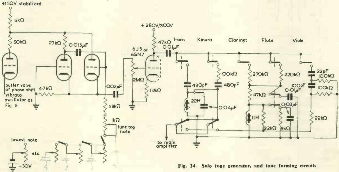
Fig. 24. Solo tone generator, and tone forming circuits
