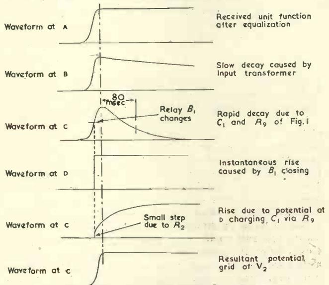
Fig. 2. Waveforms in circuit when unit function is received
