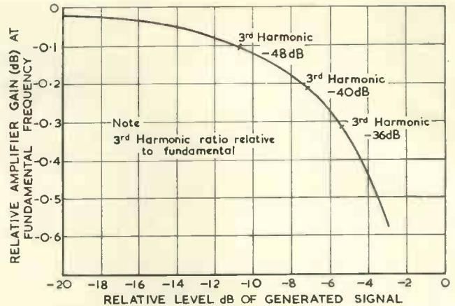
Fig. 6. Measured relationship between amplifier gain at the fundamental frequency and the amplitude of the generated signal
