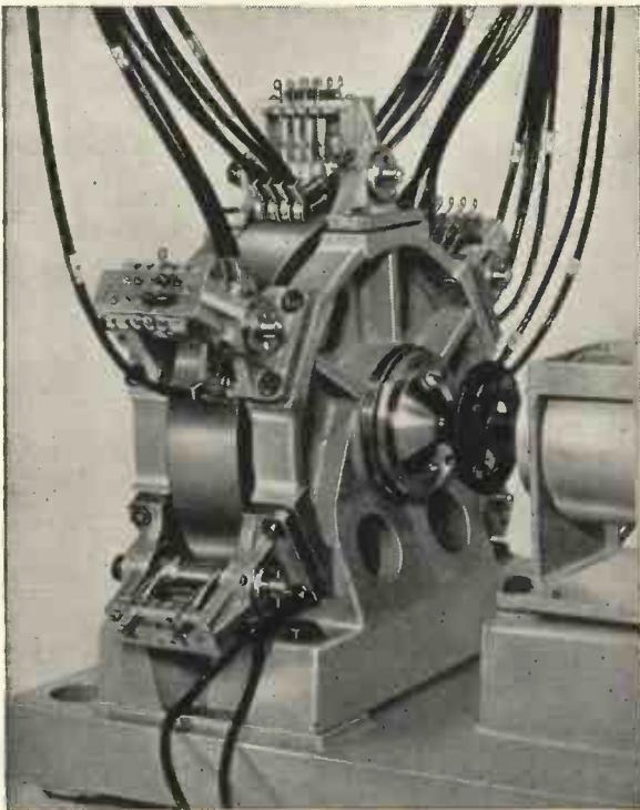
For the drum, which is the main store or memory of the computer, a metal was required with sufficient homogeneity for symmetrical turning to obviate the need for balancing and which would thereafter remain stable. 'Duralumin' was the answer.
