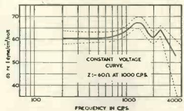
The latest Miniature Earphone is characterised by its high efficiency and slim, elegant appearance. The curve shown above was taken on a Post Office type 1½ c.c. artificial ear and the dotted lines represent the 95% confidence limits calculated from a batch of Earphones of this type.
