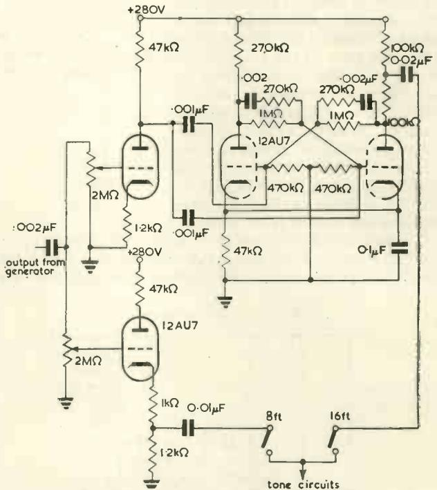
Fig. 25. Frequency divider and isolating valves
