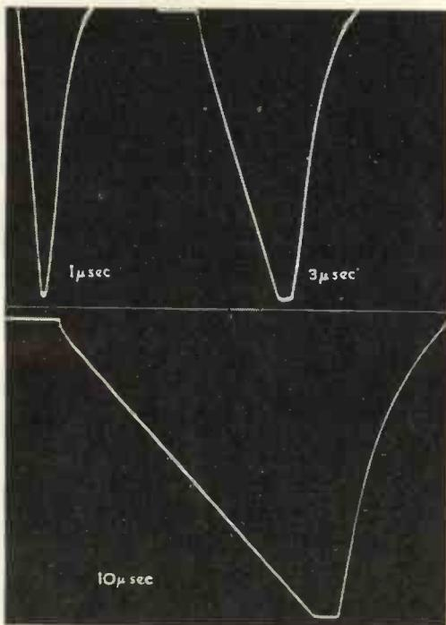
Fig. 4. Sweep waveforms from single ended sweep generator of 1, 3, and 10  $\mu$ sec duration
