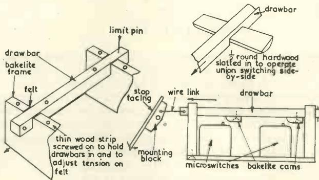
Fig. 22. Stop switches using microswitches
