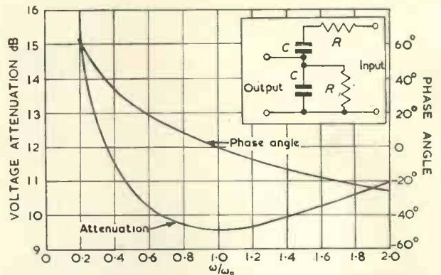
Fig. 1. Attenuation and phase angle/frequency characteristic of basic frequency control network at a given setting  $\omega_0 = 1/CR$
