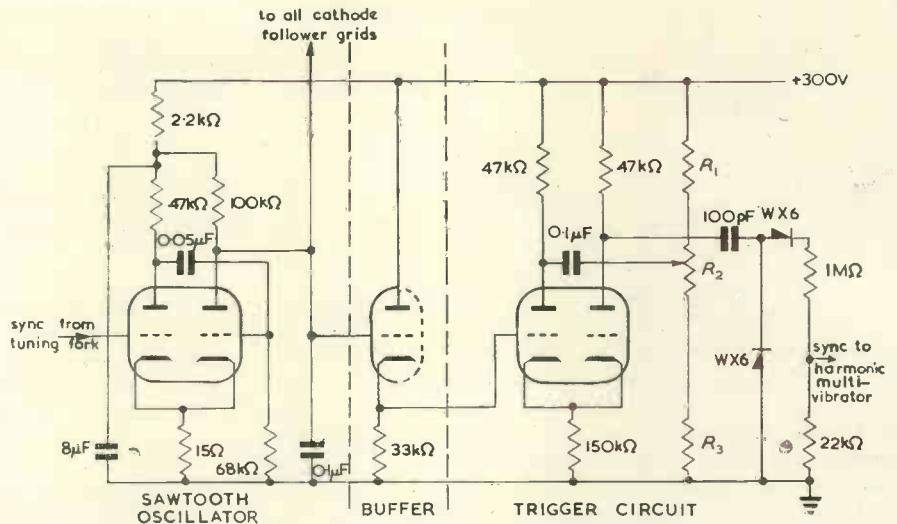
Fig. 3. Phase controlling unit
