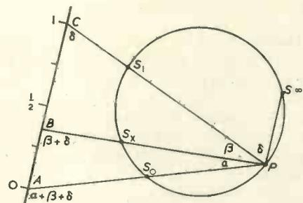
Fig. 7. Illustrating general relationship between pole and scale
