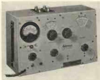
directly in terms of circuit magnification. The oscillator is modulated at 50c/s 50 per cent, so that d.c. amplifiers need not be used in the valve voltmeter, thus eliminating zero setting.
