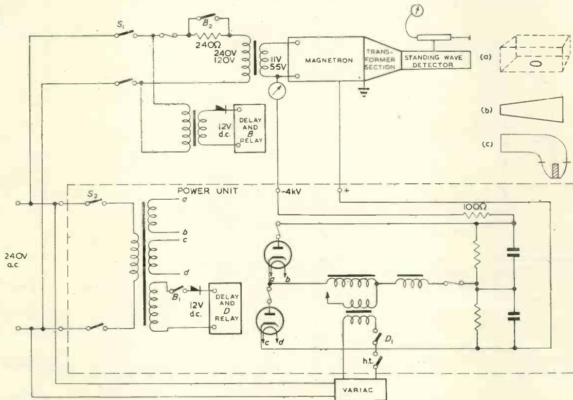
Fig. 2. General Layout of Apparatus
