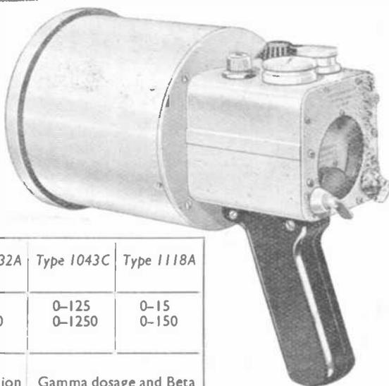
This Monitor is designed for use with X-Rays and will give accurate indication of dosage of soft radiation. It is self-contained and portable. There are other Ekco Monitors of similar design for Gamma dosage and Beta qualitative detection, as listed on right.
