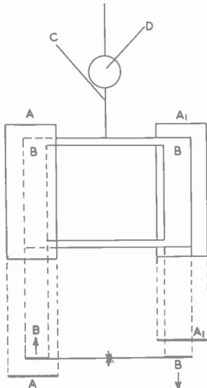
Fig. 18. Mechanical arrangement of a Knudsen gauge
