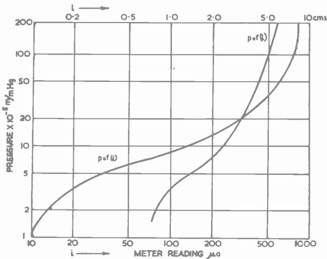
Fig. 16. Calibration curve for Philips ionization gauge
