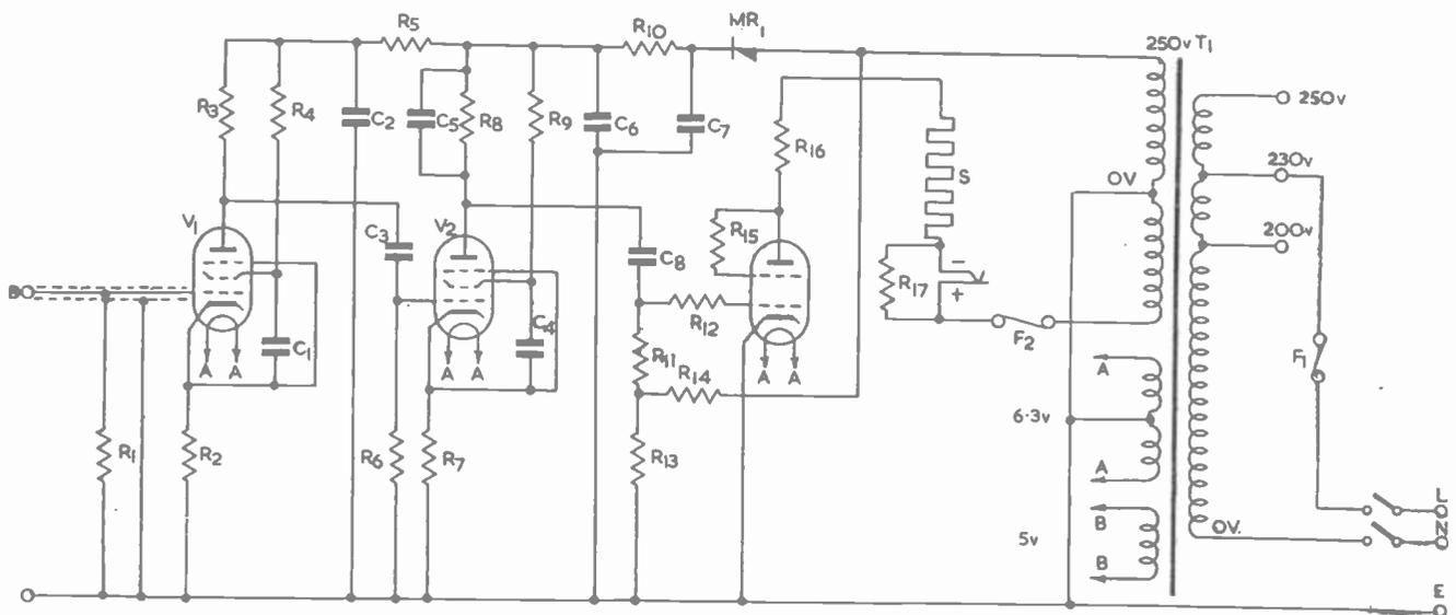
$R_1 = 1 \text{ M}\Omega$ ,  $R_2 = 2.2 \text{ k}\Omega$ ,  $R_3 = 220 \text{ k}\Omega$ ,  $R_4 = 1 \text{ M}\Omega$ ,
