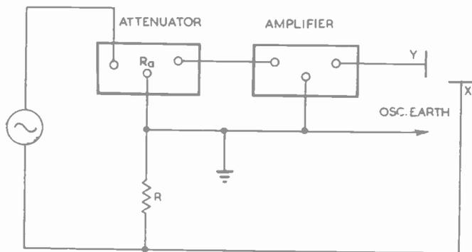
Fig. 1. Usual circuit to measure voltage gain
