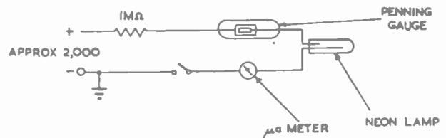
Fig. 15. Philips gauge with indicator
