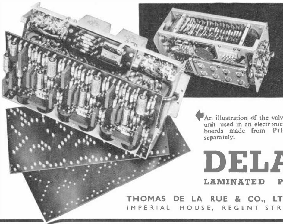
← An illustration of part of the navigational equipment of an aircraft, showing Delaron insulation mounting strips and terminal panels wired in position.
