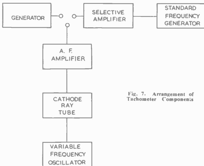
Fig. 7. Arrangement of Tachometer Components
