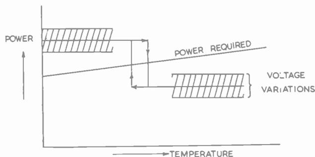
Fig. 1. Operation of two-position controller
