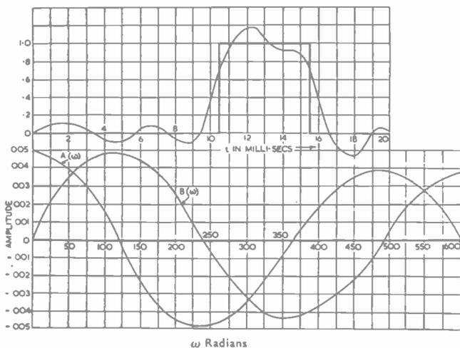
Fig. 3. Fourier analysis and re-synthesis of a short pulse
