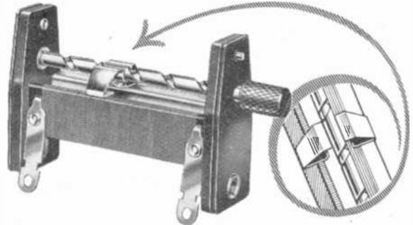
The value of the EGEN midget pre-set variable resistor to the television and electronics designer has been enhanced by a new *double slider* operating on the radius of the element, giving greater stability and making accurate adjustment easier. This reliable, precision engineered component can also be supplied mounted in a series of one, two or three on a common panel which can be suitably engraved. Available in any value from 10 ohms. to 25,000 ohms.
