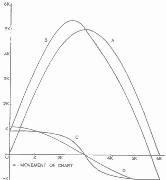
Fig. 6. A is part of a sine curve drawn by a pen with friction
