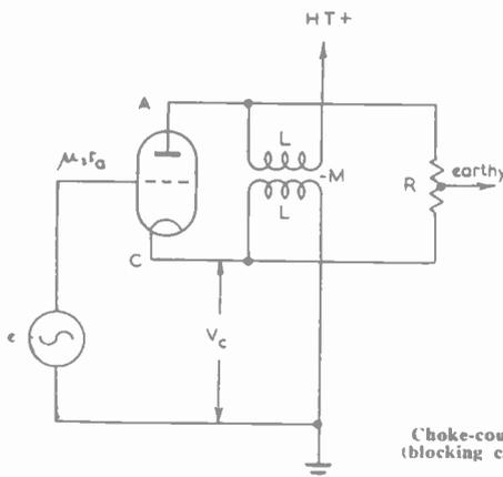
Fig. 1. Choke-coupled phase invertor (blocking capacitors not shown)
