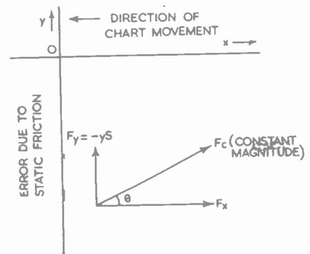
Fig. 1. Diagram of the forces exerted on the pen by its supports
