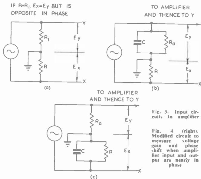
Fig. 3. Input circuits to amplifier
