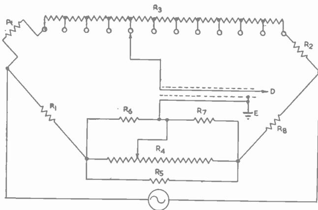
$R_1 = 24 \Omega$ ,  $R_2 = 32 \Omega$ ,  $R_3 = 11 \times 1 \Omega$ ,  $R_4 = 10 \Omega$ ,
