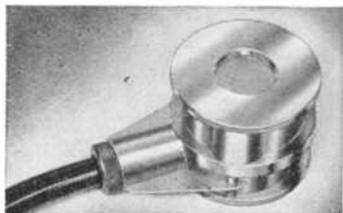
*Transducer Head. The generating crystal is air-backed to give maximum ultrasonic output. Special rear connections to crystal eliminate corona discharge at high R.F. potentials. Siastic rubber sealing rings can be supplied, enabling the transducer to be immersed in liquids up to 150°C. temperature.*
