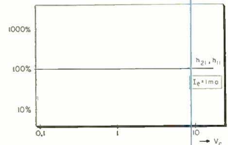
Fig. 7: Parameter  $h_{11}$  and  $h_{21}$  variation with  $V_c$ .
