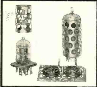
"Ventilator" shields not only improve "hot" tube performance by dissipating heat but are the most economical shields in Methode's extensive line. Easily handled and compression fitted to ground terminals on Methode laminated or printed circuit sockets, shields are available in lengths of 1-11/16" or 2-1/16" with one standard diameter which fits either seven or nine pin tubes. Available with tin or black oxide finish.
