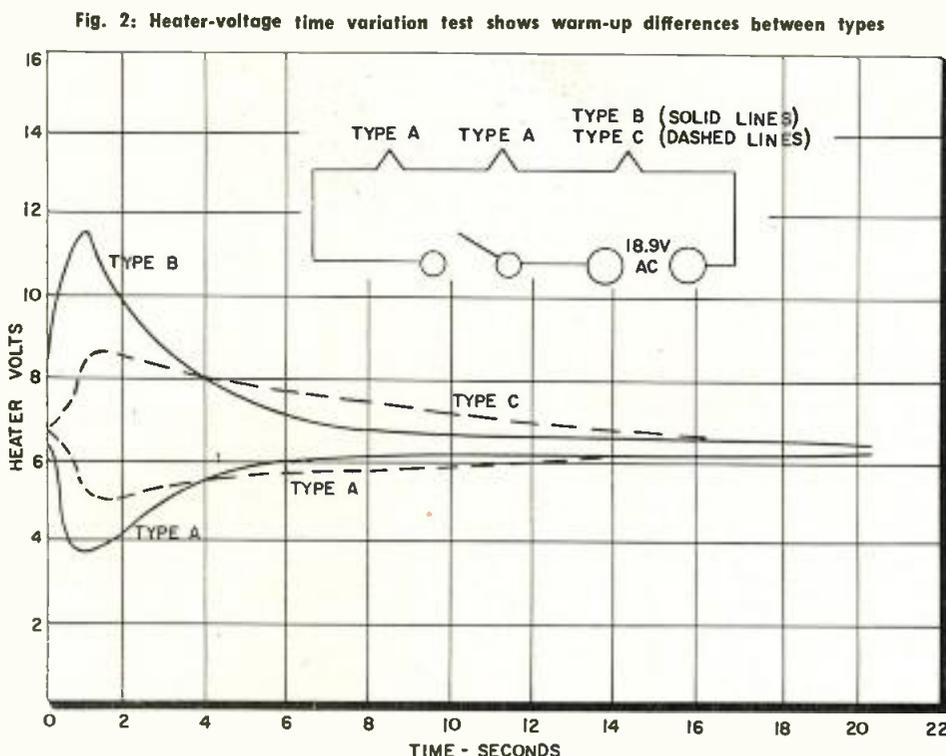
Fig. 2: Heater-voltage time variation test shows warm-up differences between types
