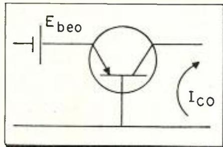
Fig. 11: Transistor equivalent circuit
