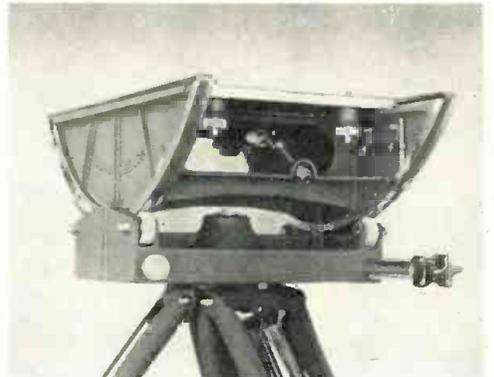
**COLOR CRADLE HEAD.** Specifically designed for RCA color television cameras. Action is similar to monochrome cradle head. On both models, camera, with all accessories attached, can be balanced perfectly when mounted on the head simply by moving the top plate on the head forward or back with a lead screw. Adapted to fit all recommended tripods, pedestals or dollies
