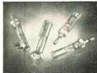
**MIDGET TRIMMER CAPACITORS** are available in standard types from 0.5 to 12.0 mmfds., or they can be designed to your requirements. Temperature coefficient for brass core units is approx. 200 ppm/deg. C.; for invar core units, approx. 50 ppm/deg. C.
