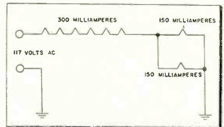
Fig. 6: Circuit designs using series-parallel combination illustrated are not reliable.
