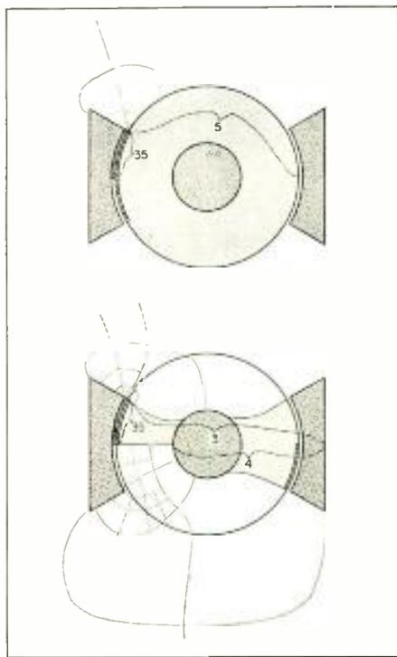
Fig. 5: Field-plotting for 2-wire line
