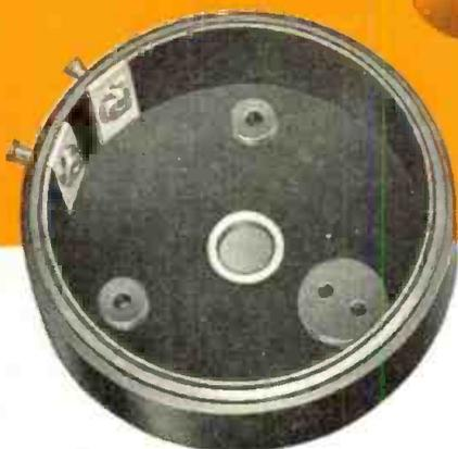
**Good Linearity at Moderate Cost** Resistance wire is uniformly wound and finished card is cemented tightly into base — uniform thickness around base prevents unequal curing and aging out of round — every unit produced is inspected for conformance with linearity specifications.
