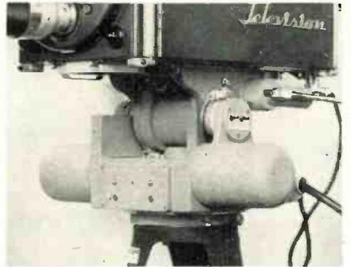
**REMOTE CONTROL HEAD.** Makes possible the operation of a TV camera from a remote point several hundred feet away. Panning, tilting, focusing and lens changing are accomplished with small electric motors operated from a portable control panel. Operation is smooth and steady. Speed is variable. Camera can be mounted in extremely high or low positions on stage, in auditoriums, stadiums, on rooftops and other inaccessible places.
