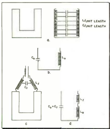
Fig. 4: 2-wire line and equivalent circuits
