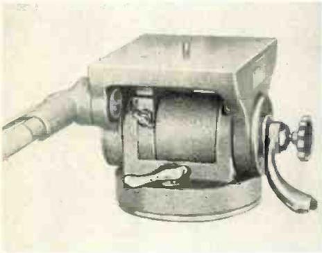
**FRICTION HEAD.** The most practical head for monochrome TV cameras and motion picture cameras weighing between 80 and 150 lbs. Provides smooth, easy panning and tilting. Pans full 360°. Tilts 45° up and 45° down. Adjustable drag and brakes provided on both actions. Camera is accurately counterbalanced. Adjustable to compensate for extra lenses, etc.
