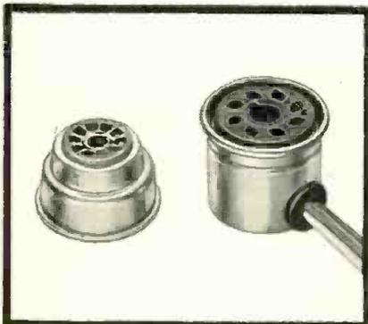
Newly designed laminated tube sockets for dip solder attachment to printed wiring panels supplements Methode's earlier development of molded snap in printed circuit sockets. Individual terminal hole punching permits printing of jumper and cross over connections directly on circuit panel. Springlike tabs permit amazingly strong terminal dip solder connections.
