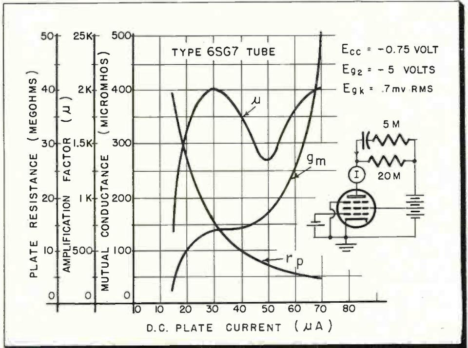
Fig. 2: Variations in tube parameters as a function of 6SG7 tube plate current
