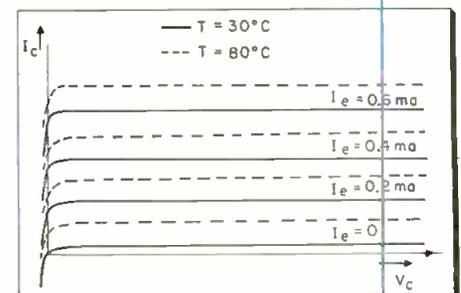
Fig. 9: Temperature-output characteristics
