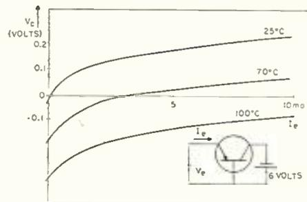
Fig. 10: Input-temperature characteristics
