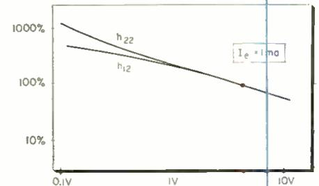
Fig. 6: Parameter  $h_{12}$  and  $h_{22}$  variation with  $V_c$ .
