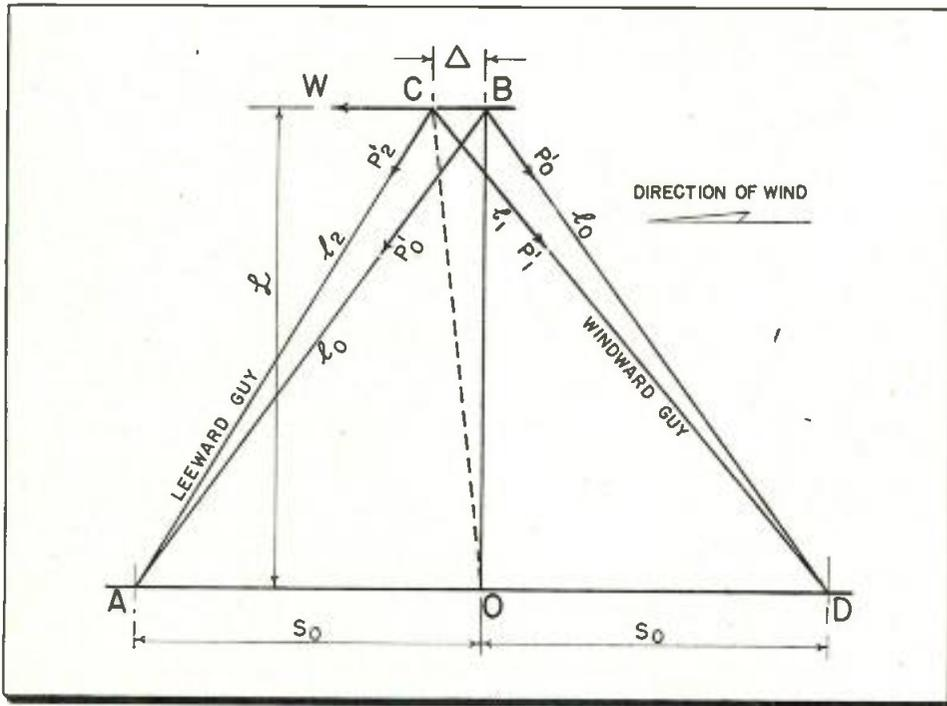
Fig. 3: Analyzing the case of 2 guys lying in a plane parallel to the wind direction
