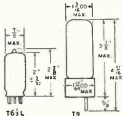
Amperite Regulators are the simplest, most effective method for obtaining *automatic regulation* of current or voltage. *Hermetically sealed*, they are not affected by changes in altitude, ambient temperature ( $-55^{\circ}$  to  $+90^{\circ}$  C), or humidity. Rugged; no moving parts; changed as easily as a radio tube.
