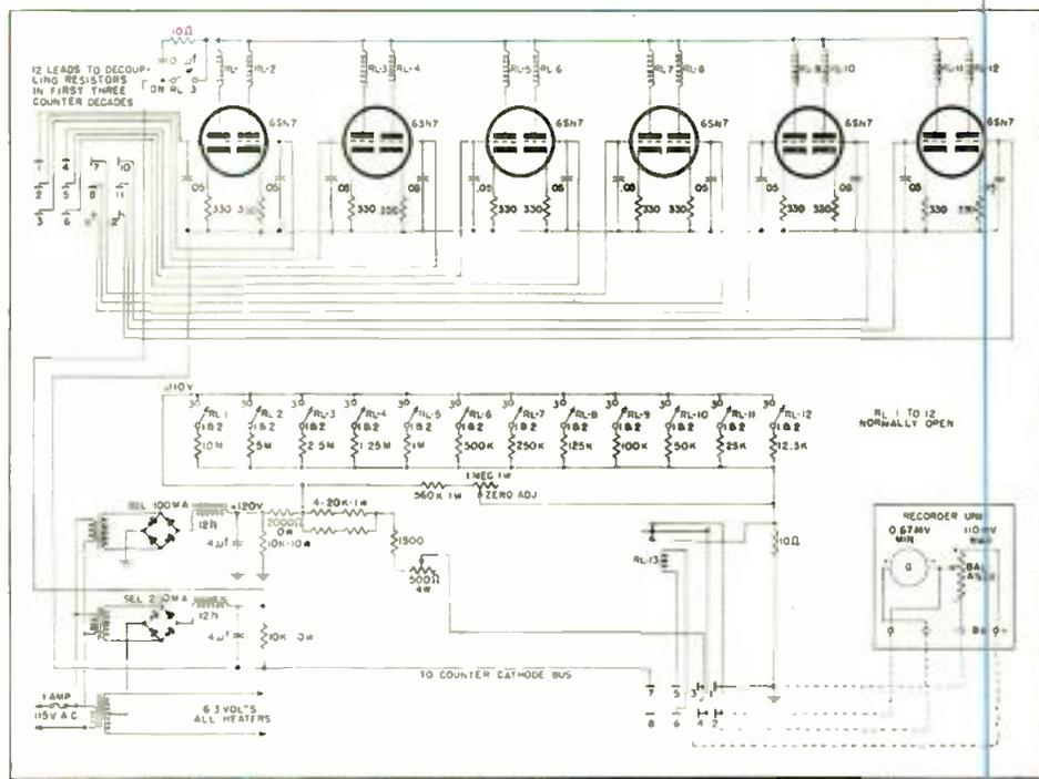
Fig. 5: Output voltage of this generator is proportional to numerical value indicated by lights
