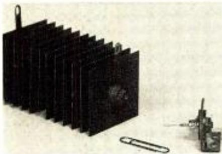
New silicon power rectifier at right operates over  $-60^{\circ}$  to  $150^{\circ}$  C. Selenium unit is at left
