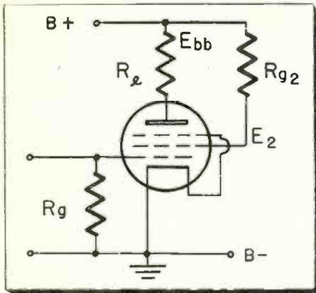
Fig. 1: Basic starved amplifier circuit
