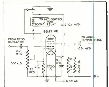
Conelrad warning employs avc controlled relay
