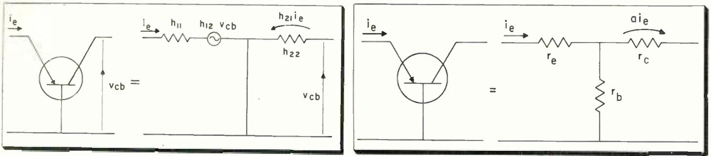
Fig. 1: (l) Low frequency equivalent transistor circuit, h-type Fig. 2: (r) Equivalent transistor circuit, T-type
