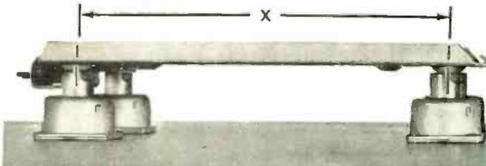
Excessive height required. Unit mount bulk imposes reduced spacing (X) between support centers, resulting in impaired stability (critical in lateral direction). Greater sway space required.
