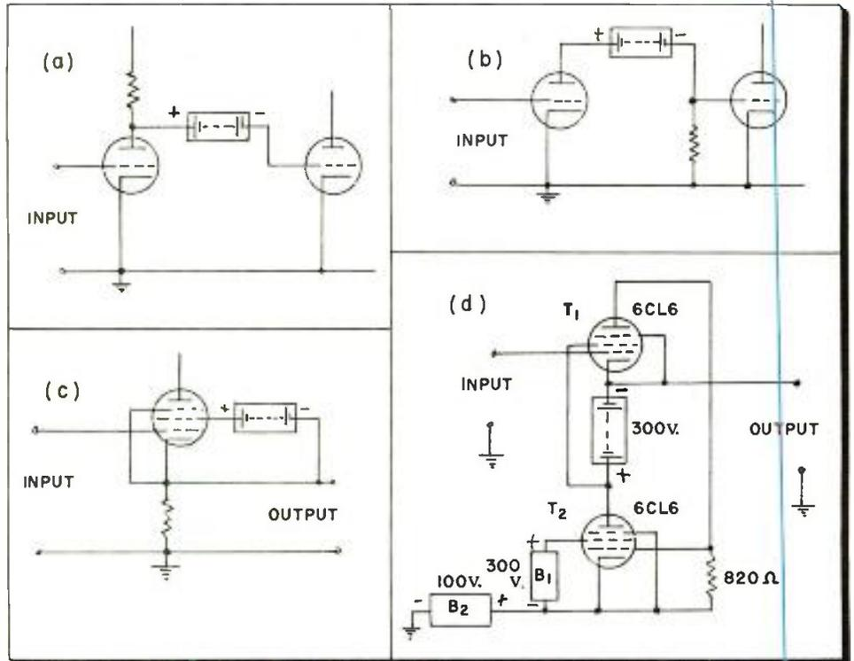
(a and b) Power supply in interstage coupling. (c) Use in pentode cathode-follower circuit with low input capacitance. (d) Special application in two-tube direct-coupled cathode-follower circuit
