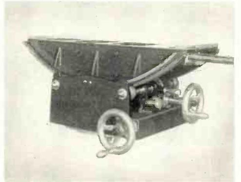
**GEARED HEAD.** Provides exceptionally smooth, constant-speed panning and tilting for television and 35mm motion picture cameras. Two geared speeds on both the pan and tilt. Gearing can be quickly disengaged so unit operates as a free head. In tilting, the head rotates camera about its center of gravity, maintaining absolute balance at all times. Full 360° panning is smooth and steady.
