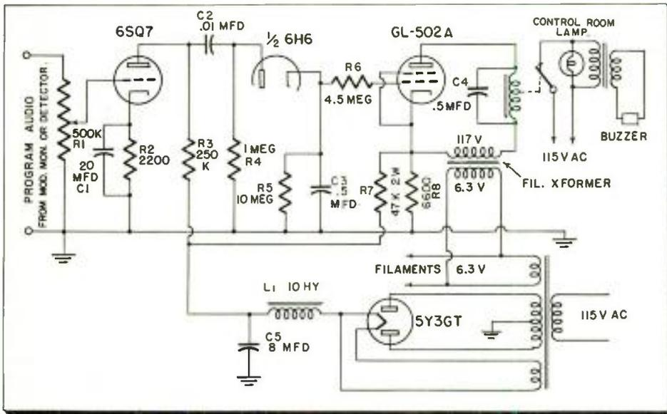
Circuit of program carrier alarm actuated by carrier modulation to sound buzzer or flash alarm
