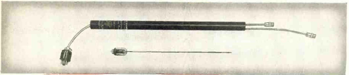
**Type 6493**—Low level 2000-4000 MC amplifier. Greater than 35 db gain with 15 MW output.
