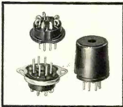
For high voltage tubes these corona caps and socket combinations for both octal and noval sizes feature generously rolled outer surfaces. Assemblies are designed for screw mounting to condenser studs or stand offs and are available with general purpose black or low loss mica phenolic insulators. Noval caps available with 1-5/16" or 1-1/2" major rim diameter. Octal units have insulating fibre liners.
