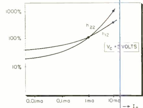
Fig. 8: Parameter  $h_{12}$  and  $h_{22}$  variation with  $I_e$ .
