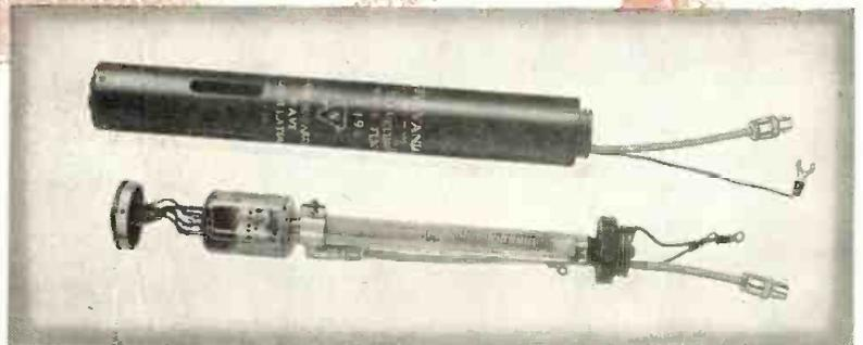
**Type 6496**—Tunable backward wave oscillator. 35 MW output, up to 1 watt. Complete 2000-4000 MC coverage.
