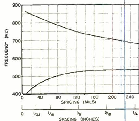
Fig. 6: Frequency vs. spacing, with 416 A tube
