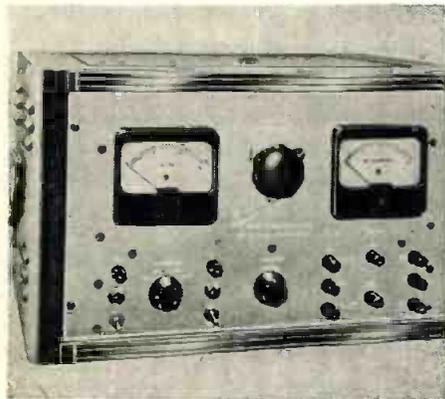
5 ma. The unit offers a fixed voltage of 250 v., 0 to 50 ma, derived from the C supply, and an unregulated 6.3 v., 10 amp, center-tapped, filament supply. It will provide klystrons with up to -600 v. cathode voltage, and an additional 0 to -250 v. for the reflector. Furnished to operate from either 115 or 230 v. ac, 50/60 cps single phase. Polytechnic Research & Development Co., Inc., 202 Tillary St., Brooklyn 1, N.Y.—TELE-TECH & ELECTRONIC INDUSTRIES. (Ask for 1-22)
