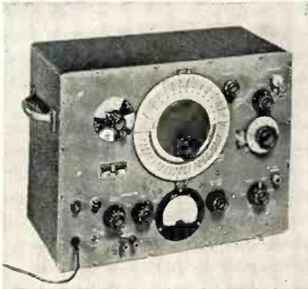
measurements can be obtained. Circuitry consists of an r-f oscillator, modulating amplifier, VTVM, attenuator, 400 cps oscillator, and power supply. The r-f carrier may be modulated from the internal oscillator or from an external source. Minimum leakage and stray fields, high reading accuracy of the frequency dial, low cable standing wave errors. Light weight, sturdy construction. Clough-Brengle Co., Dept. TT, 6014 Broadway, Chicago 40, Ill.—TELE-TECH & ELECTRONIC INDUSTRIES. (Ask for 1-23)
