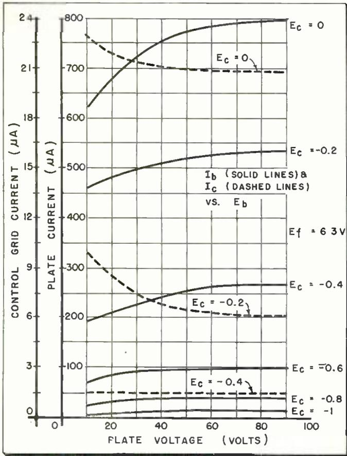
Fig. 6: (above) Static characteristics of 6AG5, screen voltage 10 v.
