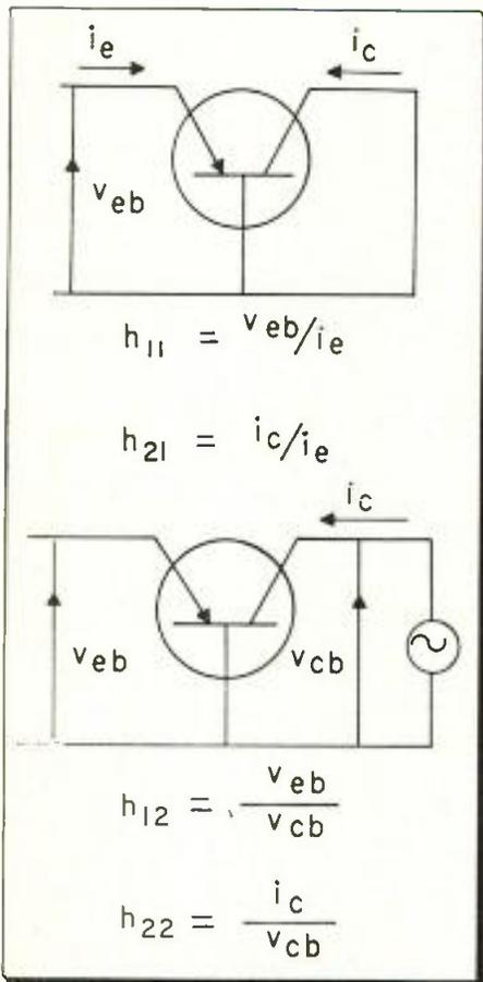
Fig. 3: Measurement of h-parameters
