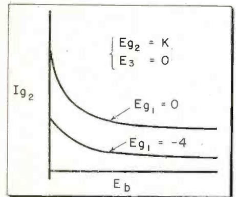
Fig. 8: Space current—plate voltage curves
