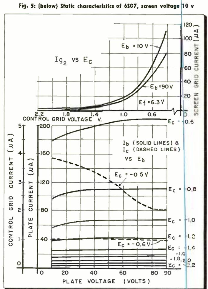
Fig. 5: (below) Static characteristics of 6SG7, screen voltage 10 v
