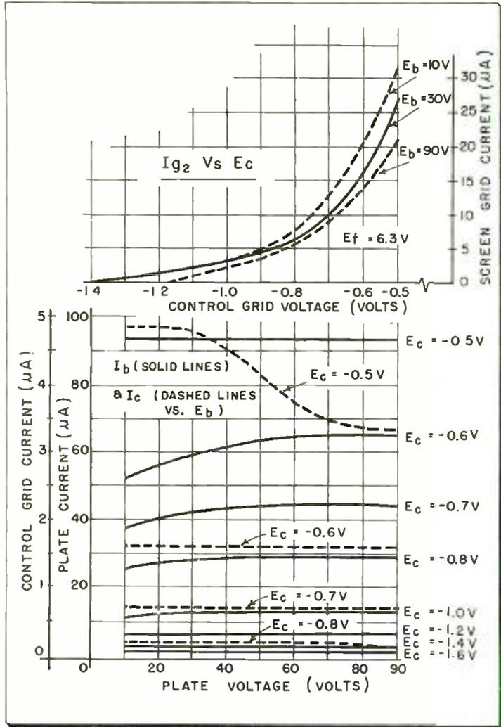
Fig. 4: (I) Static characteristics of 6SG7 with screen voltage 5 v.
