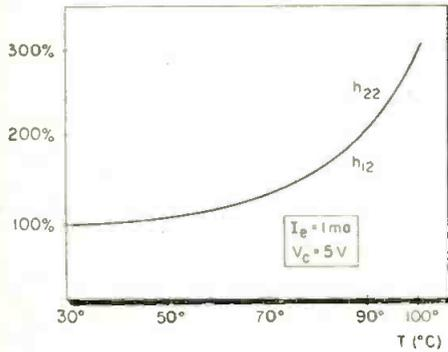
Fig. 12: Increase of  $h_{22}$  with temperature
