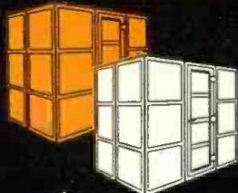
An economical enclosure, available in copper or galvanized wire cloth, that meets basic requirements for suppressing r-f radiations of industrial or laboratory equipment. Copper Screen: 70db from 100kc to 1000mc, 40db at 14kc. Galvanized Screen: 40db from 15kc to 400mc (Uniform-Field measurements).
