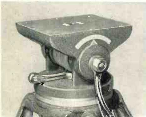
**TILT HEAD.** For fixed-position TV cameras or microwave parabolas. Friction-type action, but without drag adjustment. Camera or parabola may easily be positioned and locked in place. Calibration scales on both azimuth and tilt allow for quick re-setting of fixed points.
