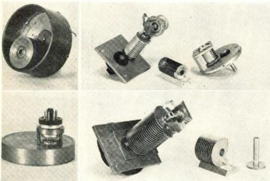
Fig. 1: (l) Eccentric concentric line oscillator. Fig. 2: (r) Examples of two-wire type construction
