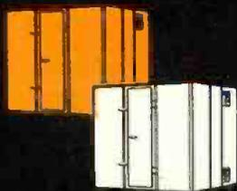
These enclosures employ the rugged Lindsay Structure, available in either sheet copper or galvanized. They can be transported completely assembled or disassembled; may be used indoors or out. Copper: 100db from 150kc to 1000mc; 70db at 15kc (Uniform-Field measurements). Galvanized: 110db from 14kc to 1000mc; 9db at 60cps; 37db at 1000cps for magnetic fields (MIL-S-4957 measurements).
