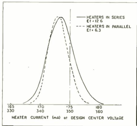
Fig. 3: Comparison of series and parallel heater currents at design center voltage
