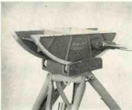
**MONOCHROME CRADLE HEAD.** Remarkable smoothness and ease of operation for black and white TV cameras are made possible by the perfect balance of the monochrome cradle head. The camera rotates around a constant center of gravity, always in absolute balance. Tilts down 38° and up 30° on ball bearing rollers. Tilt drag is adjustable. In panning, also rides on ball bearings. Brakes on both pan and tilt
