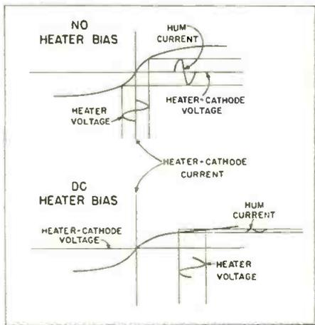
Fig. 5: Heater bias voltage reduces hum
