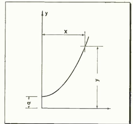
Fig. 1: Catenary formed by suspended cable
