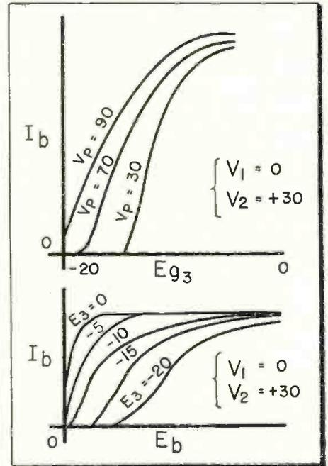
Fig. 9: Effect of change in plate resistance
