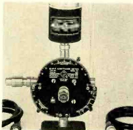
necessary. Furthermore, accuracy has been improved by several additional calibrated points on the multiplying-factor scale. And, at low frequencies, a small, shielded, variable air capacitor replaces the adjustable stub previously used as a susceptance standard. The unit is direct reading from 41 to 1,500 MC. General Radio Co., 275 Massachusetts Ave., Cambridge 39, Mass.—TELE-TECH & ELECTRONIC INDUSTRIES.
