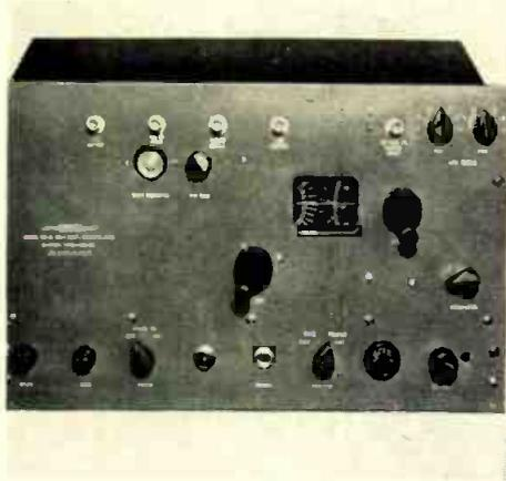
of frequency in the range of 20 to 1,000 MC with an accuracy of better than 1 part in  $10^7$ —depending on the accuracy of the 100 kc source. The unit can be operated directly from a 105-130 v., 60 cps, ac line, and its safety factor allows continuous operation for indefinite periods. Gertsch Products, Inc., 11846-48 Mississippi Ave., Los Angeles 25, Calif.—TELE-TECH & ELECTRONIC INDUSTRIES.
