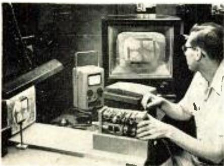
An inspector in Camden, N. J., plant of RCA Victor Div., Radio Corporation of America, checks circuits of the company's new "TV Eye" closed-circuit television camera as initial models come off assembly lines. Midget 4-lb. camera, with housing removed from chassis, is focused on test pattern at left. Signal, channeled through control unit seen between camera and receiver, reproduces pattern on receiver screen.
