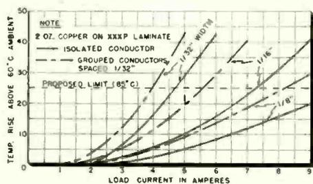
Fig. 9: Temperature rise of etched conductors
