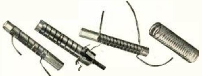
Corning Metallized Glass Inductances—are noted for their exceptionally high electrical stability and negligible drift characteristics, even under widely variable ambient temperatures. High Q is inherent. They can be furnished with uniform, variable or double-pitch windings and for fixed tuned, permeability tuned inductance trimmer combinations.
