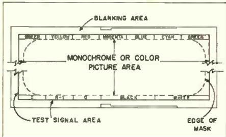
addition, a color burst and possibly one line of gray scale would be sent. These signals are described as consistent with approved standards, would generally lie in masked-off area, and would provide standard of comparison for receivers whenever needed.
