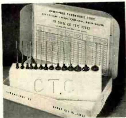
$\frac{1}{8}$  in. wide and vary to approximately  $\frac{1}{2}$  in. in diameter. All units are varnish-impregnated for moisture and fungus-proofing. Inductances are RMA preferred values ranging from 6.8  $\mu$ h to 1.0 mh. Color-coding is the RMA three-dot system. An inside cover chart gives all necessary electrical data. Cambridge Thermionic Corp., 445 Concord Ave., Cambridge 38, Mass.—TELE-TECH & ELECTRONIC INDUSTRIES.
