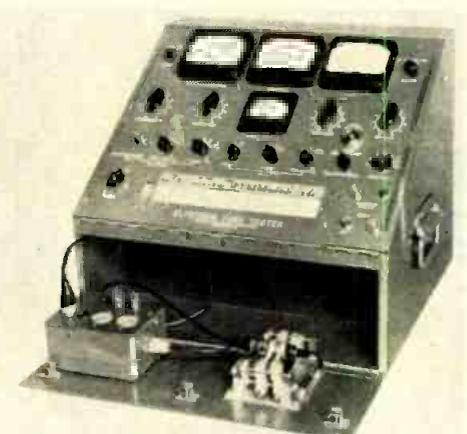
ments, precautionary means for safely testing high voltages, and convenient tube data charts for the rapid determination of control settings. It also provides for external modulation so that the klystron tubes may be tested dynamically with external r-f measuring equipment. Polarad Electronics Corp., 100 Metropolitan Ave., Brooklyn 11, N.Y.—TELE-TECH & ELECTRONIC INDUSTRIES.
