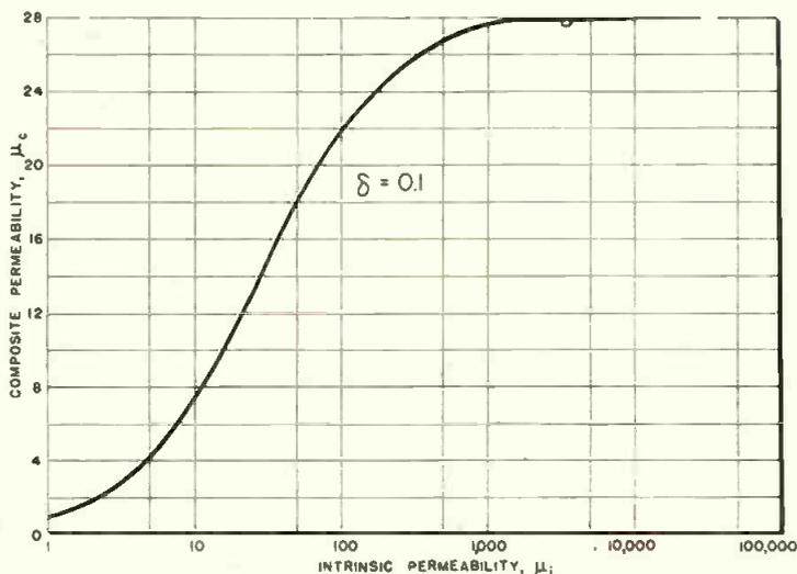
WHEN powdered iron is placed in the magnetic field of an r-f coil, both the inductance and resistance of the coil increase. The Q of the coil may either increase or decrease depending on the relative changes of inductance and resistance. We are only concerned in this paper with the increase of inductance.
