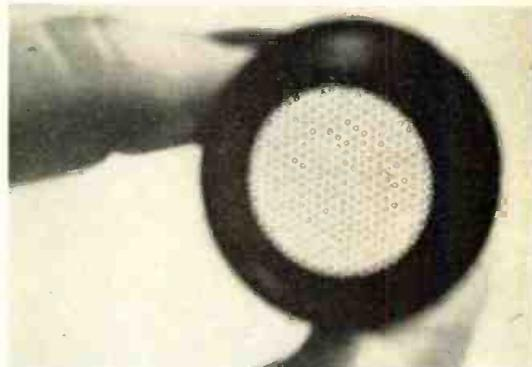
**6** Color-dot pattern as seen through magnifying lens. The 600,000 dots are arranged in triangular groups, each group containing RGB
