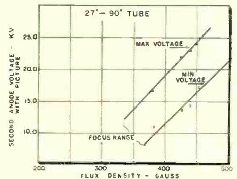
Fig. 3: Focus range available with unit positioned 1 3/32 in. from edge of G<sub>1</sub> anode
