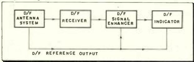
Fig. 2: Delay line enhancer delays and adds desired signal
