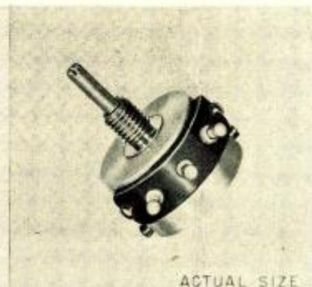
separated by "Paliney" contact material. The take-off brushes are made of gold alloy and rotate on a coin-silver ring. The metals provide noise-free operation for a life of one million cps. The unit is available with up to  $360^\circ$  electrical and mechanical rotation in resistance ranges up to 50,000 ohms,  $\pm 1.0\%$ . Jet Electronics, Inc., 93 Massachusetts Ave., Boston, Mass.—TELE-TECH & ELECTRONIC INDUSTRIES.
