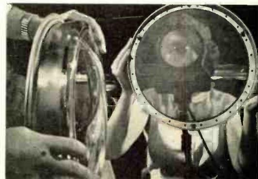
**3** Quality control inspection of shadow mask (r) assures that specifications are met. Tube's 15-in. faceplate (l) is also checked
