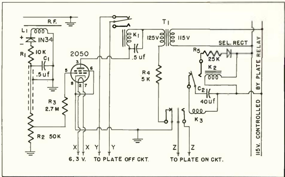
Rapid cycling lightning protection obtained from self operating thyratron relay
