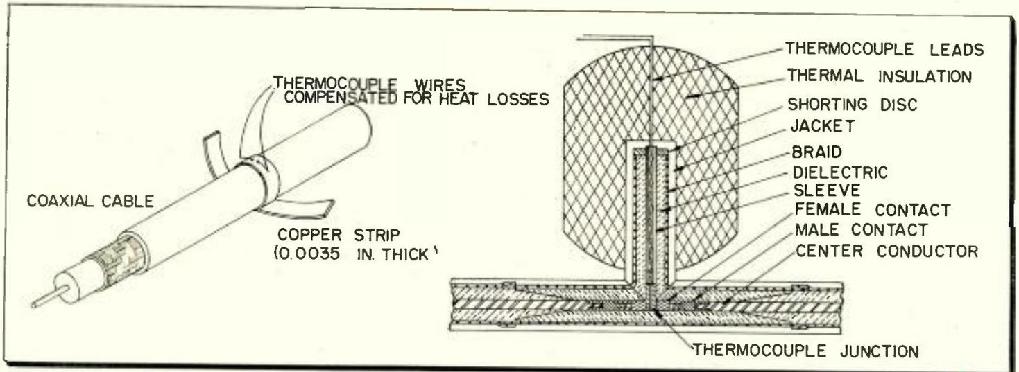
Fig. 2: (a) Cable surface temperature measured with thermocouple on copper strip. (b) Transformer isolates thermocouple from center conductor
