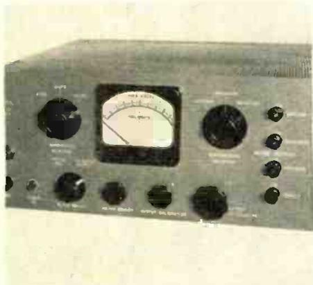
The basic noise source is a gas tube producing an approximate Gaussian output. This provides the signal source to the three controlled distribution channels generating the Gaussian, Rayleigh, and uniform distributions. The distributions are accurate to 2%. Statistical Instrument Co., P.O. Box 552, Church St. Sta., New York 8, N.Y.—TELE-TECH & ELECTRONIC INDUSTRIES.
