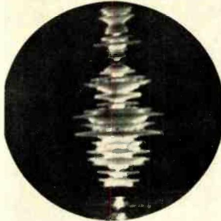
Capt. Richard Dobbin of the "Flying Cloud" operates first commercial U. S. installation of "Fischlupe" (top), made by Electroacoustic G.m. b.H., Germany, and distributed by Radiomarine Corp. of America. Supersonic signals reflected from fish are displayed on CRT (bottom) showing large school of fish located above sea bottom
