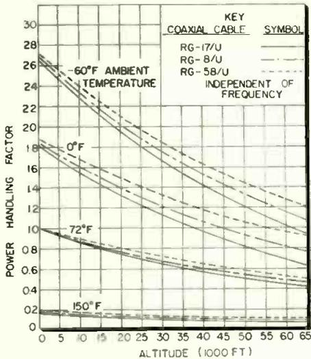
Fig. 9: Theoretical power rating factors for various coaxial cables at various altitudes with environment temperature as parameter
