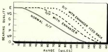
Fig. 9: Graph showing results of flight tests with and without the signal integrator
