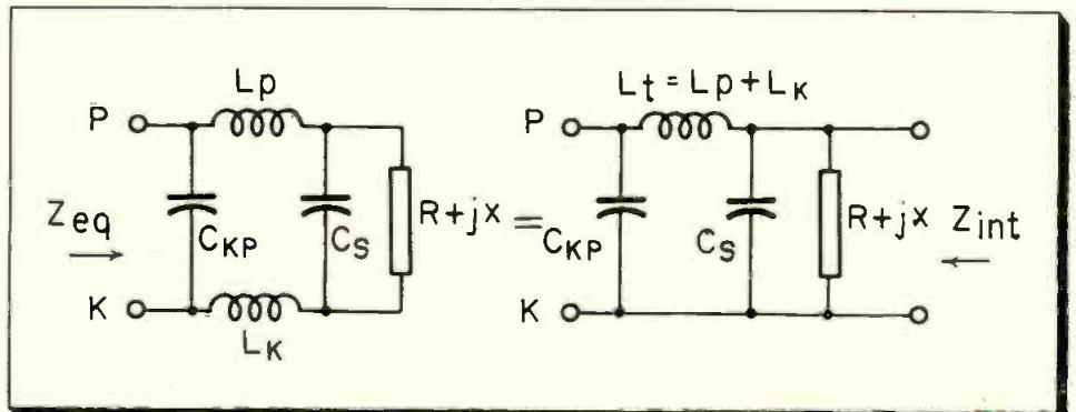
Fig. 1: Four-terminal network connected to diode results in desired current in external load
