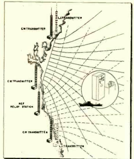
Fig. 1: Type N Raydist employs transmitters on shore, and receiving and phase-measuring equipment on craft exploring for oil in Gulf
