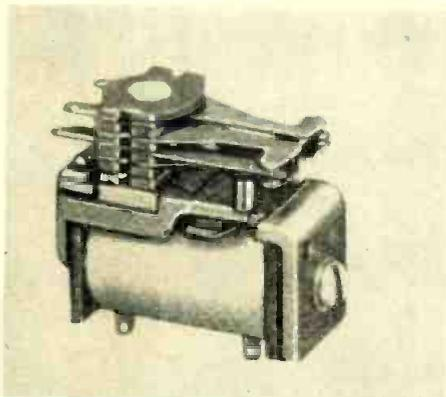
government specifications. Coil windings are rated for dc voltages up to 115 v. Contacts are palladium and rated non-inductive load at 3 amps. at 24 v. dc, or 115 v., 60 cps. Units can be supplied with silver contacts rated at 5 amps. on special order. Smallest of the series, in the hermetically sealed types, type 8614, measures  $1\frac{5}{8} \times 1\frac{1}{2} \times 1\frac{21}{32}$  in. Signal Engineering & Manufacturing Co., Long Branch, N. J.—TELE-TECH & ELECTRONIC INDUSTRIES.
