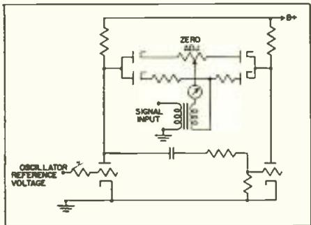
Fig. 3: Schematic of phase sensitive detector
