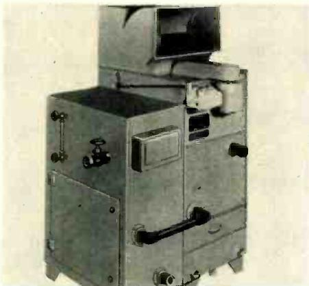
supply cooling water as low as 86° F with a 75° wet bulb condition. Capacity range is from 36,000 BTU/hr. to 465,000 BTU/hr. with entering water temperatures from 90° F to 160° F. Volume of cooling water from 20 G.P.M. to 150 G.P.M. Mayer Refrigerating Engineers, Inc., Lincoln Park, N.J.—TELE-TECH & ELECTRONIC INDUSTRIES.
