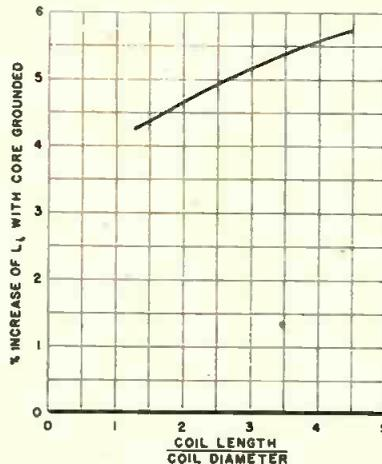
Fig. 7: (l) Coil's apparent inductance when core is grounded. Fig. 8: (r) Curves for high ratios
