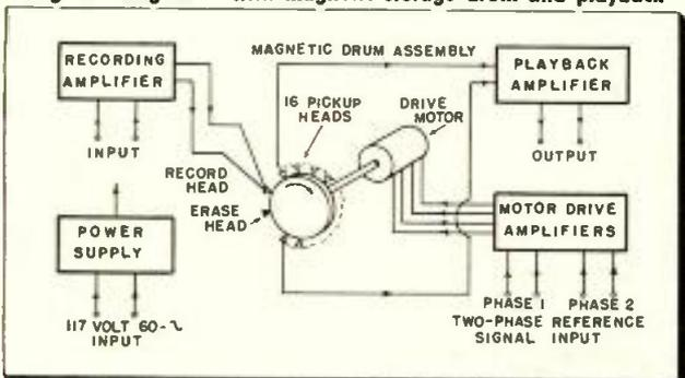
Fig. 4: Magnetic storage drum and playback, record and erase heads
