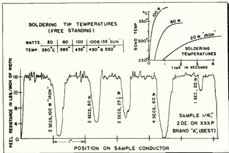
Fig. 5: Main curve depicts impairment of bond under hand soldering conditions. Temperature level reached by etched conductors being soldered can be judged from graph in upper right.
