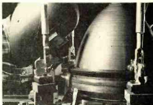
**9** Shielded by a welding mask, technician joins faceplate section of color TV picture tube to main cone, providing rugged air seal
