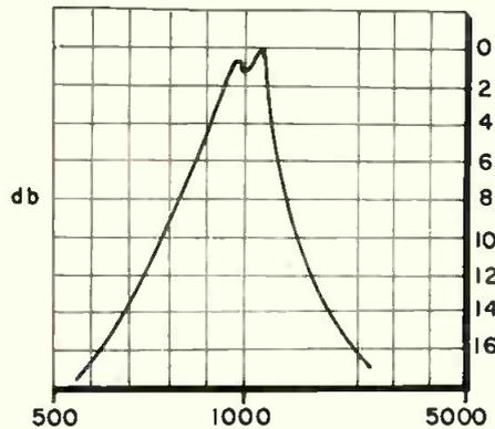
Response curve of telephone filter devised from FL 30 range filter and 1 meg. pot.
