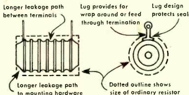
$+100^{\circ}\text{C}$  as compared with only 5 cycles from  $-55^{\circ}\text{C}$  to  $+85^{\circ}\text{C}$  required by MIL-R-93A. In qualification approval tests more rigid than MIL-R-93A, another leading eastern airborne electronic manufacturer reports that Shallcross "P" type resistors passed all tests without failure. Three other manufacturers tested had from one to nine failures in each test.
