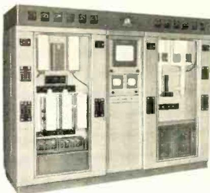
**GPL-CONTINENTAL TRANSMITTER:** 1 KW UHF unit with construction and performance far above standards of today. Space saving, but easily accessible. Air-cooled. No transmitter control console needed. Flexible for power increase.
