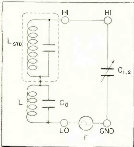
Fig. 10: Circuit for measuring coil inductance accounts for distributed capacitance
