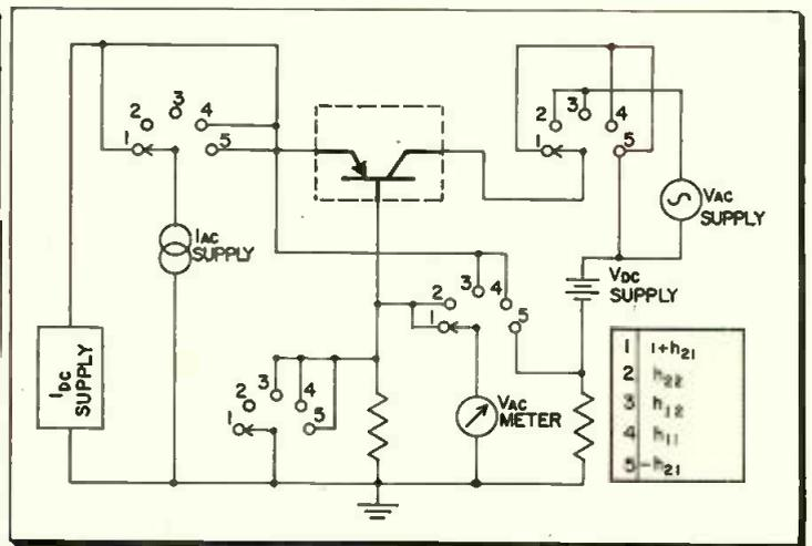
Fig. 2: Circuit for measuring h parameters
