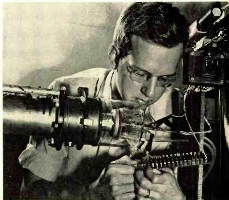
Electron gun of 6,000,000-volt linear accelerator undergoes tests. Apparatus developed at Stanford University is junior version of its billion-volt, 200-ft. accelerator. Gun shown will be attached to 6-ft. copper tube, through which electrons will be accelerated by SHF waves from klystron. Device is suitable for industrial radiography and medical X-ray and cancer treatment. It will be produced by General Electric, and made available in next few years
