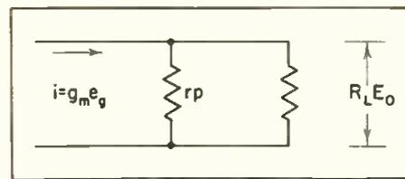
Fig. 6: Amplifier constant current equivalent
