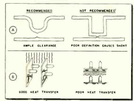
Fig. 11: (A) Adequate spacing of conductors avoids reduction of surface resistance (B) Properly orienting printed deck for heat transfer extends life and voltage characteristics
