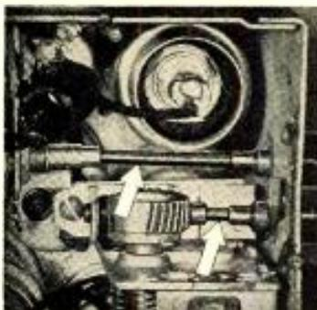
The flexible shafts reduced assembly time and labor, eliminated alignment problems and provided 100% vibration-free performance. In addition, it is apparent from the illustration that these coupling shafts give wide latitude in the placing of parts and make possible the most effective arrangement. It's savings
