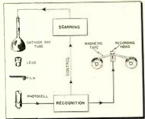
Fig. 2: In operation, scanning control directs CRT beam to appropriate area on microfilm. Information is picked up by photocell, converted into coded pulse form and recorded on tape
