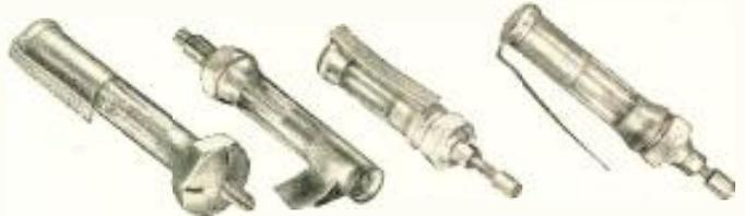
Corning Midget Trimmer Capacitors—have practically zero temperature coefficients in the VHF range. Capacity shift is negligible even with widely variable ambient temperatures. They're available in standard types covering the ranges of .3 to 3, 1 to 8, and 1 to 12 u.u.f., or we'll design them to your special requirements. With direct traverse trimming, there is negligible capacity shift under vibrations and an absolutely smooth capacity curve.
