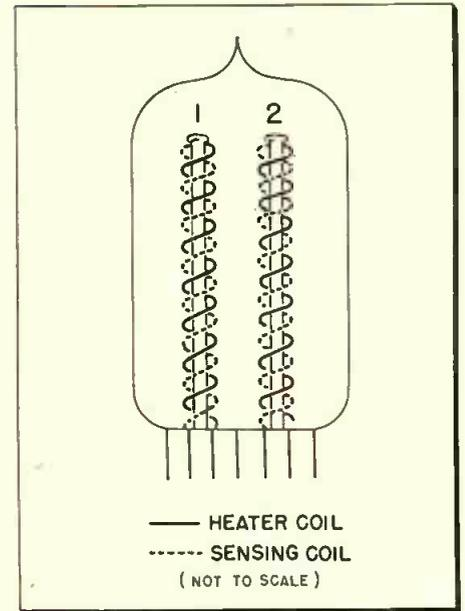
Fig. 6: Construction of thermal unit. Heating and sensing windings on rods are in thermal, but not electrical, contact with each other
