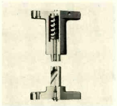
die assemblies are mounted in die sets and operate in a press in the same way as conventional dies, enabling unobstructed feeding. The units may be mounted directly to standard flat surface die sets, or on templates. Wales-Strippit Corp., 345 Payne Ave., North Tonawanda, N.Y.—TELE-TECH & ELECTRONIC INDUSTRIES.
