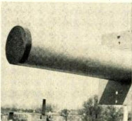
vantage can be taken of their decoupling possibilities in adjacent circuits, the units are made available in either the righthand or lefthand sense. The antenna consists of a molded 30-in. fiberglass helix with a 4 in. diameter that is rigidly mounted to a 16 in. sq. ground plate. Mark Products Co., 3547-49 Montrose Ave., Chicago 18, Ill.—TELE-TECH & ELECTRONIC INDUSTRIES.
