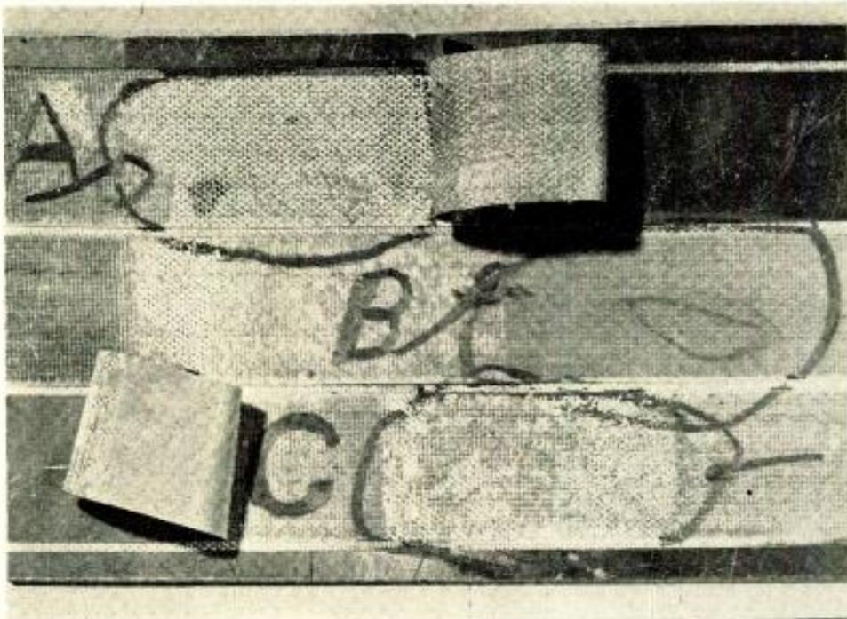
Fig. 4: Peel test samples show separation (a) at the copper-adhesive interface, (b) below the main interface, and (c) alternating between (a) and (b). (c) is strongest type of bond
