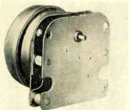
a wide variety of electrical appliances. The units are less than  $\frac{1}{2}$  in. in diameter and available in output speeds ranging from 450 rpm to 1 rev. in 31 days. Gear trains can be added to the basic unit to enable further speed variation. Gear pinion assemblies in reduction units are made of molded nylon which, in combination with "Lubricone", provides quieter operation and longer life. Sessions Clock Co., Forestville, Conn.—TELE-TECH & ELECTRONIC INDUSTRIES.
