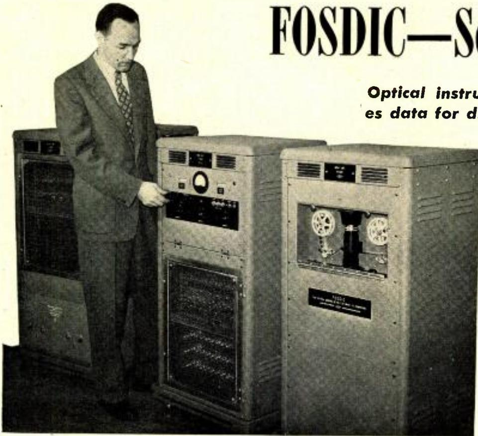
Fig. 1: Microfilmed copies of marked documents are read in FOSDIC cathode-ray scanning unit (r). Scanning generator (c) to drive CRT also receives photocell signals from scanning assembly. Answer information is fed to output unit (l) where it is converted into coded pulse form for magnetic tape recording. Power to all units are supplied from a fourth cabinet
