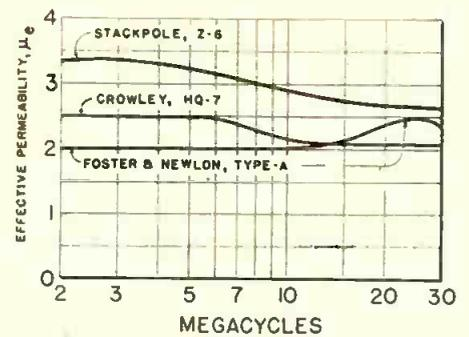
Fig. 6: Permeability-frequency characteristics
