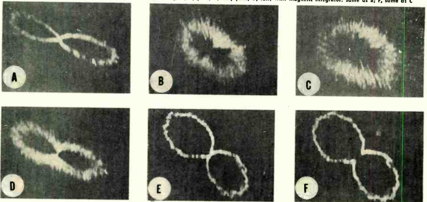
Fig. 8: Bearing presentations. A, poor signal; B, poor plus normal integration; C, poor signal plus integration and positive feedback; D, very poor signal; E, very poor signal plus normal integration; F, very poor signal plus integration and positive feedback
