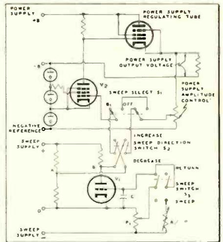
Fig. 3: Sweep circuit varies output voltage of regulated power supply at a uniform rate
