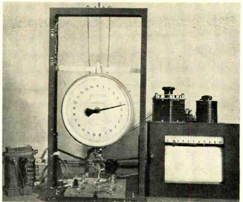
Fig. 1: (l) Samples of plated, etched and stamped wiring for radios. Fig. 2: (r) Extensometer set-up for stripping tests of clad laminates
