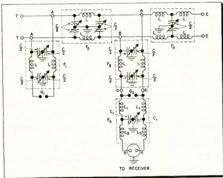
Fig. 2: Circuit diagram of duplexing system
