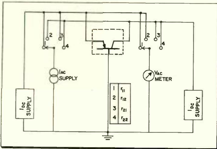
Fig. 1: Circuit for measuring r parameters
