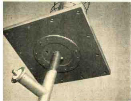
**SIMPLIFIED DESIGN** for fast transmission line hook-up! Power line may be readily removed or connected to the input feed adapter shown here. Beacon light cable feeds *inside the antenna* to eliminate any potential signal interference.
