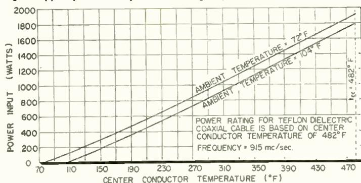
Fig. 8: (r) Comparison of experimental power ratings
