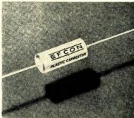
$\pm 1\%$  tolerances of any value from 0.01 to 1.0  $\mu\text{f}$  in 200, 400, and 600 v. dc voltage ratings, in standard miniature case sizes. The type of construction, it is said, provides high insulation resistance with very low dielectric absorption. Temperature range of the MH capacitors extends from  $-60^\circ$  to  $+125^\circ$  C. without derating. Electronic Fabricators, Inc., 682 Broadway, New York 12, N.Y.—TELE-TECH & ELECTRONIC INDUSTRIES.
