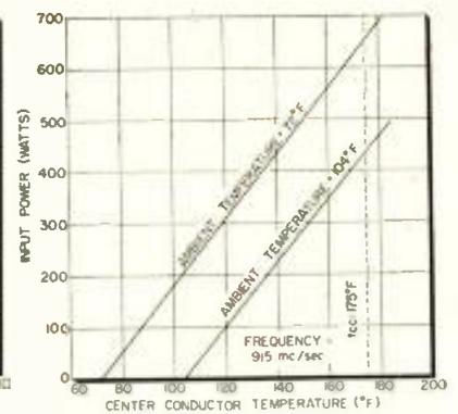
Fig. 5: (l) Experimental and calculated RG-8/U power ratings at various ambient temperatures.
