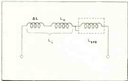
Fig. 11: Arrangement for determining iron core permeability in series measurement of a coil
