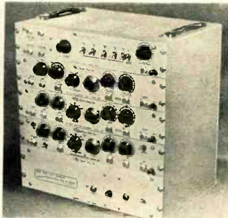
variable. Using no gas tube pulse-forming circuits, operation from either internal or external frequency are provided at repetition rates up to 100,000 cps with single pulse and gated operation. Main pulse amplitude is 80 v. maximum across an internal 93-ohm resistor. Electro-Pulse, Inc., 11811 Major St., Culver City, Calif.—TELE-TECH & ELECTRONIC INDUSTRIES.
