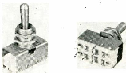
position off. Detent action gives positive "feel." Each pole of the switch element is rated at 6 amps, 125/250 vac, 30 vdc, resistive and 3 amps, 30 vdc, inductive. Weight is approximately 1 oz. Exposed parts are stainless steel or corrosion resistant. Electrosnap Corporation, 4218 W. Lake Street, Chicago 24, Illinois.
