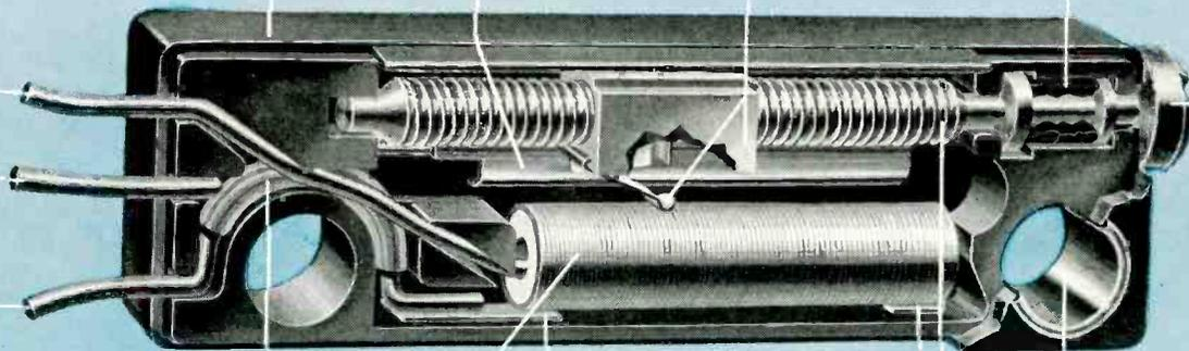
**TERMINALS**—Three terminals are gold-plated copperweld wire or Teflon-insulated leads.
