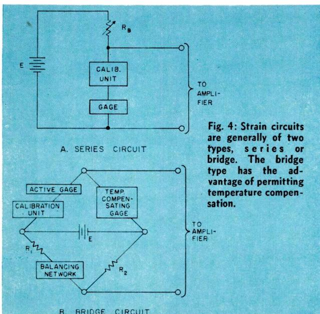
Fig. 4: Strain circuits are generally of two types, series or bridge. The bridge type has the advantage of permitting temperature compensation.
