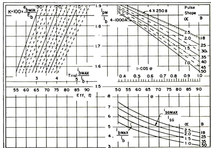
Fig. 2 (above): Charts used for the design of an amplifier.
