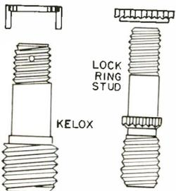
The Kelox stud serves the same purpose as the Keensert but is locked in position by a locking key ring which has two keys attached to it and which slides over the stud and is driven into the parent material.
