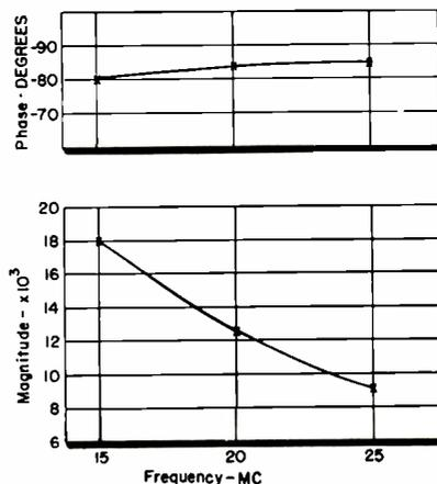
Fig. 8: Magnitude and phase shift of impedance represented by pole-zero plot of Fig. 7.
