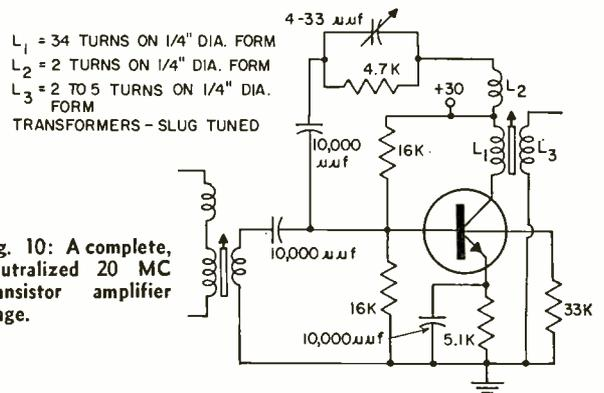
Fig. 10: A complete, neutralized 20 MC transistor amplifier stage.
