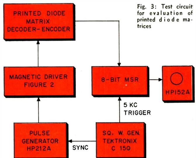
Fig. 3: Test circuit for evaluation of printed diode matrices
