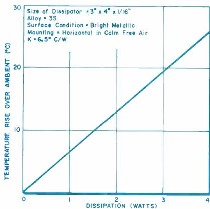
Fig. 1: Calibration curve for dissipator
