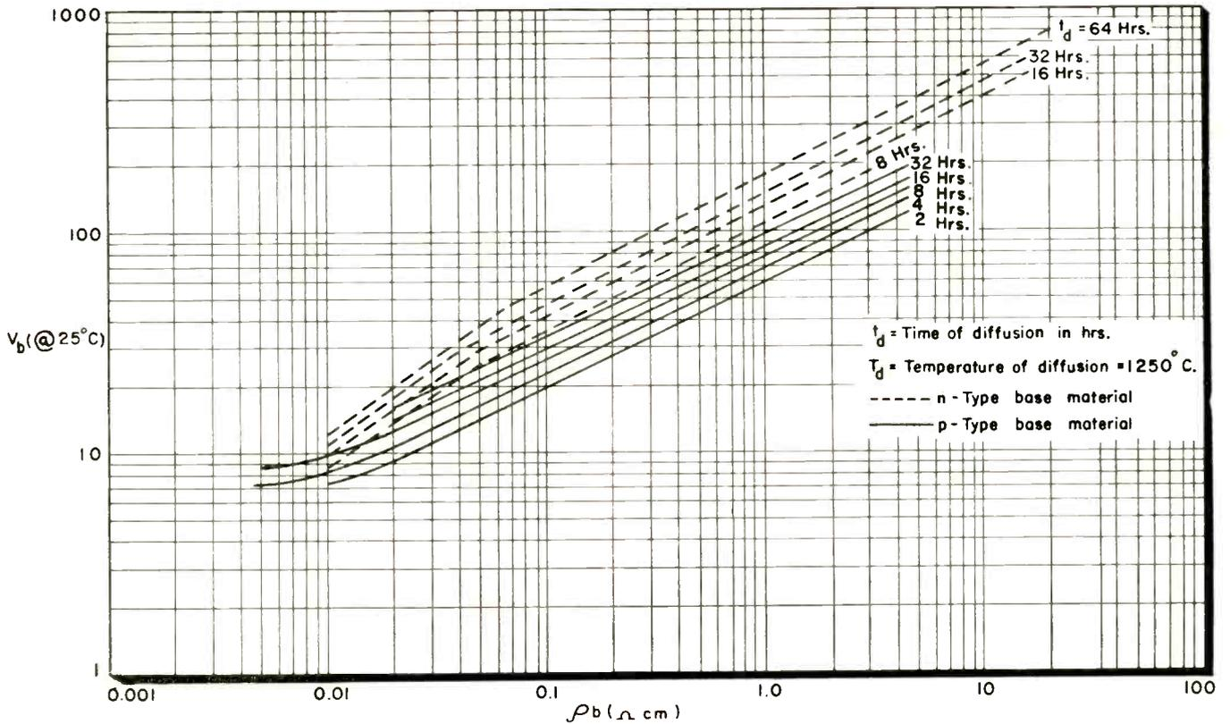
Fig. 7: Breakdown junction of diffused junction diodes measured at a reverse current of 10 ma., as a function of base layer resistivity for n- and p-type base regions with diffusion time as a parameter.
