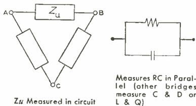
Wayne Kerr Universal Bridge, Type B-221 is a highly accurate transformer ratio arm bridge providing 2, 3 or 4-terminal measurement of impedance or transfer admittance over an extremely wide range. An impedance between any two terminals may be easily measured regardless of other impedances from either or both terminals and a third point. Measurement is unaffected by impedance of test leads.
