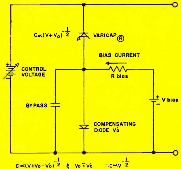
Fig. 4: Compensating junction circuit for temperature stabilization and extension of capacitance range.
