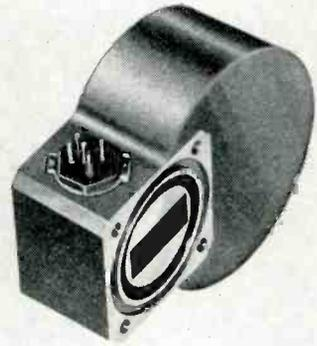
It may be used as a shutter or switch element. Featured are: Frequency Range 13.5 KMC  $\pm 15$  MC; Isolation at 25 db min.; Insertion Loss is indicated at 0.3 db max.; Input VSWR Transmit is 1.10 max. at center frequency; Input VSWR Reject 30:1; Rise Time at 100  $\mu$ sec max.; Control Coil Power at 2 w max. Ambient temperature 85°C to 105°C. Kearfott Co., Inc., Microwave Div., 14844 Oxnard St., Van Nuys, Calif.
