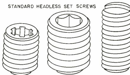
The cup point and flat point require no shaft preparation other than a flat while the other styles require deforming the shaft to accommodate the screw point. The flat point is usually used against hard materials and cup point against materials which are softer than the set screw so that it can dig in. Standard set screws are positively held in place during severe vibration by means of a sealing compound or by installing one set screw on top of the other.
