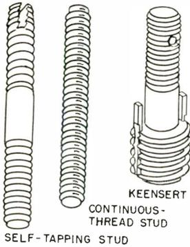
The most familiar threaded stud for small thread sizes is the continuous thread stud which has thread for its entire length and is chamfered on both ends. These studs can be obtained from any specialty house in various materials and thread sizes, or cut from longer lengths.
