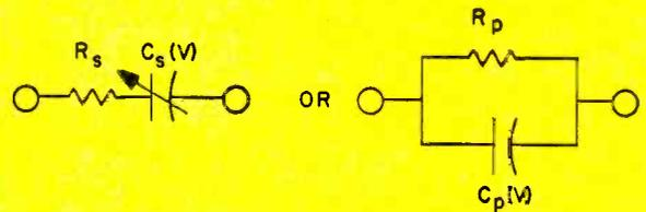
Fig. 1 Equivalent circuit of the voltage variable capacitor can be simplified to an equivalent series resistance and the capacitance which is a function of the applied voltage.
