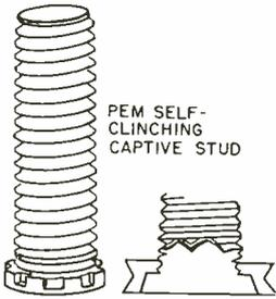
The Pem Stud has the same applications as the National stud. A hole slightly larger than the nominal thread size is drilled in the panel and the stud pressed in. The panel material cold flows into a circular portion between the threaded portion and the stud head, while the many grooves around the head act as the anti-torque
