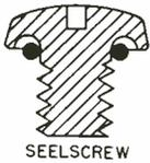
Seelscrews are specially designed machine screws with a silicon rubber "O" ring seated under the head. The "O" ring deforms as the screw is tightened and fills the void between the screw and the assembly creating a seal against the escape or access of liquid or gas. The "O" material can seal pressures as high as 500 PSI and can be used over a temperature range of  $-120^{\circ}\text{F}$
