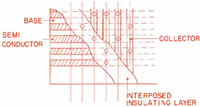
Fig. 1a (left): Layer Structure of the printed diode matrix.
