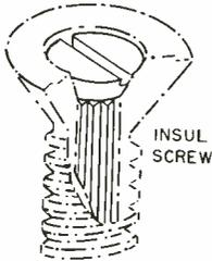
The Insul-screw is a nylon screw with a metal core. This metal core increases the shear strength of the screw over a straight plastic screw while the plastic gives the insulation properties and anti-corrosive properties.
