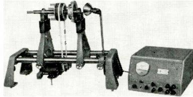
100 lbs., as well as a wide range of operating-balancing speeds. It is suitable for nearly every type of rotor up to a maximum diameter of 24 inches . . . fans, armatures, blowers, pulleys, crankshafts, propellers, impellers, etc. Micro Balancing, Inc., Garden City Park, New York.
