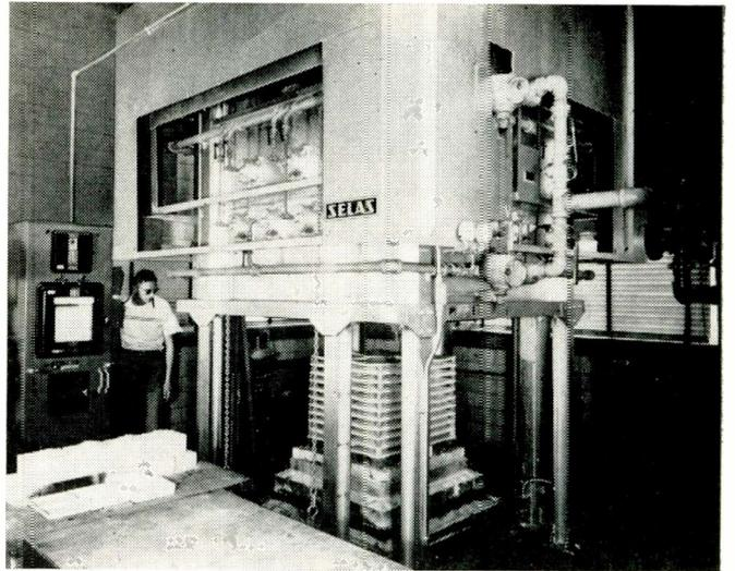
The heating unit was specially designed and built by Selas Corporation of America, Dresher, Pa., to fire ceramic piece parts such as cathode support insulators for microwave amplifier tubes and structural members for other electron tubes. As many as 12,000 pieces at a time can be uniformly heat processed in this kiln with a minimum of rejects.
