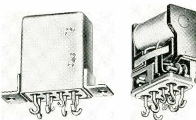
R-575C and MIL-R-25018. Standard operating coils are 26.5 vdc nominal—coil resistance, 400 ohms. Weight is 3 oz. Size is  $\frac{5}{8}$  x 1-1/32 x 1 1/4 in. Hook type and long and short wire lead terminals available. Headers have 0.2 in. grid spacing. Struthers-Dunn, Inc., Pitman, N. J.
