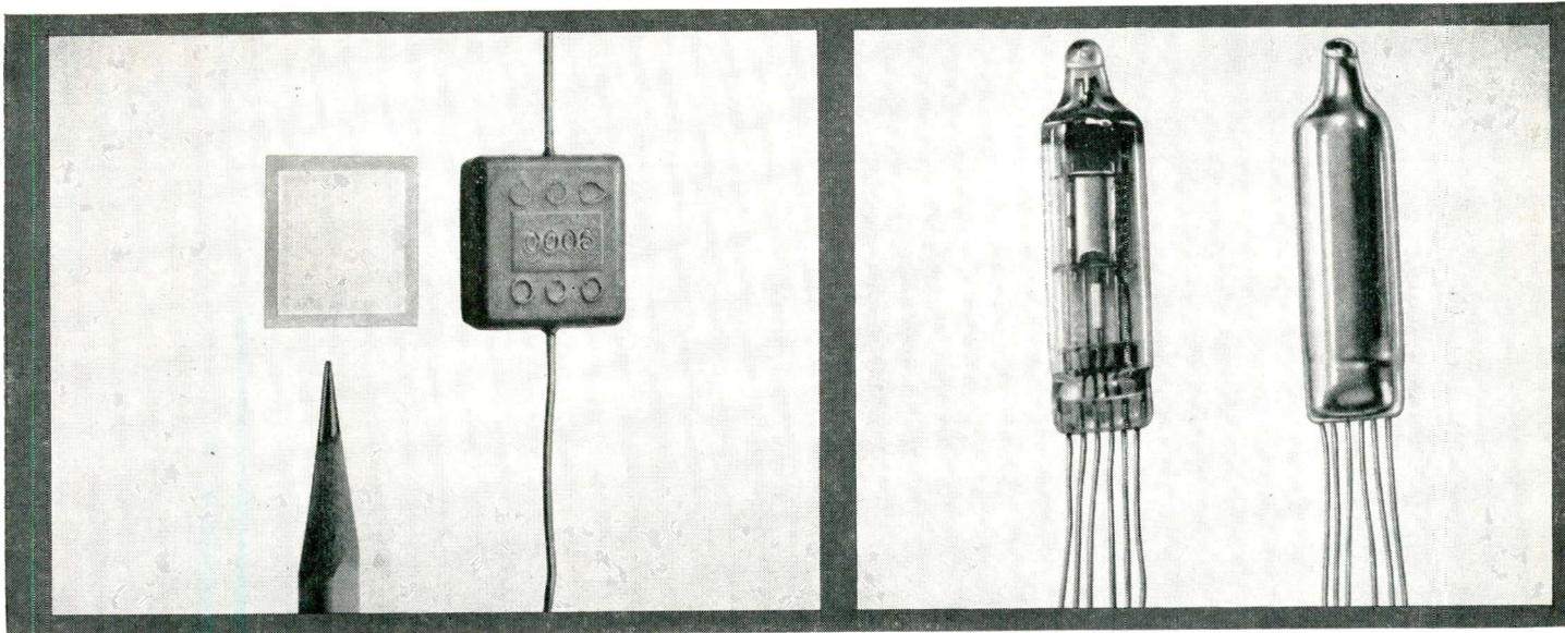
• This mica film has been coated with special Du Pont silver preparations and is used in the manufacture of silver-mica capacitors (shown above).
