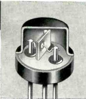
CBS NPN switching transistors have proved themselves in flight in many of our important "birds." They have been found to have the advantages of fast switching, high voltage, low cutoff current, and low saturation resistance. All 28 of these CBS transistors exceed the MIL-T-19500A specification.
