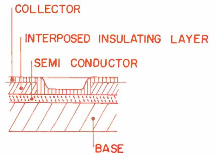
Fig. 1b (right): Cross section through a single diode junction.
