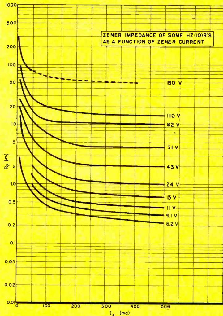
Fig. 9: Reverse breakdown impedance as a function of reverse current.
