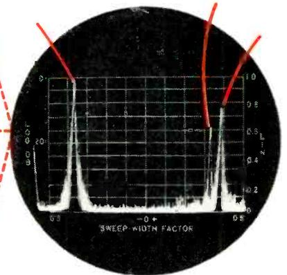
Interference analysis with Model SA-8b Panadaptor. Sidebands from AM channel #3 is seen to spill into band occupied by intermittent CW channel #2.
