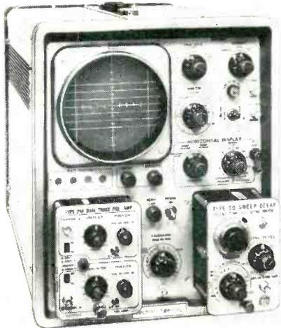
others that simplify operation and waveform analysis. In addition to a plug-in sweep delay, several plug-in pre-amplifiers are available. The dc to 20 MC, 0.05 v/cm Type 20A "Plug-in" serves the majority of single-channel applications. An electronic switch pre-amplifier "Plug-in"—Type 20B—is available for dual trace applications. Other pre-amplifier "Plug-ins" will be produced to meet specific needs. Electronic Tube Corp., 1200 E. Mermaid Lane, Philadelphia 18, Pa.
