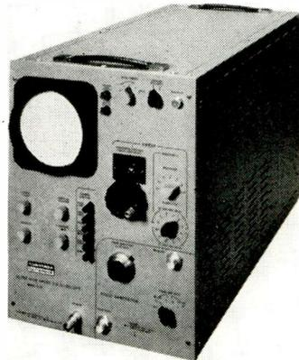
nal-to-noise ratio. Samples are taken from the successive, unamplified repetitive pulses under investigation, and their amplitudes are sampled for a very small time interval (400  $\mu$ sec), amplified, stretched to about 1 msec. and displayed as a composite picture of the pulse shape on the CRT. Lumatron Electronics, Inc., Westbury, L. I., N. Y.
