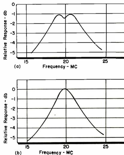
Fig. 9: Response at point A in Fig. 5, with stage 2, (a) unneutralized and (b) neutralized.
