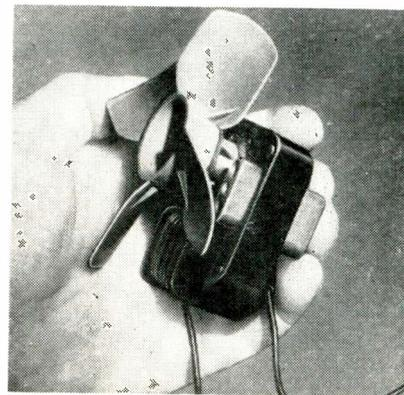
220 50/60 cycle voltage. Rotor turns at 3400 RPM with recommended loads, horsepower ratings 1/750 to 1/185. Operates from -10 to +250°F. Dept. 26, Howard Industries, Inc., 1760 State St., Racine, Wis.
