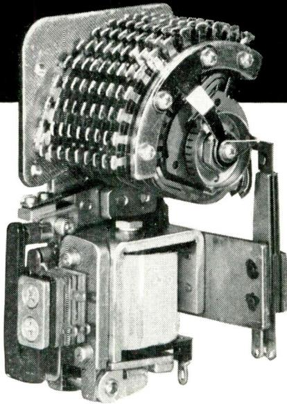
**Eleven-point stepping switch has 12-level capacity, 100,000,000-step\* life**
