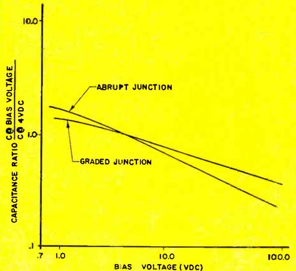
Fig. 2 Capacitance vs voltage relationship for the abrupt junction shows an inverse square root relationship; the diffused junction shows an inverse cube root relationship.
