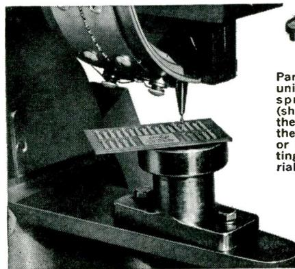
Part of the secret's in Segal's unique anvil tool holder and spring loaded work table (shown at left) which allow the eyelet to pass through the assembly before staking or flaring. Avoids loose settings, compensates for material variations, too.
