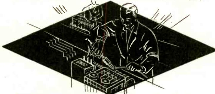
Rugged construction, low power consumption, and the application of "Balanced Heat" principle of construction, actually increases soldering efficiency substantially. Costly tip replacements and element burn-outs are minimized because hexagon-shaped barrels dissipate 20% more excess heat when irons are used intermittently.
