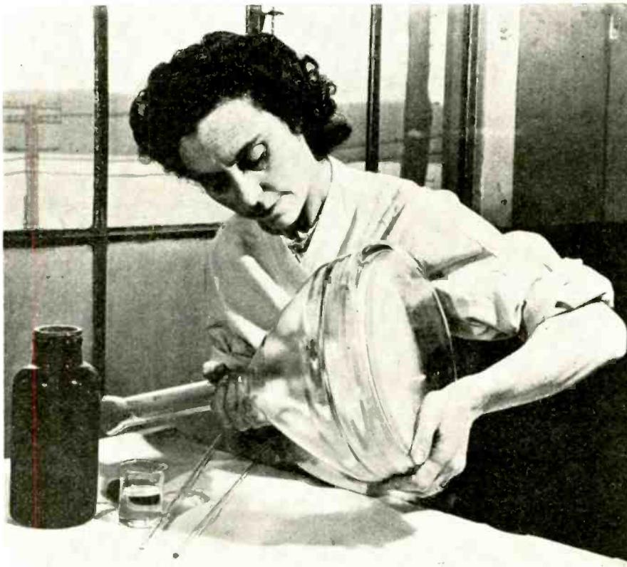
Fig. 18—Dusting a phosphor coating on a large (10 in.) cathode ray tube
