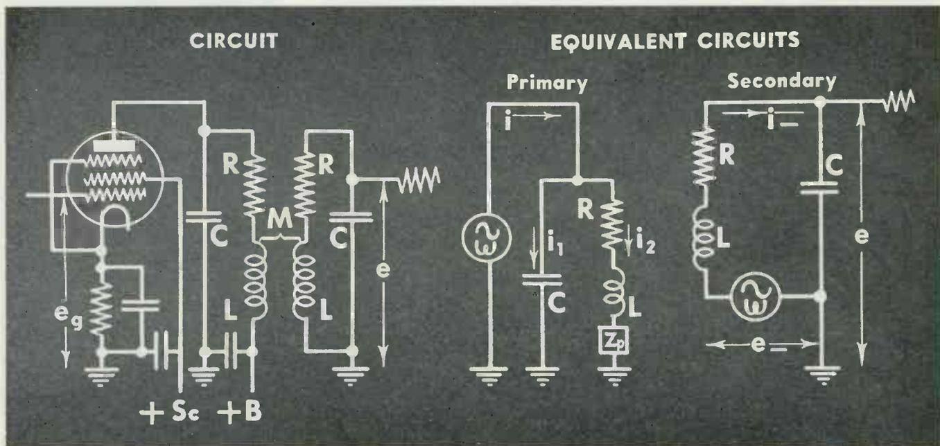
$$(3) \omega = 2\pi f = 2\pi(f - f_0 + f_0) \\ = 2\pi f_0(d+1) = \omega_0(1+x/2)$$
