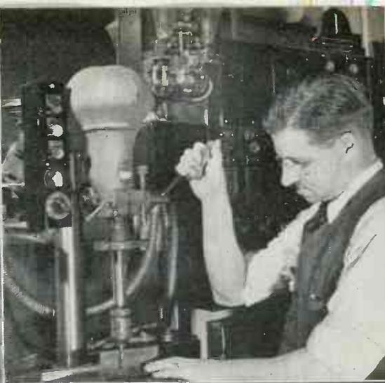
← **MOTOR CONTROL** on drill press at G-E Scheenady plant gives constant speeds of 25 to 1750 rpm, allows tapping, fly-cutting, and drilling molded compounds at controlled speeds
