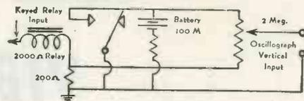
Circuit used for obtaining above oscillograms. Battery voltage appears on oscillograph input except when shorted by closed contacts. Voltage developed across 200 Ohms resistor used to indicate relay coil current. All oscillograms untouched photographs. 30 cycle sweep.
