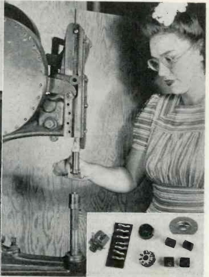
**FORMING SMALL PARTS** with a riveting machine. At Emerson Radio and Phonograph Corp., N. Y. C., a standard riveting machine was drafted into service to press out small parts. Fitted with proper punches and dies, the improvised forming-machine has been entirely successful. Sample parts shown at bottom right
