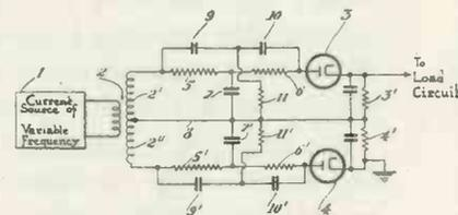
creased or decreased. Filter network 5',6',7',9',10',11' has a similarly shaped impedance-frequency characteristic, the maximum-impedance frequency being  $f_2$ . Frequencies  $f_1$  and  $f_2$  are located at, or even beyond, the extremities of the frequency deviation range of the applied frequency-variable waves. Their mean represents the center frequency of the input voltages. Since at that point the impedances of the two networks are equal, the voltages developed across resistors
