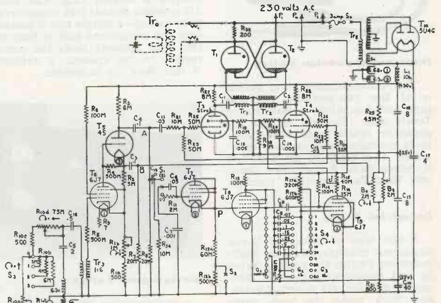
WELDER control circuit adjustable between one half-cycle and 60 half-cycles
