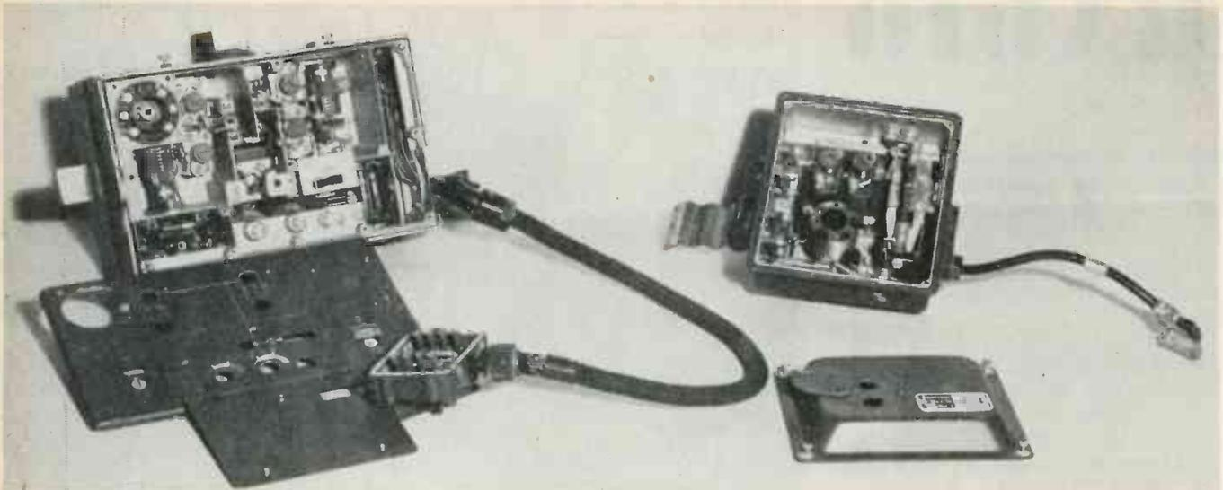
BLIND landing equipment used on the Messerschmitt Me 110 fighter plane operates on the Lorentz system and consists of two units, the beacon receiver and the marker beacon receiver, both operating through a common audio amplifier
