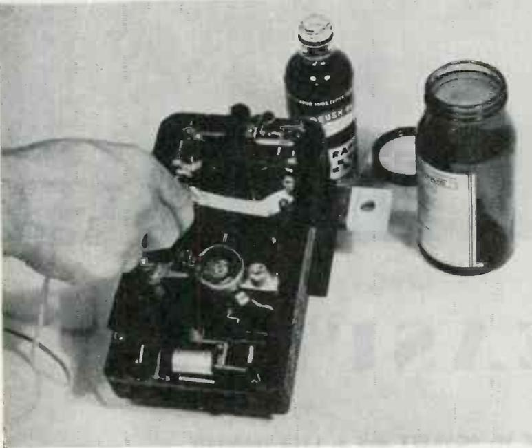
**LOCAL SILVER-PLATING** of electrical equipment to reduce contact resistance with portable apparatus developed by Rapid Electroplating Process, Inc., 1414 So. Wabash, Chicago. Powered by rectifier or battery, swab-like applicator anodes are used, with electrolytes for silver, gold, zinc, copper, nickel, tin, or cadmium plating
