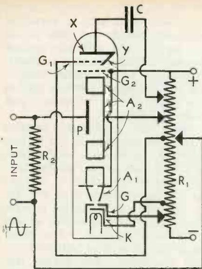
Fig. 6. Scanning wave generator directly synchronized
