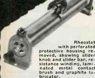
Rheostat with perforated protective housing removed, showing slider knob and slider bar, resistance winding, laminated metal contact brush and graphite lubricator.
