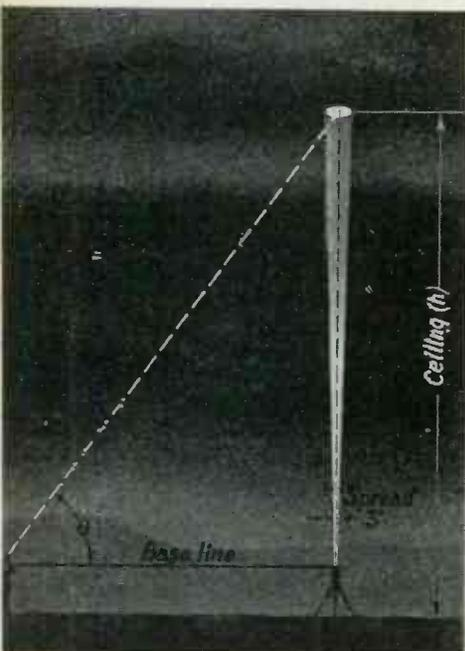
Fig. 1. Basic method of measuring cloud height.  $h = \text{Base line} \times \tan \theta$ . Night-time observer uses clinometer on visible reflection from high-intensity light-source
