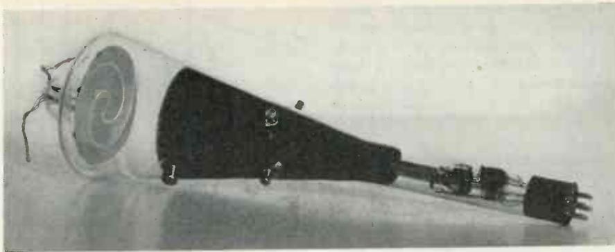
Fig. 4. Shelby system for producing phase-modulated signals
