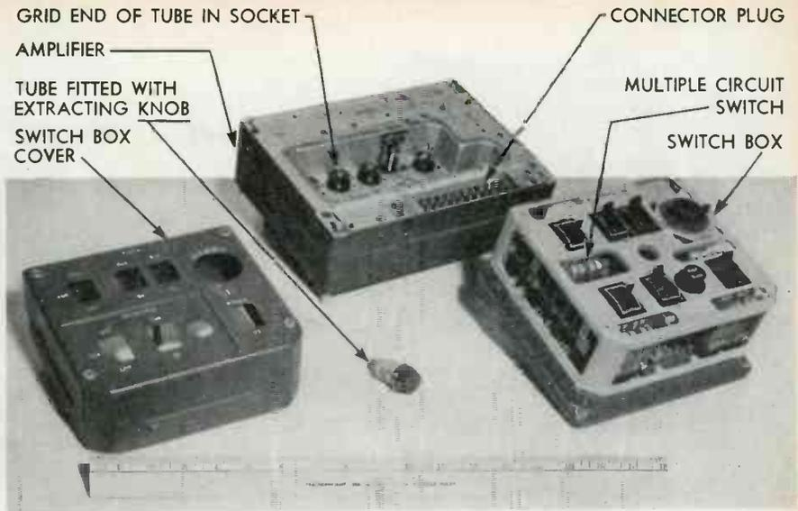
AMPLIFIER and switch control units used in the Messerschmitt interfone unit
