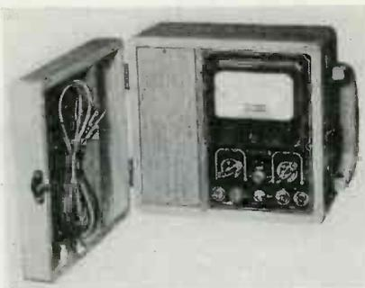
high degree of accuracy both as a resistance measuring instrument and as an insulation tester. Housed in a heavy-duty oak portable cabinet with a bakelite panel the device measures 9 ½ x 8 ½ x 6 in. When battery operated, the 500 v. potential is made available by means of an integral vibrator power supply by throwing a front panel toggle switch. Price \$62.50. Another model, 610-E, operates on 110 v. ac and is available for \$52.50.
