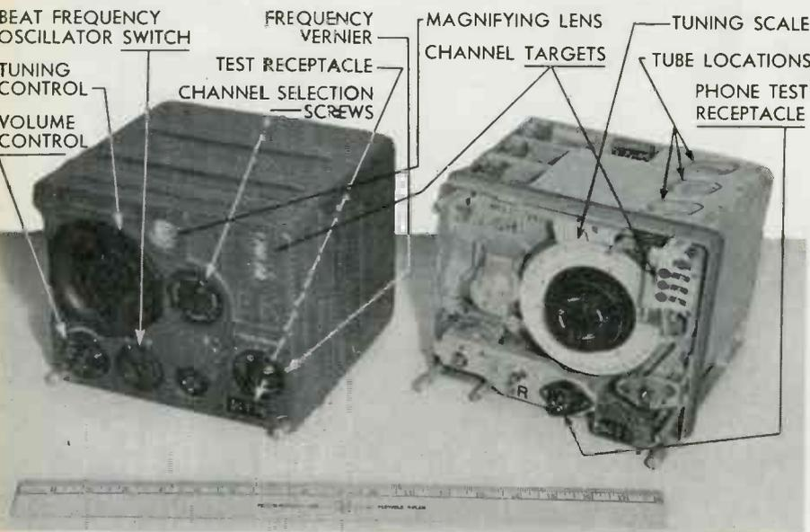
EXTERNAL and interior construction of the long and short wave receiver units
