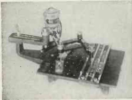
For lettering panels of steel, aluminum, brass, or bakelite, or for marking finished apparatus.
