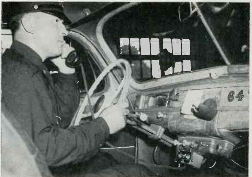
EACH of the 70 mobile police units carries AM receiving equipment and for talk-back operators rely on 25-watt FM transmitters on 35.1 megacycles
