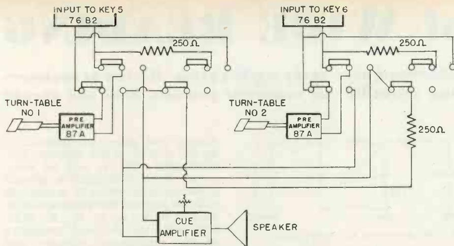
**CIRCUIT** diagram of WINS method for cuing and presetting transcriptions, developed by studio engineer, J. B. McNally
