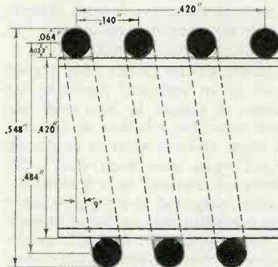
Fig. 2. Three turn wire-wound coil
