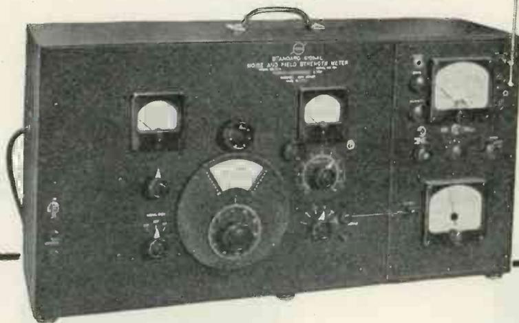
Model 22-32 is a versatile instrument designed to meet the need for a precision meter combining in a single unit, the measurement of sensitivity, noise and field strength.
