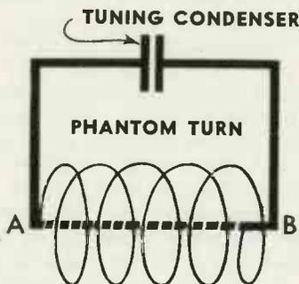
Fig. 7. Showing effect of lead connections external to the coil
