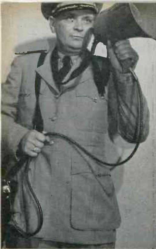
**P.A. MEGAPHONE** for use on merchant vessels, made by Guided Radio Corp., N. Y. Mike and speaker in megaphone, amplifier slung over shoulder
