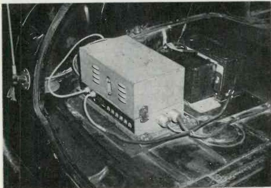
INSTALLATION of mobile equipment including the Link 25-watt transmitter, the power supply and receiver for AM, arranged for quick servicing
