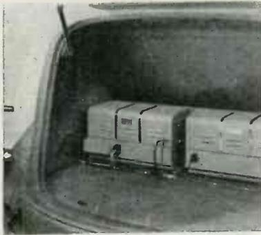
Complete 22 Watt High Frequency Mobile Installation
