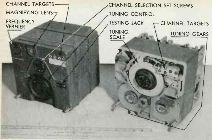
LONG and short wave transmitters used on the Messerschmitt Me 110 airplane
