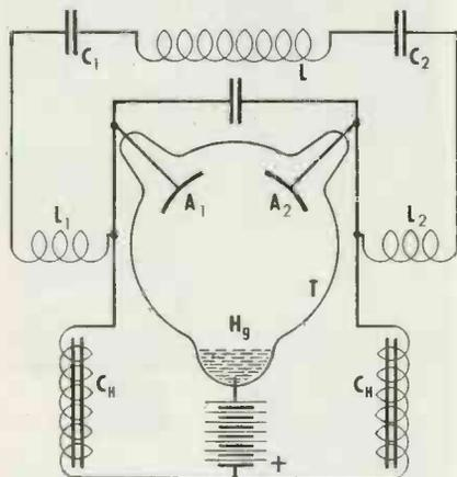
determined by these constants. Stable operation is aided by the inductive chokes in the anode supply leads, shown as C<sub>H</sub>. The Vreeland tube is thus, basically, a synchronous switch.
