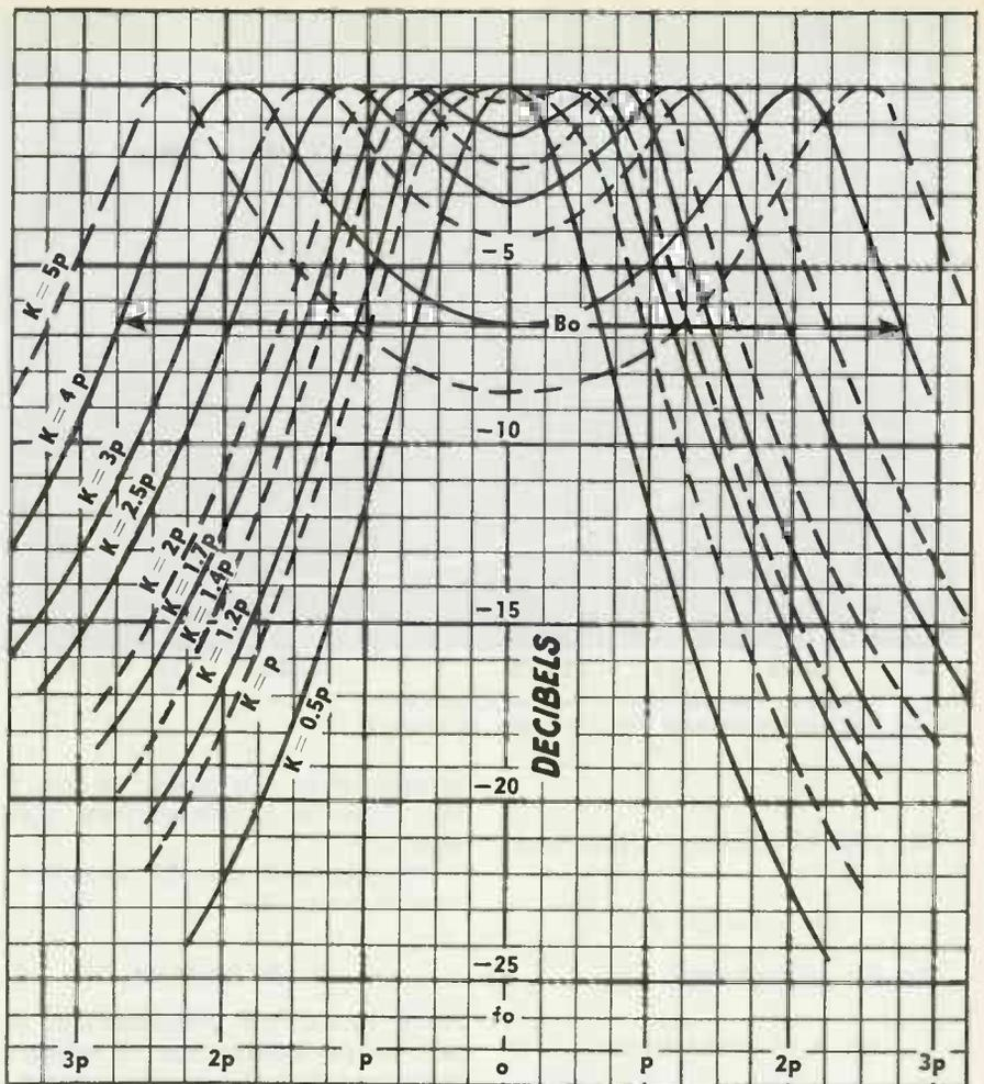
Fig. 2. Here the scale of abscissae is pure number; that is, units of  $p=1/Q$ . To convert to frequency, multiply by  $f_0$ . For example, if the  $Q$  of the coils is 20, and the center-frequency is  $f_0=10$  mc, then each division ( $p$ ) represents  $pf_0$  cycles  $=0.05 \times 10$  mc  $=500$  kc
