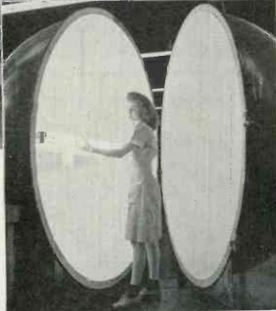
← **LIGHT MEASUREMENT** with seven ft. sphere and phototube checks radiation of fluorescent lamps
