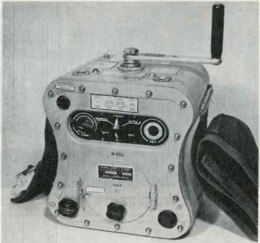
Emission is 500 kc, ICW, the modulation frequency 1000 cycles, modulation in excess of 100 per cent. The transmitter may be automatically or manually keyed. The sig-
