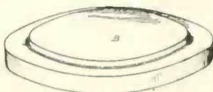
ous essential properties and characteristics above pointed out, by combining equal parts of ozocerite and paraffin. Such a composition is found to be tough and smooth in texture. The shaving formed by the recording point is continuous and does not break into bits and stick to the surface of the record or clog the point of the stylus. The record groove is clean cut and the walls or surface thereof are smooth and entirely free of inequalities.
