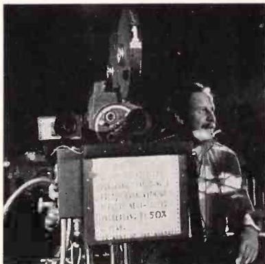
Tv camera mounted on right side of film camera is used as monitor.
