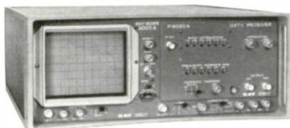
sweep of the Kay 159D, 160A, or 162A sweep signal generators. Kay reports that a system can be swept with the loss of less than one line of video information, thus allowing testing without interruption of subscriber service.
