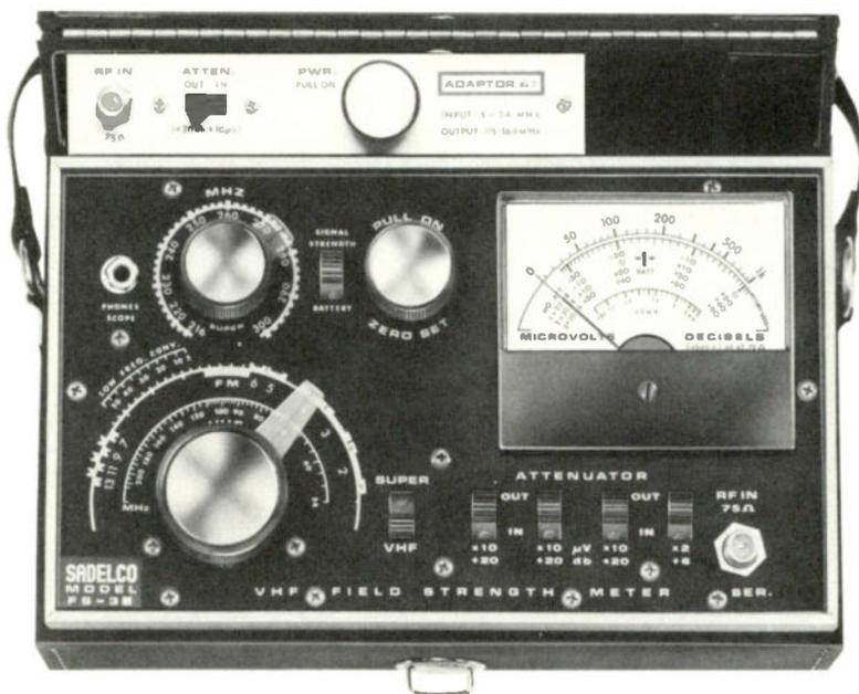
Range does not end at 250 or 260 MHz but covers complete new band flat to 300 MHz (no high end roll-off).
