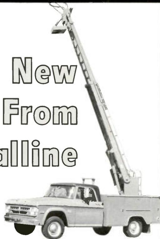
The HALLINE Model EMES-25SLA Aerial Ladder is a compact and versatile unit, designed to mount on a 3/4 Ton chassis (built up to camper special specifications) with single rear wheels. Mounting the EMES-25SLA on a 3/4 chassis provides a unit that is easy to handle in heavy vehicle traffic or confined space at the job site. The EMES-25SLA with its counter-weighted pedestal design is completely stable without the use of outriggers or ballist added to the chassis frame.
