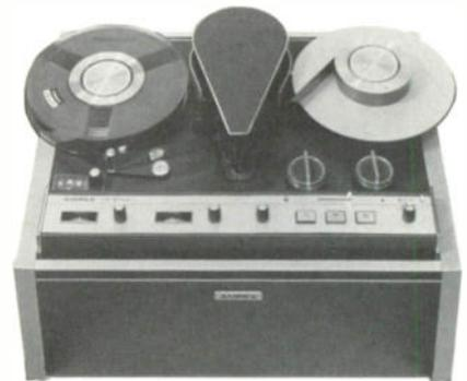
feature four-minute rewind and fast forward speeds. Both units operate at a tape speed of 9.6 inches per second, a writing speed of 1,000 ips, and offer one hour of playing time.
