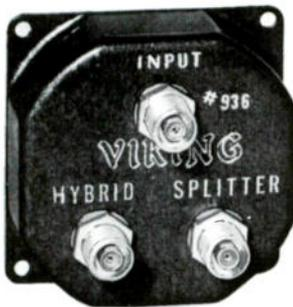
This coupler has a frequency range of 50 to 220 MHz and a 75 ohm impedance on all terminals. The unit has a low VSWR of 1.2:1 maximum input, and 1.3:1 maximum output. Its thru-loss is 3.5 dB maximum. Only \$3.75 each.
