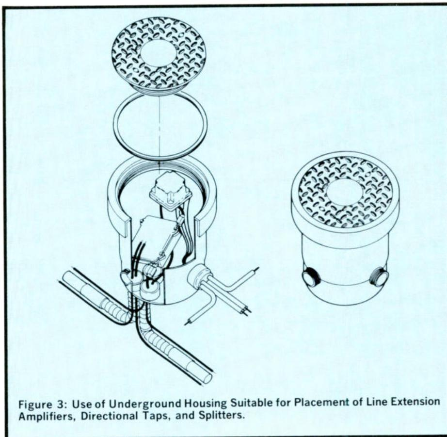
Figure 3: Use of Underground Housing Suitable for Placement of Line Extension Amplifiers, Directional Taps, and Splitters.
