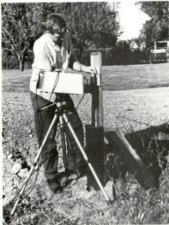
The portable field X-Ray unit can be mounted on a tripod and used to check splices made in pedestals. Here, the technician tapes polaroid film to the splice.
