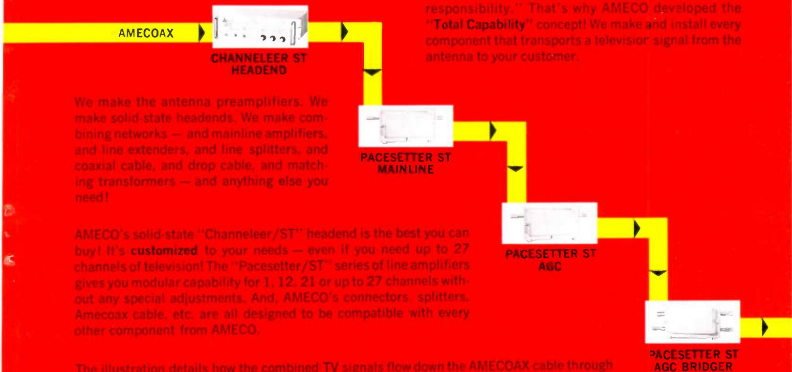
We make the antenna preamplifiers. We make solid-state headends. We make combining networks — and mainline amplifiers, and line extenders, and line splitters, and coaxial cable, and drop cable, and matching transformers — and anything else you need!
