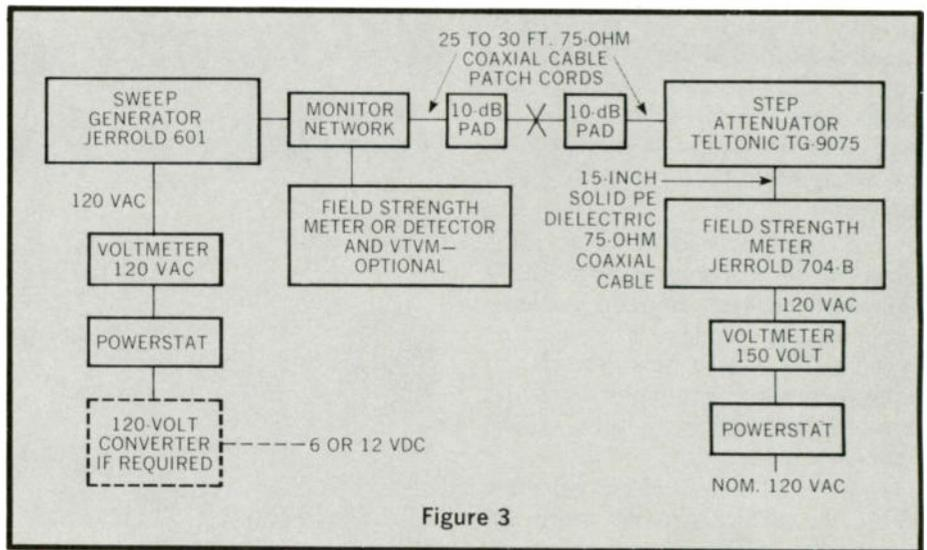
(a) Sweep Generator—1. ALC: about 80% max. (mark knob position). 2. Horizontal Phasing: approximately 50% max. 3. Sweep Range: 45 to 225 MHz (or as desired). 4. Sweep Width: Max. (sweep width should extend at least 2 MHz beyond range to be measured). 5. Switch Attenuator: 10 dB "in." (b) Step Attenuator—1. Switch in sufficient attenuation that a
