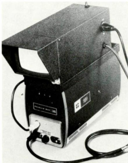
can economically convert them to viewfinders. Two models are available: one for the PB-920 (as shown) and one for the PB-940. Both are offered with zoom lens controls as PB-920VFZ.
