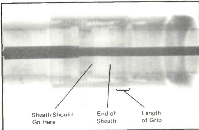
Sheath Should Go Here      End of Sheath      Length of Grip
