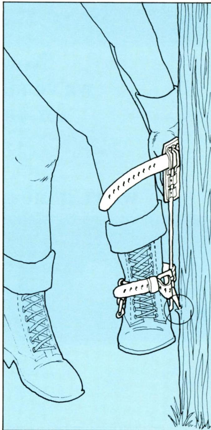
1. Select a location on the pole that is free and clear of gaff marks, cracks and knots.
