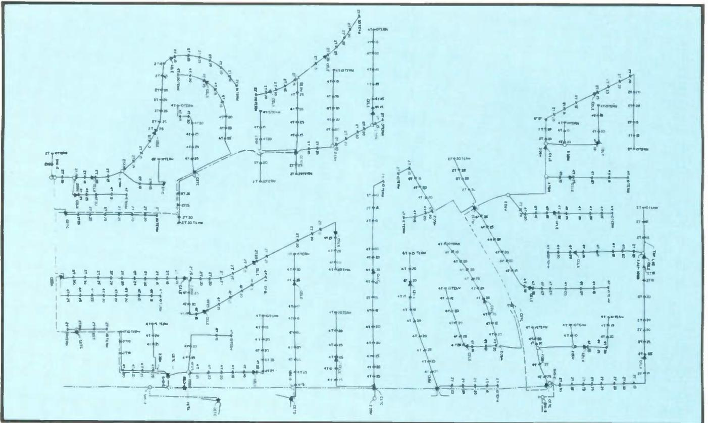
By varying light exposure time while photo-map prints are being made, the aerial photo detail can be "burned out" completely so that only the strand map remains. A portion of one photo-map is shown at actual size below.
