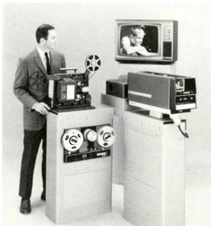
equipment. The camera can be quickly removed from its pedestal and with the addition of a standard zoom lens can then be used for normal cablecasting applications. The film chain can be expanded to a multiplex system having up to two more sources—16mm and 2x2 slides. Film chain camera output is NTSC type color that can be utilized by color RF modulators.
