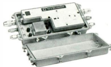
the manufacturer lists the following features: each amplifier has its own integral, line-isolated, regulated power supply; the units are modular; each mainline amplifier includes a full range of attenuators (3 dB, 6 dB, 9 dB and 12 dB), while the line extender is provided with a zero dB and 6 dB plug-in attenuator; and plug-in line equalizers (8 dB, 12 dB and 17 dB standard) are provided as specified for the normal range of cable and amplifier spacing.
