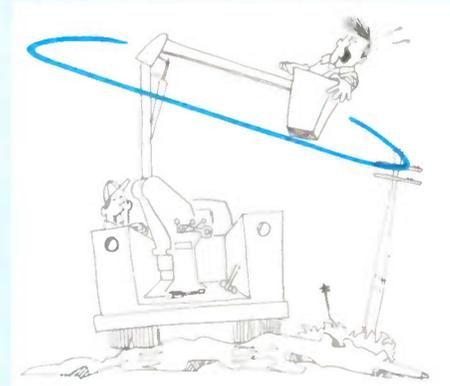
Sam has decided to make several minor adjustments in the field . . . while Norman tries his hand at some work. Sam fiddled around the lower controls and left a tool lying on them. The tool, of course, actuates the rotation lever and Norman is off on an unscheduled trip.
