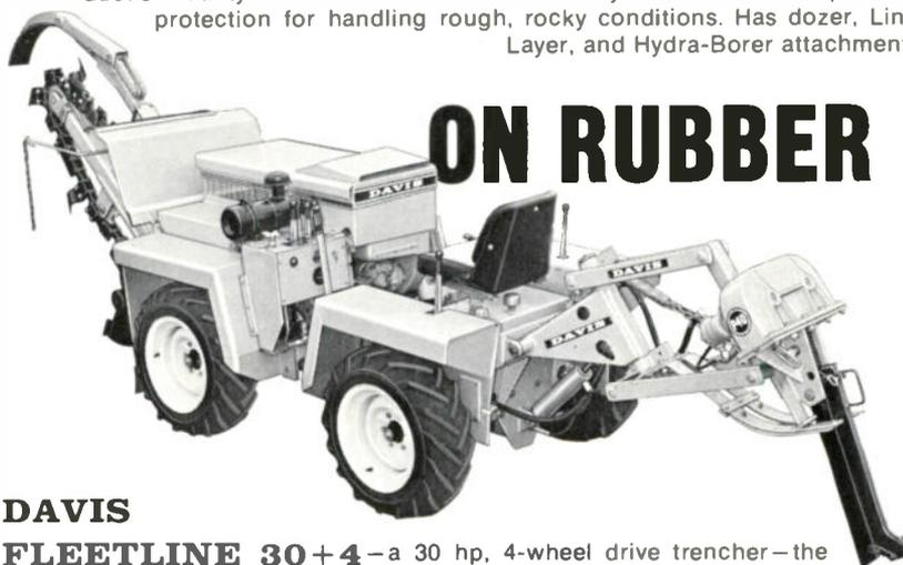
**DAVIS FLEETLINE 30+4**—a 30 hp, 4-wheel drive trencher—the closest thing to tracks on wheels. Exclusive Hydra-Static axle puts full-time traction to all four wheels when trenching, dozing, or laying cable. Has patented hydraulic articulated steering. Available with Line-Layer attachment, as shown, or dozer, or backhoe...plus an all-weather cab.
