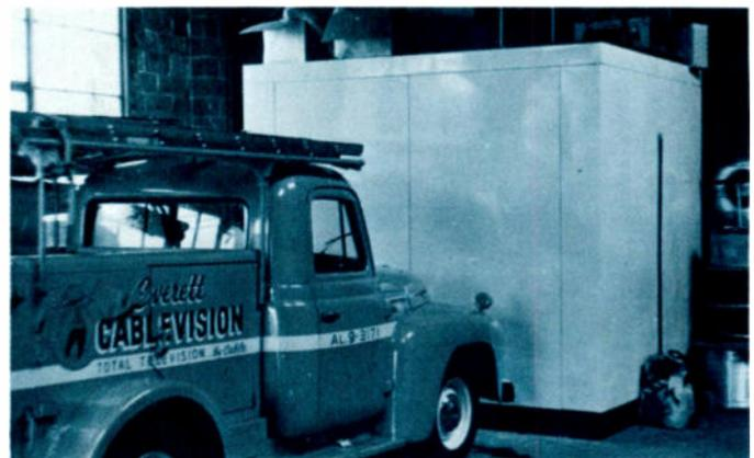
*The climate chamber used in the equipment testing facility protrudes into the garage area of the Everett Cablevision offices. The freezer room has an operating range of 30 degrees below zero to 140 degrees above zero.*
