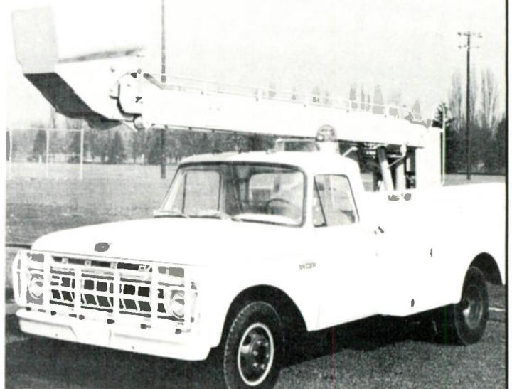
The EME is designed for any type of maintenance work. Choose from 4 models with extended platform heights of 26' to 35'. Four types of work platforms and baskets are available. Looking for a self-contained unit? The HALLINE EMH is your answer. Completely self-powered by a 9 h.p. gasoline engine housed in ladder base. Equipped with 110 A.C. outlet for use of electric power tools. 3 models available, 26'6" to 35'. CATV's best buy in self-contained ladders!
