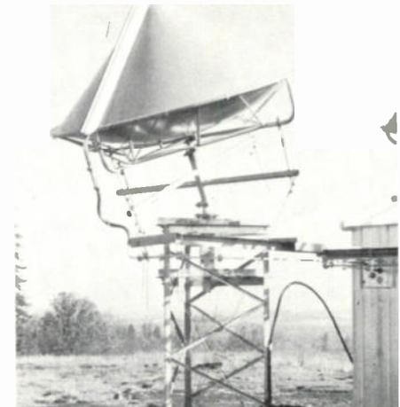
Microwave antenna used to illuminate a tower-mounted reflector.
