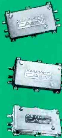
**THE INSIDE STORY** of the Phoenician Amplifier series. Modular construction of the "plug-in" type allows complete interchangeability from trunkline amplifier to 2 and 4-output bridging amplifier — or combinations of trunkline and bridging amplifier (with or without AGC and automatic tilt). Built-in knob type controls eliminate the need for screwdrivers, plug-in pads or accessories.
