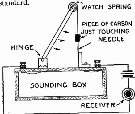
This microphone for the amateur experimenter has an extremely sensitive contact and will give remarkable results.
