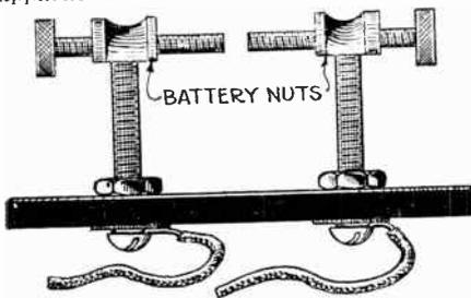
The acme of economy is achieved by this ingenious adjustable spark gap constructed of machine bolts and "dry-cell" binding screws and nuts. Besides economy and efficiency, it has the added virtue of neatness.
