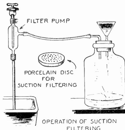
Filtering by a vacuum; a simple filter pump draws air from the large bottle so that the liquid is forced by atmospheric pressure through the filter paper.
