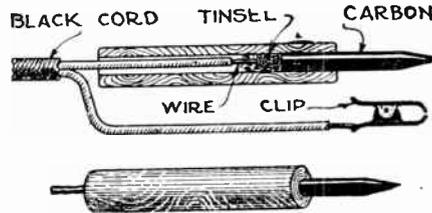
This soldering "iron," built around a battery carbon, melts the soldering wire through which the heating current passes, when the wire is brought in contact with the carbon tip.
