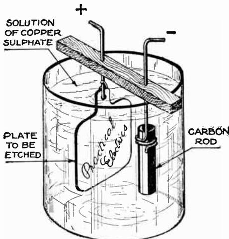
A simple rigging for etching by the electrolytic process; an outside source of electricity is required.
