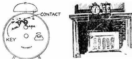
This switch is adapted for use on the ordinary alarm clock and is so arranged that the key makes contact and closes a circuit when it revolves, due to the winding off of the alarm, but does not make contact when winding up the alarm, in which case the contact point is turned to one side. It is used for operating buzzers, bells, lamps, etc.
