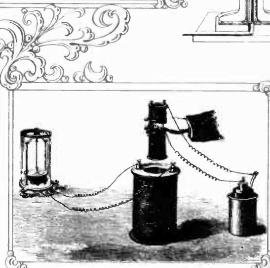
Electromagnetic induction is illustrated strikingly by the famous Faraday experiment shown at the left. The small coil carrying a current induces a current in the large secondary when dipping into its core. The secondary current is indicated by the galvanometer at the left.
