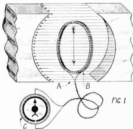
Diagram explaining zero potential induction. A coil of wire cuts a field of force without result.
