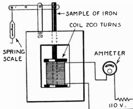
This apparatus, readily constructed, will enable the experimenter to investigate the magnetic properties of the iron used in his experiments.
