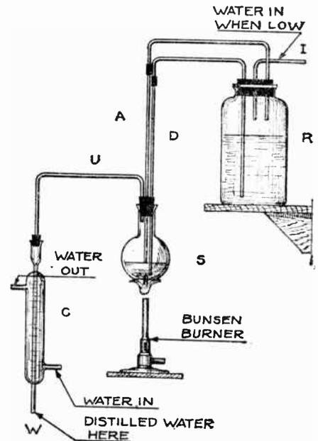
Diagram of the continuous still, showing its mode of operation.
