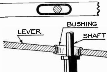
A section showing the arrangement of the lever for the vertical motion of the drill. Notice the oblong hole for the shaft.
