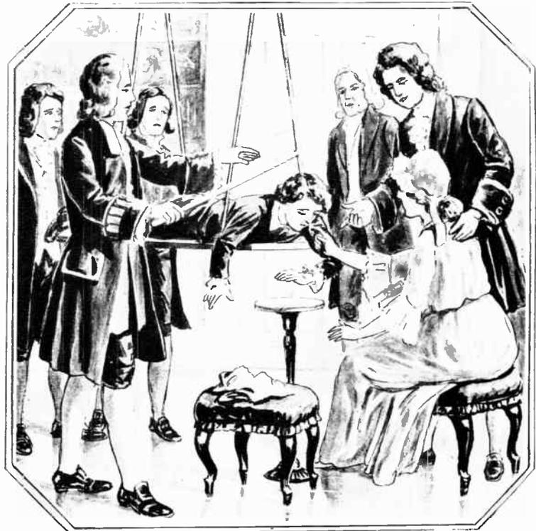
The human condenser, demonstrated by Nollet at the Court of France, is a boy insulated from the ground and charged with an ebonite rod rubbed with fur. When the body accumulated sufficient electricity sparks were drawn from it, and it attracted pieces of paper or other light insulating substances.
