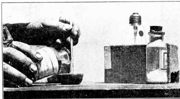
Etching or frosting the glass bulb of an incandescent lamp with hydrofluoric acid; the mixture of sulphuric acid and calcium fluoride supplies the gaseous acid, and the glass will be permanently frosted.
