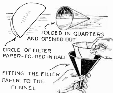
Putting the filter paper in a funnel. This is one way of doing it. Other ways will be described in a subsequent article. The funnel contains water, the little finger of the left hand closing the lower end of the stem.
