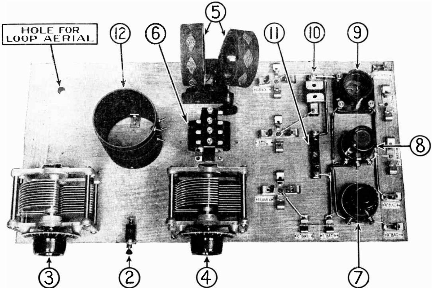
The hook-up board is clearly shown with new instruments mounted on it. The numbers designate the following instruments: 2, crystal detector; 3 and 4, variable condensers; 5, honeycomb coils; 6, amplifying transformer; 7, rheostat; 8, potentiometer; 9, socket; 10, grid condenser; 11, grid leak; 12, oscillator coil. These numbers correspond with those in the other illustrations.
