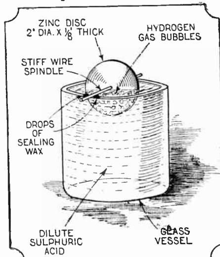
one side than on the other (shown in the diagram by + and - signs), and the side which has the greater "lift" caused by the bubbles will be lifted up and rotation will begin.
