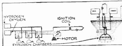
By means of an explosive mixture of oxygen and hydrogen and an electric ignition system sound waves of a predetermined frequency are transmitted over great distances under water. The explosions take place in submerged chambers. An electric motor switches the ignition circuit to the various chambers at the desired frequency.
