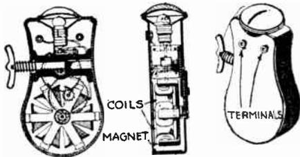
Current is generated for lighting this flashlight by pushing the handle in and out. A train of gears spins a magnet about the coils, causing the generation of current. Terminals are also provided so that the instrument may be used for testing outside lamps, bells, etc.
