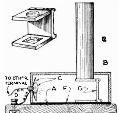
The simple "linen-tester" is there put to novel use as a small microscope. The object viewed is illuminated by a small electric light.
