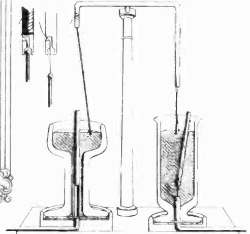
The huge electric motors of the present day are material expressions of the principles involved in the experiment illustrated above. The electromagnetic reaction between a permanent magnet and a wire, carrying an electric current, and dipping in mercury, causes rotation of the wire in the apparatus at right and of the magnet in the vessel at the left.
