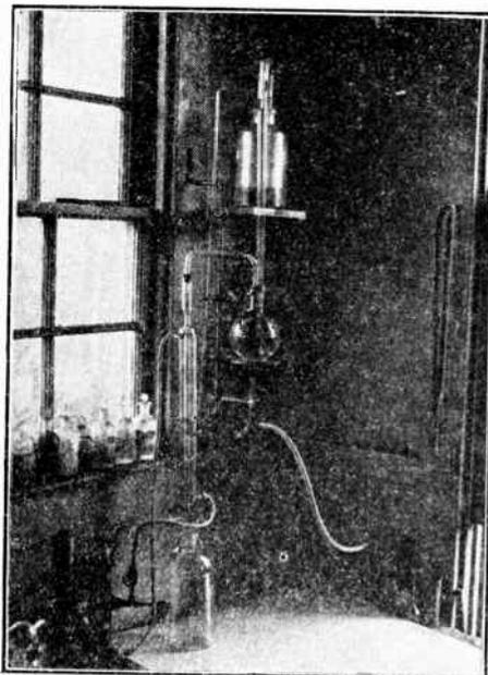
A corner of the writer's laboratory, with a continuous water still set up to supply distilled water for analyses.
