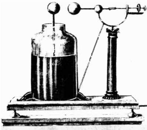
This later form of the Leyden jar is provided with an adjustable spark gap whereby its potential can be measured.
