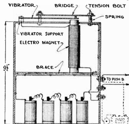
This unique door buzzer, operating on flashlight cells gives signals of unusual volume on account of its mount—a cigar box. Its electromagnet being a dismantled Ford coil consumes very little energy.
