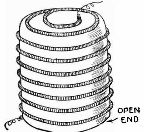
A simply constructed furnace for use in the laboratory. A coil of wire heated by the current produces the heat. It sometimes happens that one has to work in a laboratory without gas.
