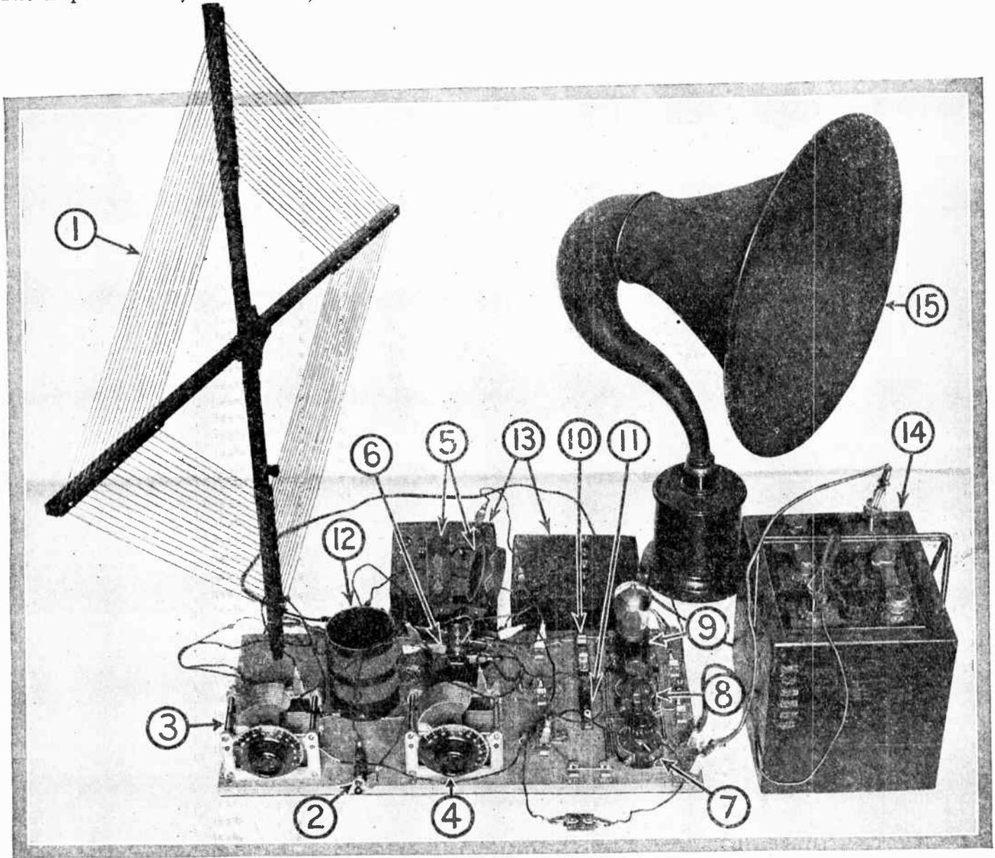
The hook-up board with circuit No. 13, connected. Note the number of connections required for this complicated hook-up. It is one of the best single-tube hook-ups there is, as it operates a loud speaker from a single tube when using a loop aerial. In addition to the instruments shown in our hook-up board illustration the following are used: 1, loop aerial; 13, "B" battery; 14, "A" battery, and 15, loud speaker.
