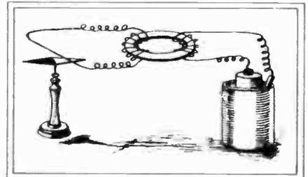
An incipient form of the transformer was constructed by Faraday in his study of electromagnetic induction. Upon closing the battery circuit a current pulse induced in the secondary causes a momentary deflection of the needle.
