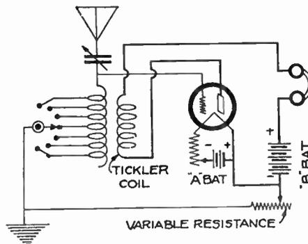
The simplidyne circuit, which is similar to the ordinary single circuit receiver except that no grid condenser is used and a high variable resistance is connected between the filament and the ground. Remarkable results are claimed from this receiver.
