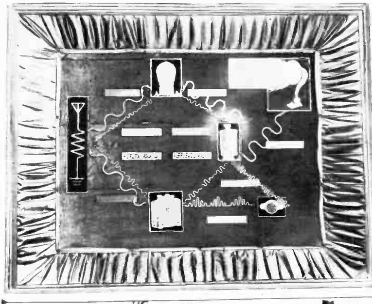
The operation of the reflex circuit is easily understood by the aid of this electrical demonstration board used at the Chicago Radio Show. The oscillations are represented by neon tubes, which become successively illuminated, showing the various stages of both radio and audio amplification and detection.
