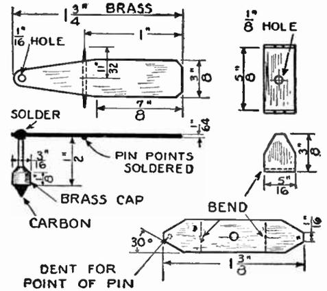
Fig. 5. Details of the parts required for building the microphone relay shown in the other illustrations and also on our front cover.
