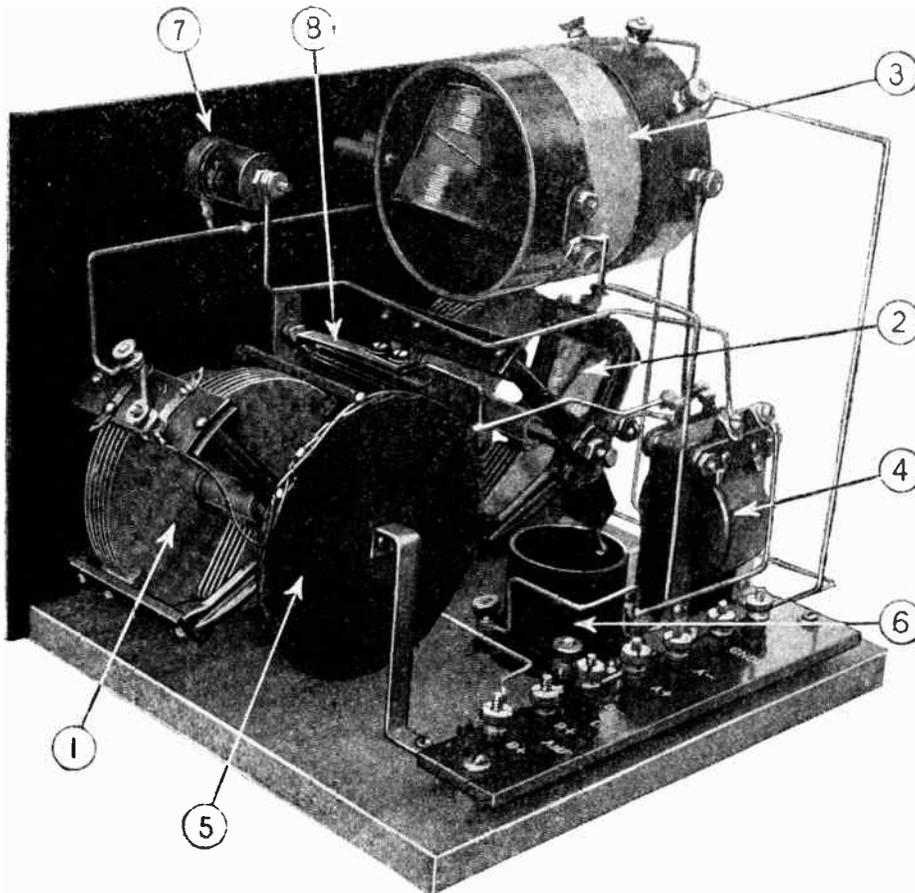
Rear view of the superdynced reflex receiver. The numbers designate the following instruments: 1, plate circuit condenser; 2, grid circuit condenser; 3, tuning coil; 4, audio frequency transformer; 5, plate coil; 6, socket; 7, crystal detector; 8, telephone jack.
