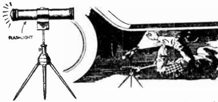
The object of this invention is to provide a suitable stand or support for mounting a flashlight so that it may be placed in any convenient location to facilitate the repairing of motor vehicles, etc.
