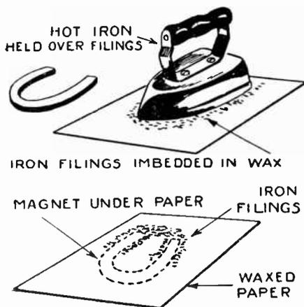
A delicate and transitory experiment is here made permanent. The iron filings disposed around a permanent magnet are made to absorb by capillarity the warm wax covering the paper upon which the filings are spread, fixing them permanently.
