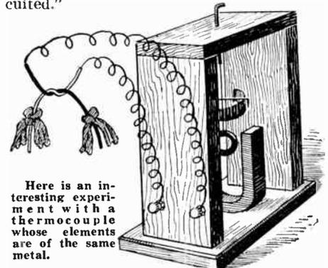
The two terminals at the top connect to a sensitive galvanometer—the lower ones are free, but a piece of cloth or thread is wrapped around each. Then carbon disulphide, gasoline, naphtha or ice cold water is poured on one (the object being to cool it). Boiling hot water is poured on the other cloth.
