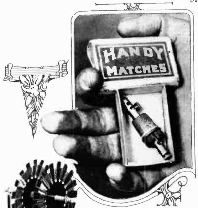
This thimbleful of radio apparatus is a crystal receiving set that fits into a matchbox—and works! It was constructed by a young experimenter, Charles Allen, of Alameda, California, who used it successfully in receiving local stations.
