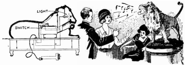
This phonograph is mounted in an ornament form, simulating an animal. By means of a switch a signal lamp indicates through the eyes of the animal when the record approaches the end of its journey, at which time the machine is automatically stopped. A lid in the back allows for exchanging records.
