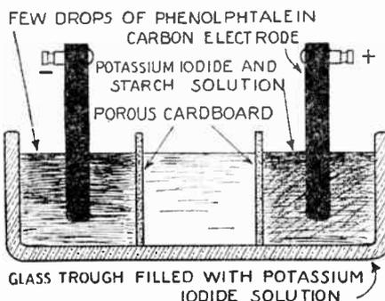
alkali appears in the left hand division and affects the phenolphthalein. This gives the red. The central division determined by the porous paper, is unaffected. The
