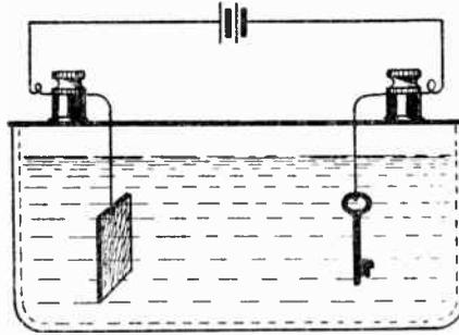
Electrical analysis of a key. This is a very pretty experiment, involving the deposition of copper from the key and weighing of the same. If the key is of true brass the difference will be zinc.
