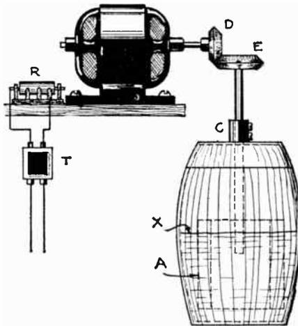
The electric motor drive in connection with the improvised churn, it may be from a Mason preserving jar, illustrated above, adapts the device to daily use in the city home.
