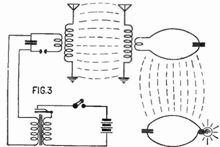
Here is a way of converting electromagnetic into electro-static vibrations, according to our author.
