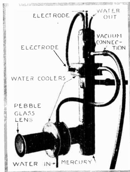
This shows a vacuum mercury arc lamp with quartz lens for emitting ultra-violet rays.
