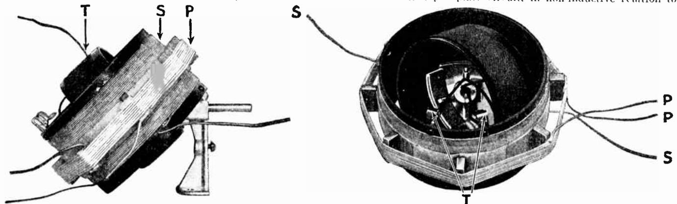
Fig. 5. An unturned primary coupler that has given excellent results in Mr. Pearce's experiments with radio frequency amplifiers. Note how well the primary is spaced from the secondary so as to reduce electrostatic coupling between the two windings.
