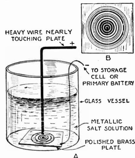
The beauty of this fascinating electro-chemical experiment is enhanced by the facility with which it is produced, a metallic salt solution and a storage battery being the only requisites.
