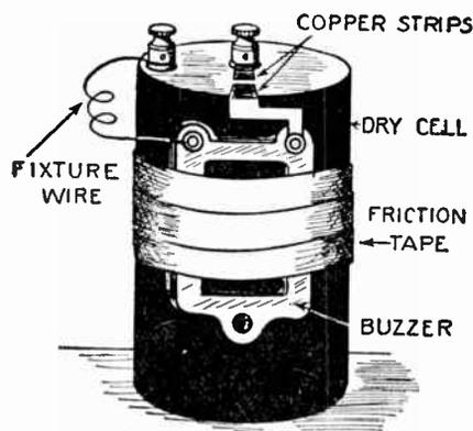
it thoroughly practical. The voltage of a single cell would not show by its effect on a lamp, but enough current will go through the circuit to operate the buzzer.
