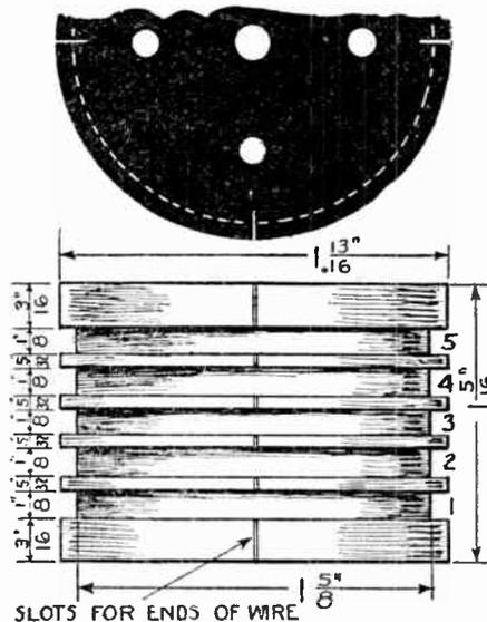
Wooden form for constructing the Rasco radio frequency transformer. The experimenter may turn this form out on a lathe and wind the coils according to the directions given in the text.
