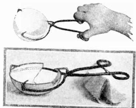
Improved chemical tongs. In the lower view the dish is broken away to show how the tongs grip it. Note rubber band.
