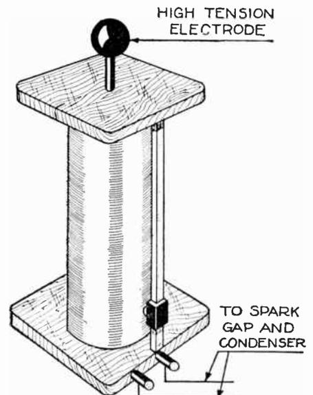
A simple and effective form of that endless source of electrical experiments, the Oudin coil, is shown above. It is constructed on the core of an old "tuning coil."
