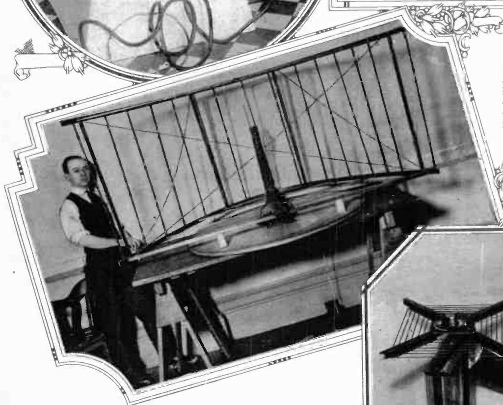
Directed transmission, while still in its experimental stage promises success with this parabolic reflector for radio waves; devised by Marconi.
