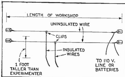
A sort of two or three trolley wire circuit for the laboratory; currents can be taken off as desired.
