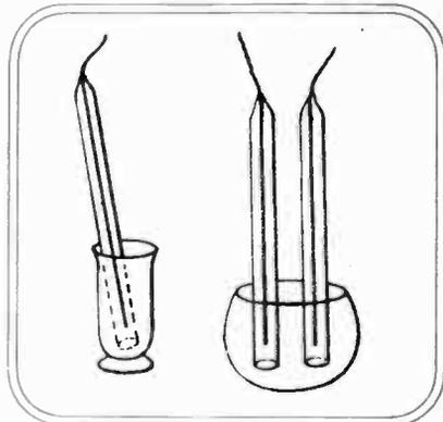
Many of Faraday's experiments were concerned with electrolysis. His apparatus for decomposing water embodies the unusual feature of separating the electrodes at the sealed top of the tubes, rather than through the open bottom, as done by modern experimenters.
