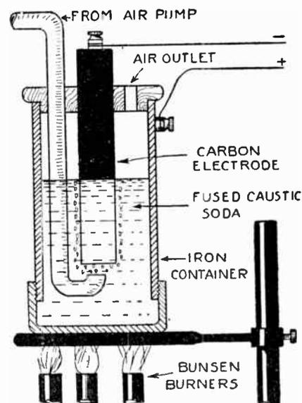
Experimenters with a taste for strange apparatus should try this "wet" cell which functions through the simultaneous operation of Bunsen burners, an air pump and a chemical reaction.
