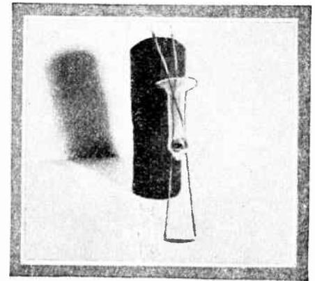
The apparatus on the left are home-made power vacuum tubes, ingeniously assembled from iron pipes and the anchor leads of burnt-out incandescent lamps. The necessity for the water coolers testifies to the magnitude of the power delivered by them.
