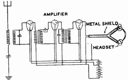
In many radio receivers the telephone cords cause difficulty in tuning due to electrostatic feedback. This invention provides for shielding the cords with a suitable metallic shield connected to the filament circuit of the apparatus.
