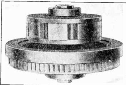
The small turbo-generator used to supply power for miners' lamps has a pneumatic-turbine rotor and a rotary permanent magnet for the generator field, mounted on the same shaft.
