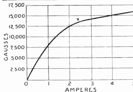
The graph illustrates the variation of magnetic density in an iron specimen with variations in the current through the electromagnet. Such graphs are at the basis of all dynamo design.
