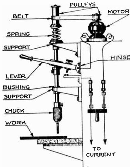
An electric drill, readily constructed from odd parts. The motor is automatically started when the drill point is lowered to its work, the handle, when pulled down, closing the circuit.
