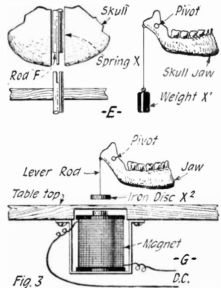
Fig. 1 shows the general layout of this rather startling experiment, the skull grimly opening and shutting its jaws and performing the other motions as described. Further details are given in Figs. 2 and 3, the whole thing constituting an interesting if somewhat ghastly display. The motor revolving a disc, operates the circuit breaker, affecting the magnet periodically. A relay is employed to give good actuating current.
