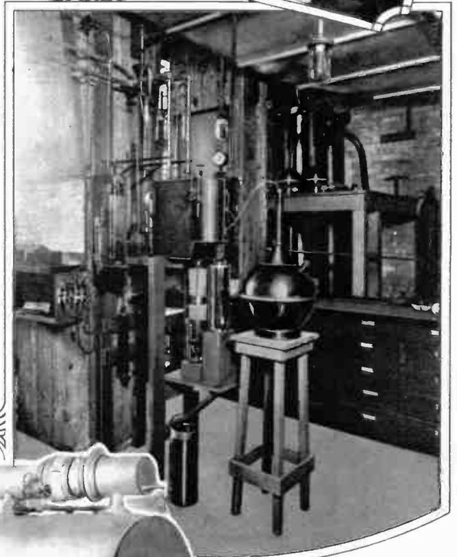
Due to the extremely low temperature required, attempts to liquefy helium gas have proved unsuccessful until Prof. J. C. McLennan of the University of Toronto, Canada, with the apparatus shown above, succeeded, after two years of patient experimentation, to reduce the gas to a liquid at a temperature of 269 degrees Centigrade, below zero.
