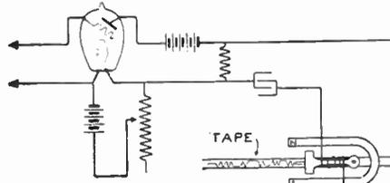
A resistance is connected in the output circuit of the receiving apparatus, the variation in potential drop due to the received signals causing a current flow through the condenser and recorder. A stylus records the signals on a moving tape.
