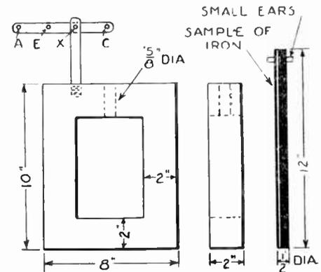
These details show the utter simplicity of the magnetic density tester. The frame recommended by the writer is of cast iron, but the core of a discarded closed-core transformer may be used with advantage.
