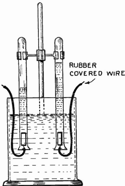
Electrolysis of water; the radio operator's spaghetti would be a convenient covering for the wires, if rubber insulated wire is not at hand.
