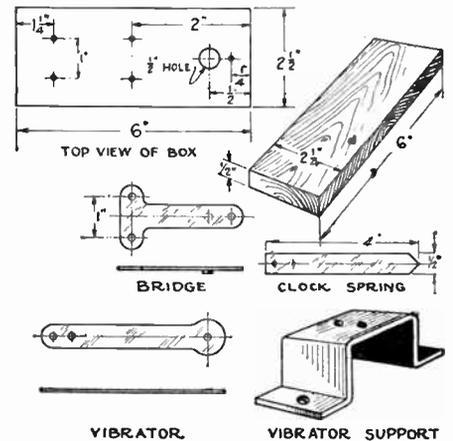
Principal details of the flashlight-cell door buzzer; all readily constructed even by the least skillful experimenter. The parts besides the cigar-box wood are odd pieces of sheet metal.
