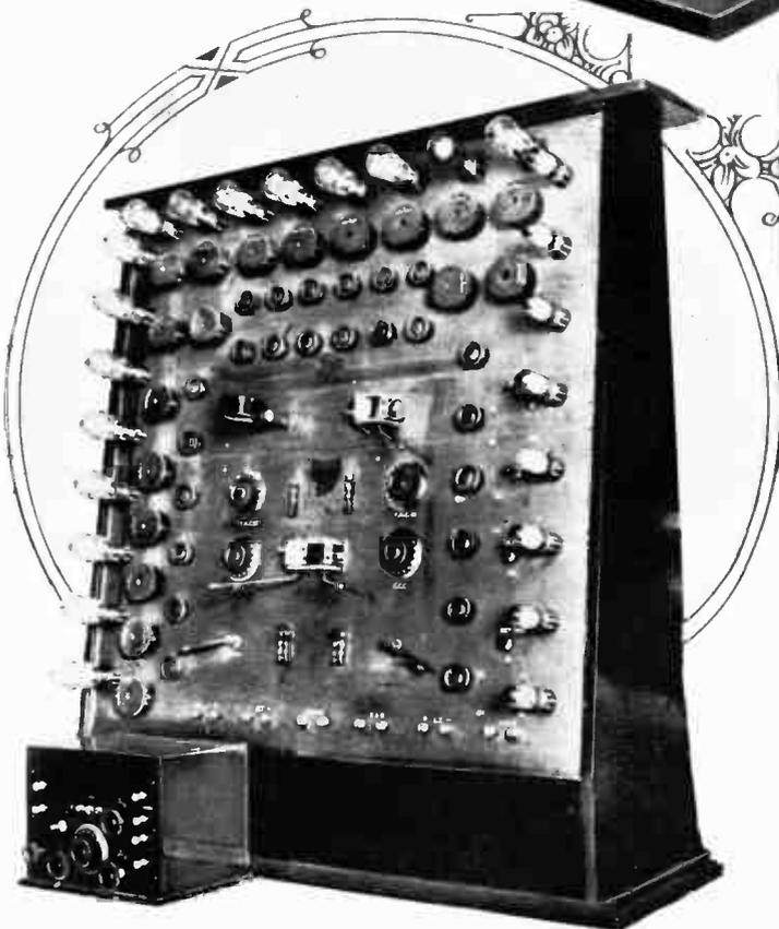
Six months of patient research on the part of British radio engineers have resulted in this 24-tube radio receiving set, specially designed to pick up communication from Mars. Compare with the ordinary two-tube set at left.
