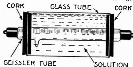
No extraordinary apparatus is required for converting the ordinary Geissler into the fluorescent type. A glass tube surrounding the Geissler tube contains the necessary fluorescent liquid.
