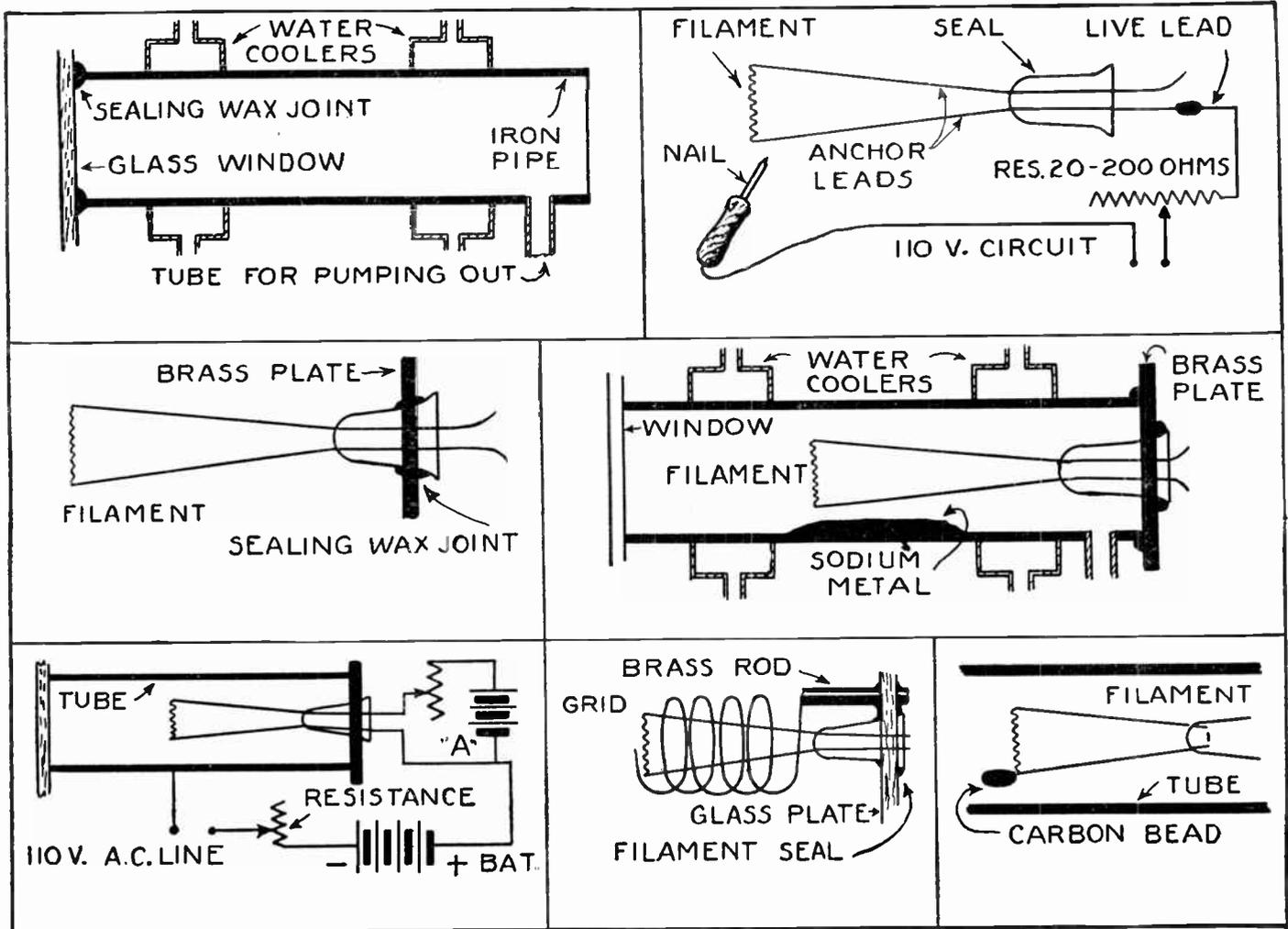
These detailed drawings remove many difficulties in the construction of the power vacuum tubes. Besides structural details the diagram indicates an interesting method of evacuating the tube. By heating sodium in the tube the residual oxygen is finally removed.
