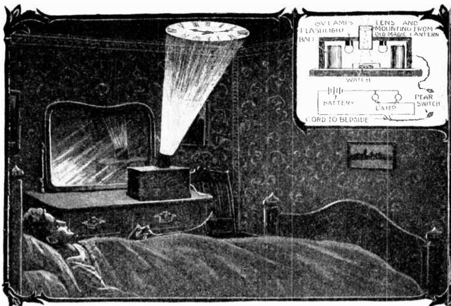
That laziness rather than necessity is the mother of invention is demonstrated by this ingenious device by means of which you can see the time indicated by your watch at any time in the night, without inconvenience. A pear switch lights two lamps in the case, whereupon an image of the illuminated dial of the watch is cast on the ceiling.
