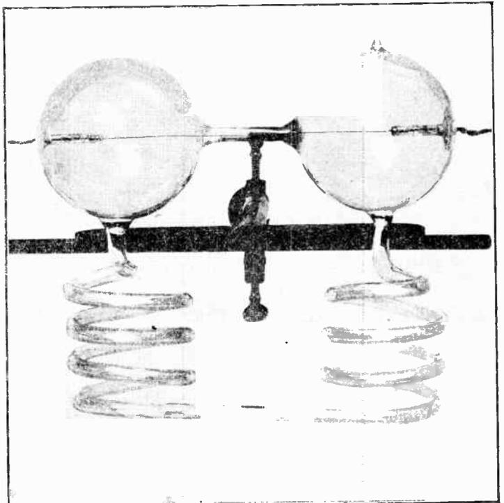
That electrical discharges do not always follow the shortest path can be demonstrated by the tube shown above. Hittorf using a high vacuum tube with 1 mm. between electrodes and with the helical tube 375 cm. long, found that at certain potentials the discharge showed decided preference for the longer path.
