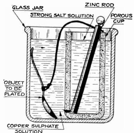
An easy copper plating experiment that may have useful applications about the laboratory and in the household. The use of a porous cup is its characteristic feature.
