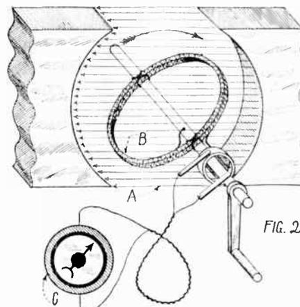
Here lines of force are so cut that the number traversing the coil changes, thereby generating electric potential as shown on the voltmeter.
