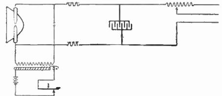
This signaling apparatus comprises an arc light connected to a D. C. line in series with suitable chokes and resistances. A condenser is connected across the line. Pressing the key energizes the spark coil, thus breaking down the resistance of the gap between the electrodes and allowing the condenser to discharge, giving an intensive flash. The flow of current stops after the condenser is discharged.
