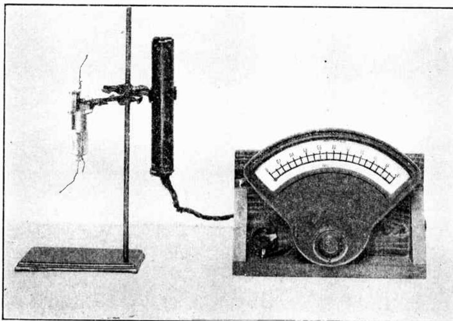
The current through a coil of wire wound around a cylindrical two-element vacuum tube may, by its magnetic field, prevent the electrons from reaching the plate. In the tube shown the magnetic field is made equal to that of the earth, and by rotating the tube the two fields may be brought into combined action; the milli-ammeter showed various currents. The intensity and the direction of the earth's magnetic field is thus determined.
