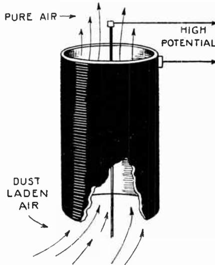
The Cottrell electrostatic precipitator, shown above, induces an electric charge in the solid particles carried by gases and then retains these particles on one of the electrodes. The process can be readily duplicated by the amateur experimenter.
