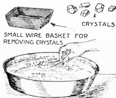
Crystallization; as the crystals form they may be removed by a little wire basket. If solution of table salt is used very beautiful basket-shaped aggregations of crystals are produced.
