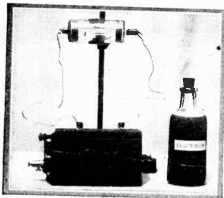
If the manufacturer has not provided fluorescent material within your Geissler tube, you can compensate for the deficiency by this ingenious method of surrounding the tube with fluorescein.
