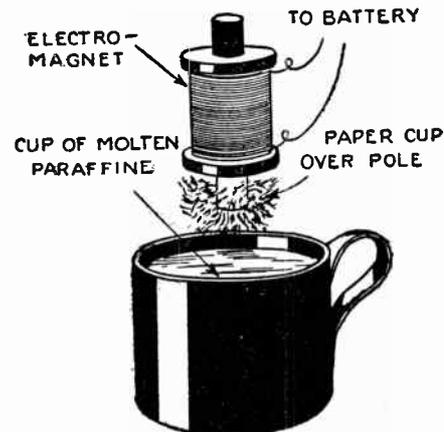
The field around the end of a bar magnet can be shown in striking relief, by immersing the cluster of iron filings formed on a card-board cylindrical case placed on the end of the magnet, in melted wax; after withdrawal and cooling it is permanent.
