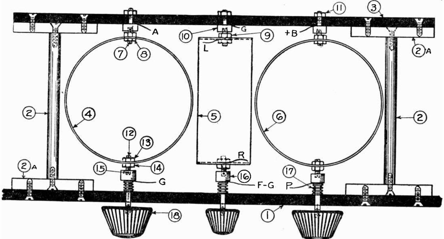
Amateur transmission and reception on wave lengths less than 100 meters have brought forward many new designs in receiving apparatus. This short wave tuning unit comprises primary, secondary, and tickler coils. By pulling the knobs out the inductances may be removed and different size coils substituted. Thus the entire amateur wave length bands may be covered.
