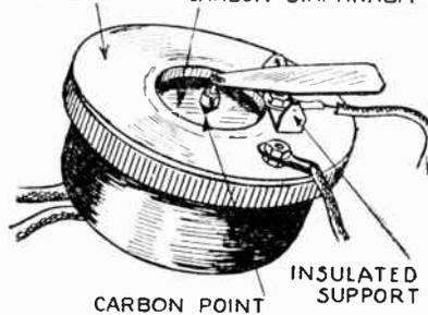
Fig. 4. Assembling drawing of the microphone relay shown in the photograph. The finished instrument should be mounted in a sound-proof box to prevent feed-back howling from the loud speaker.
