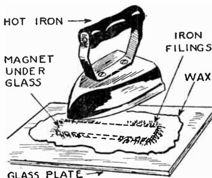
Another method of retaining the formation of iron filings is illustrated above. By the use of a heavier layer of wax upon a plate of glass and a stronger magnet, the field is better shown.
