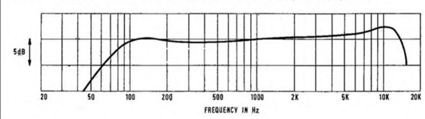
FIG. 4 PHILIPS 4307 ACOUSTIC RESPONSE (WHITE NOISE TAPE ON SPEAKER AXIS)
