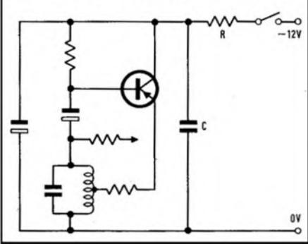
**FIG. 41** METHOD OF IMPROVING LINEARITY OF SAWTOOTH OSCILLATOR BY PROVIDING A HIGH CHARGING VOLTAGE
