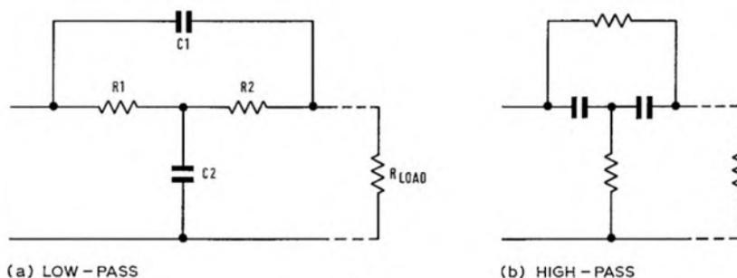
**FIG. 48** (a) PASSIVE TWIN - T RESPONSE
