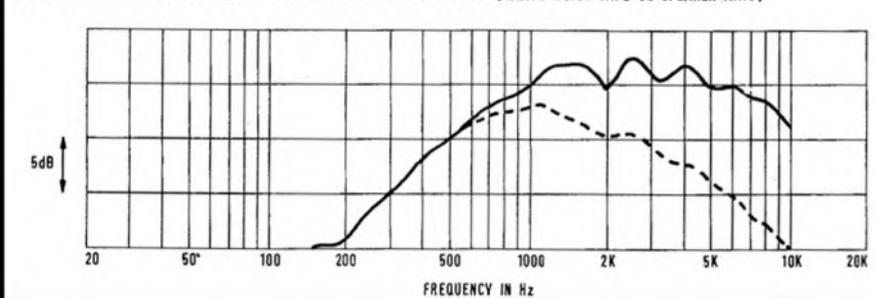
FIG. 5 PHILIPS 4307 MOVING-COIL MICROPHONE (500 OHMS IMPEDANCE)
