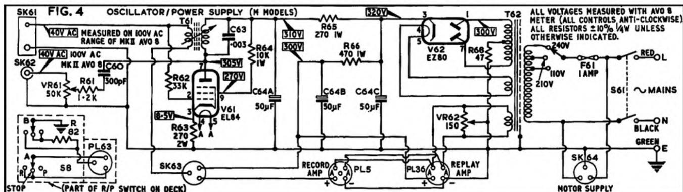
Switches themselves are easily cleaned on these models, and do not give a great deal of trouble. The rest of the R/P/A switching is fairly self-evident, consisting of coupling from V2B to V3 and the addition of the feedback loop from the output to the cathode of V2B, with an extra 220 ohms in the cathode of this triode on playback and amplification.
