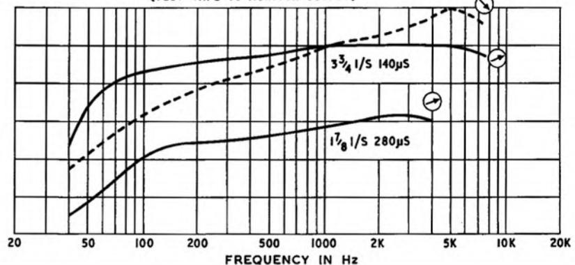
FIG. 3 SONY TC800 RECORD/PLAY RESPONSE (AUXILIARY INPUT TO MONITOR OUTPUT)
