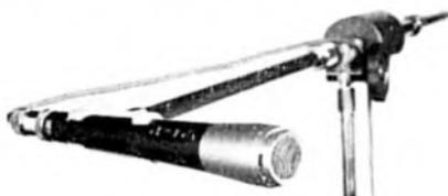
Frequency response (to -2dB points) is from 70 c/s to 16 Kc/s, and sensitivity (30-50 ohms impedance) is 88dB below 1V/dyne/cm<sup>2</sup>. Polar response is omni-directional, partially suppressed at the rear. The low-impedance *CPDL* retails at £15, while the medium and high impedance *CPDM* and *CPDH* are £16. A non-switched *CPDL*, is available at £14. Manufacturer: Reslosound Ltd., 24 Upper Brook Street, London, W.1.
