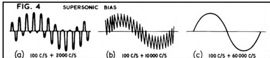
and 2 Kc/s are superimposed in a record head. We can see that the result is a high-frequency recording whose average amplitude varies at the lower frequency. There is no low-frequency distortion because the magnetic field is alternating too rapidly for the low frequency transfer-characteristic to apply.
