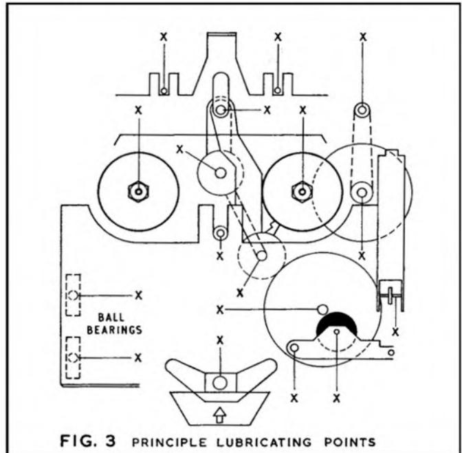
The main lever has a guide roller, held by a nylon circlip, which pushes the plate forward. The plate sits on ball-bearings in small channels of the deck plate and its position is regulated by two spring rollers (see fig. 2) which engage in cut-outs of the moving plate. Possible faults here are loss of ball-bearings after over-enthusiastic dismantling, loss or incorrect remounting of rollers, looseness of spring clamps and just plain breakage due to an attempt to increase tension by bending.
