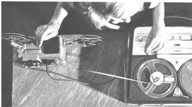
**Above:** Philips tape recorder controlling speed of Eumig projector through Eumig Phonomat attachment. **Below:** Basic set-up for recording commentary at a distance from the projector and recorder. Microphone is positioned a foot from the commentator on sungun camera bar. In front of her is cue lamp, controlled by projectionist.
