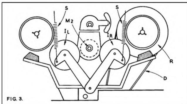
is simply pressed into rubber grommets. It is necessary to hold back the pressure pads with the fingers when removing and replacing the arm, and to ensure that the tension spring at the right-hand end is properly located after re-assembly.
