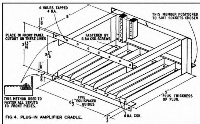
FIG. 4. PLUG-IN AMPLIFIER CRADLE.
