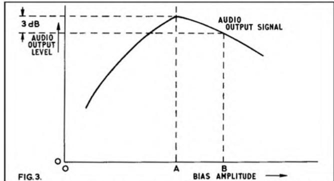
**Fig. 3.** The optimum bias setting taking into account signal-to-noise ratio and distortion should be determined aurally. The best setting will normally be found somewhere between A and B; i.e. a slightly higher bias level than that giving maximum recorded signal level.
