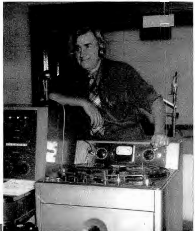
Above, Charles Nehlsen, usually called "Nelly," who spends much of his time supervising the making of recordings. Originally a recording had to be made on a disk or "platter," and many are still made that way. However the tape recorder now gives such perfect results that it equals the natural voice in quality. Words or music are impressed on the tape by magnetic effect, with no mechanical change. The use of recordings gives much greater flexibility in program planning. Nehlsen, a precision worker of great skill, listens to hours of speech and music every day, but is one of the quietest men in the place. Shown here monitoring a control-room tape recorder.
