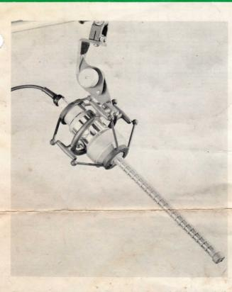
The Cardiline\* Model 642 is a highly directional dynamic microphone utilizing a combination of the characteristics of cardioid and distributed front opening designs. The cardioid action gives the microphone essentially unidirectional characteristics at frequencies up to 500 cps. At this point the distributed front opening takes over for the balance of the range to which it responds providing directional characteristics illustrated in the polar diagram, Figure 3.
