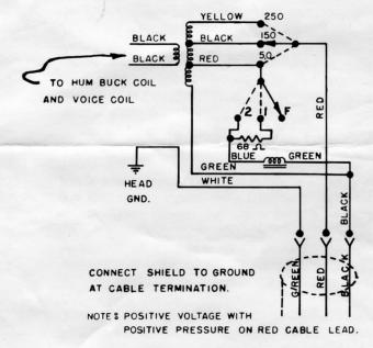
Figure 4 - Wiring
