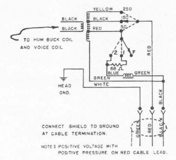
Figure 4 - Wiring
