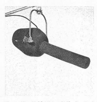
The Cardiline Model 642 is a highly directional dynamic microphone utilizing a combination of the characteristics of cardioid and distributed front opening designs. The cardioid action gives the microphone essentially unidirectional characteristics at frequencies up to 500 cps. At this point the distributed front opening takes over for the balance of the range to which it responds providing directional characteristics illustrated in the polar diagram, Figure 3.
