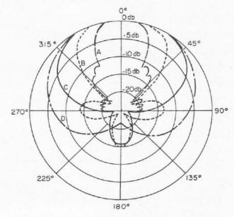
A-10,000 cps C-1,000 cps B- 2,500 cps D- 100 cps Figure 3 - Polar Pattern
