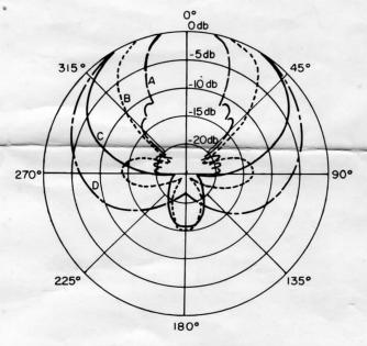
A-10,000 cps C-1,000 cps B- 2,500 cps D- 100 cps Figure 3 - Polar Pattern
