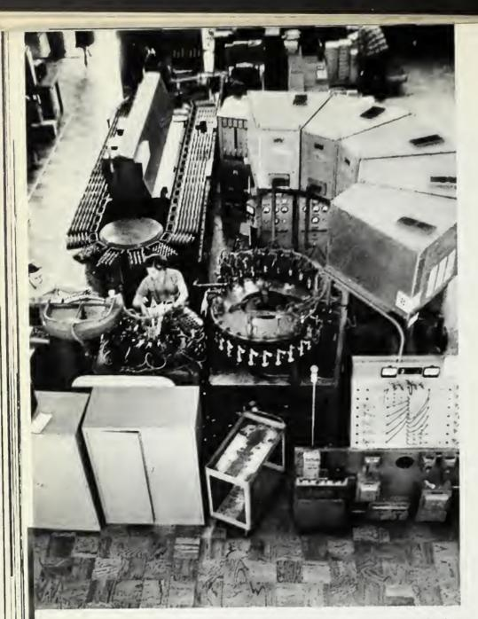
Vacuum tube assembly involves automatic machine aids, but key processes are in human hands of extraordinary dexterity. ABOVE: Sealed vacuum tubes are fed at high speed to conveyor belt. BELOW: Nimble fingers skilfully, speedily assemble tiny tube parts.
