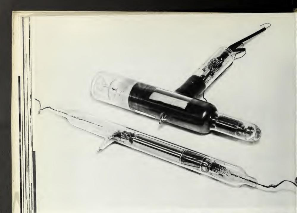
ABOVE: Special equipment for testing CBS Laboratories-developed low-friction vacuum bearings for use in high vacuum, as in outer space. The new bearings extend very substantially the effective life of instruments that operate in a high vacuum. RIGHT: Color-television ophthalmoscope permits examination of eye's circulation, as image is simultaneously recorded on film for further study. Picture below shows human retina as seen on television screen.
