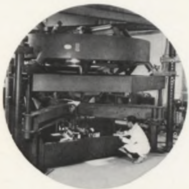
Mechanical balance produced by Dynametrics to measure forces on aircraft and missiles.
