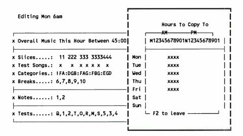
When you have marked the elements to copy and the days/hours to copy to, press the F2 key to execute the copy. You may exit, without copying with the esc key.
