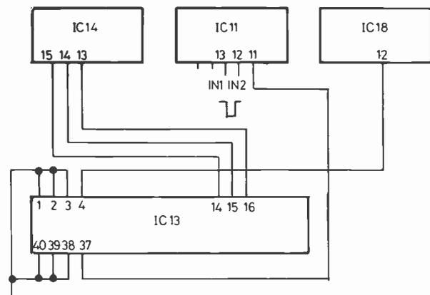
Fig. 7 PROCESSOR TO SPEED CONTROLLER CONNECTIONS
