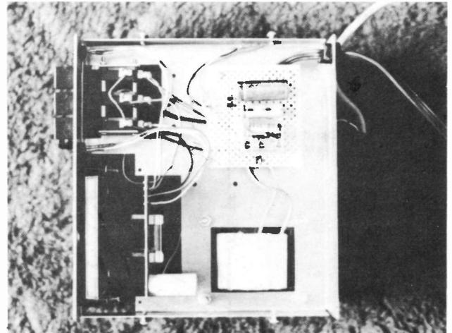
David Jolly, G3TJY, sent us this photo, as a satisfied user, of an L.J.E. D-LAY-5 rotor brake delay, fitted to his Ham II control box. Designed for C.D.E. rotors, Models CD-44, CD-45, Ham II, Ham III and Tailtwister, G3TJY says he finds it invaluable, automatically delaying brake action for 5 seconds. Full details of the D-LAY-5, which costs around 20 U.S. dollars, are available from Lance Johnson Engineering, P.O. Box 7363, Kansas City, Mo. 64116, U.S.A.
