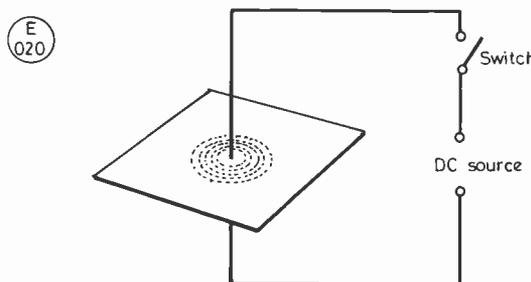
Fig.1(a) Iron filings round a wire carrying current indicate the direction of the magnetic field relative to the wire.
