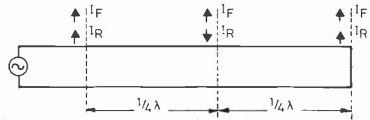
Fig 2(e) Short circuit end to Transmission line
