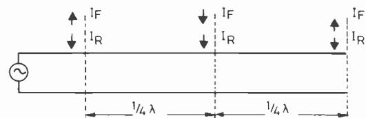
Fig.2(d) Open circuit end to Transmission line (See also Fig.2(f)).
