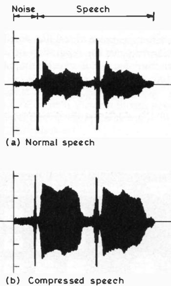
Fig.1 MODULATED SSB RF ENVELOPE
