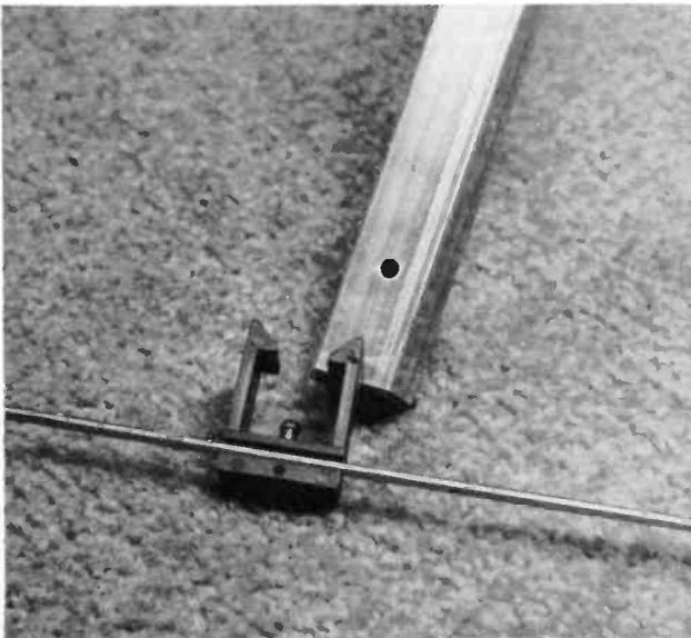
Close up of the plastic clip with element inserted, showing key which positively locates the assembly into the hole pre-drilled in the boom.
