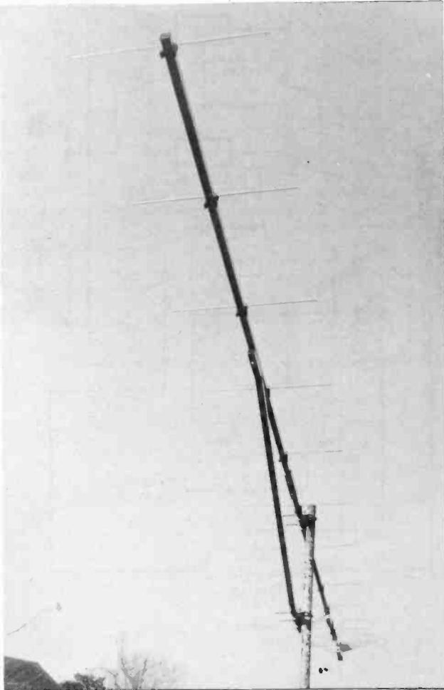
General view of completely assembled aerial. The overall boom length is 2.68 metres. The splice can be seen just in front of the mast.
