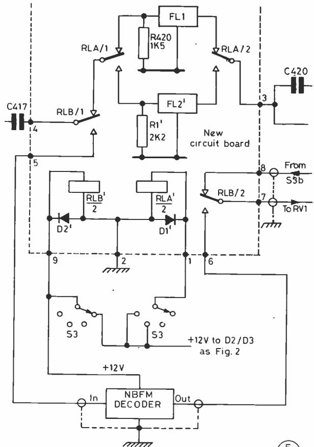
Fig. 3 COMPLETE CIRCUIT
