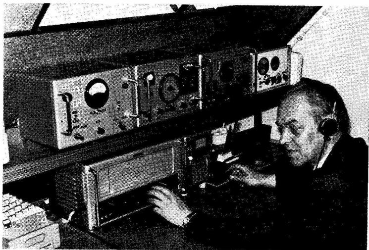
The station of Fritz Cramer, DL3MO, 4420 Coesfeld, Schuppenstrasse 22, Westphalia, near the Dutch border. Fritz started on the air in 1949, runs CW with an electronic key, and AM phone. The Tx is a home-built five-band job covering 10 to 80 metres, with a multi-band dipole outside.
