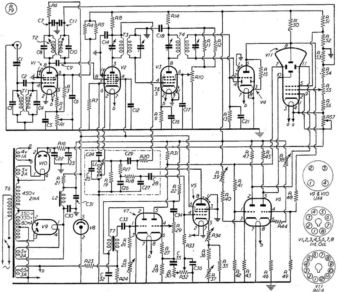
Fig. 5. Circuit complete of the panoramic adaptor unit ("panadaptor") described in the accompanying article. The frequency modulator section is enclosed in the dotted square, and all values are given in the table herewith. (Note: T5 is represented by the FM section).
