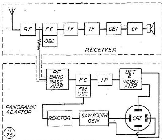
Fig. 2. Block schematic of the unit layout for a Panoramic Adaptor, which can be used with almost any receiver. The lower section is all covered by the circuit of Fig. 5.
