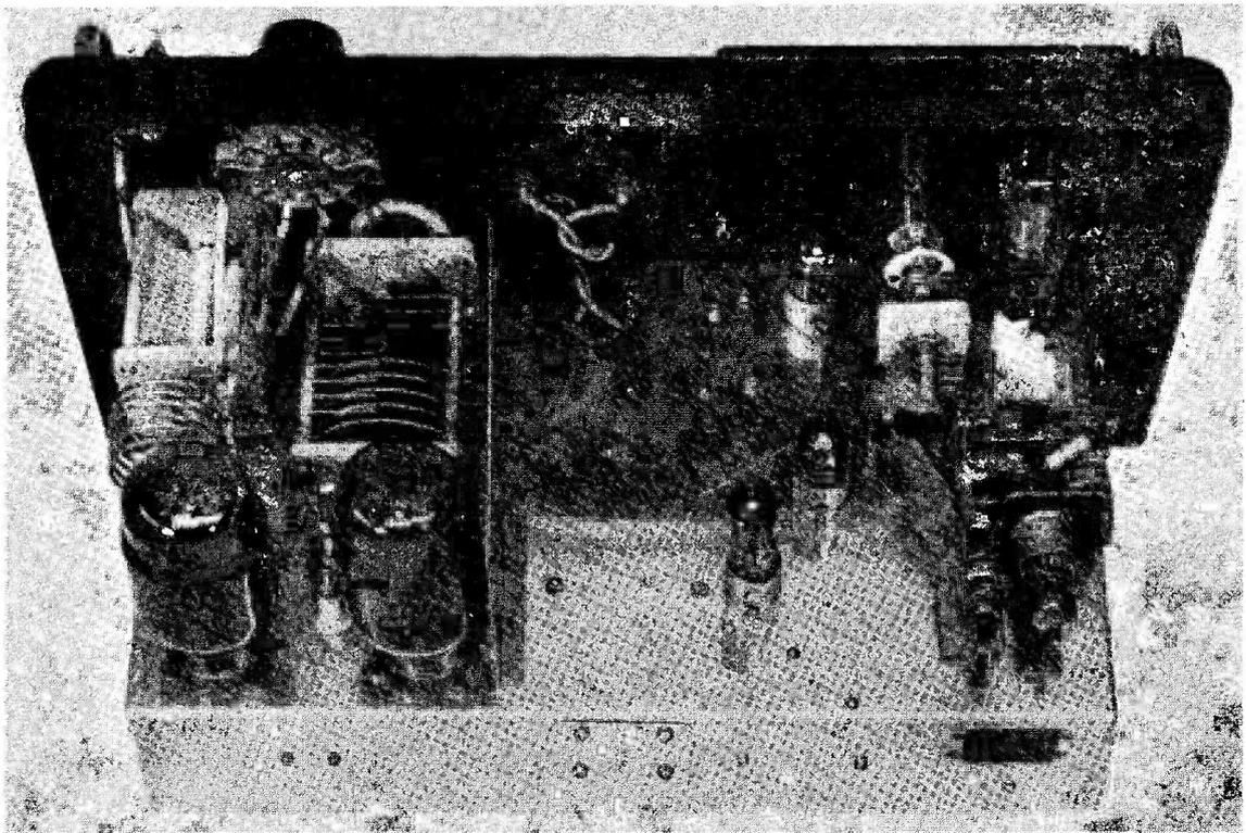
Rear chassis layout of the 14/21 mc band-switched transmitter, which runs Osram valves throughout with a pair of KT66's in the PA stage (left). This view shows many constructional details.
