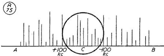
Fig. 1. Showing a section of the sweep obtained, over 200 kc of any band, with the panadaptor described in this article.
