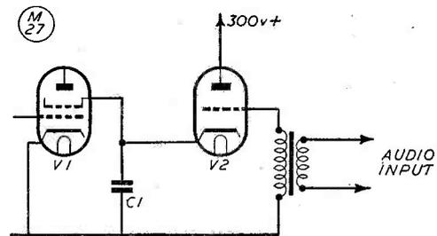
Fig. 1. The principle of screen modulation. V1 is the modulated stage, which can be an 807, 813, 829, 832 or similar; V2 is the modulating valve, such as a 6V6 or anything of that type; and C1 is the screen by-pass condenser, of some value between .0005 and .005  $\mu$ F.
