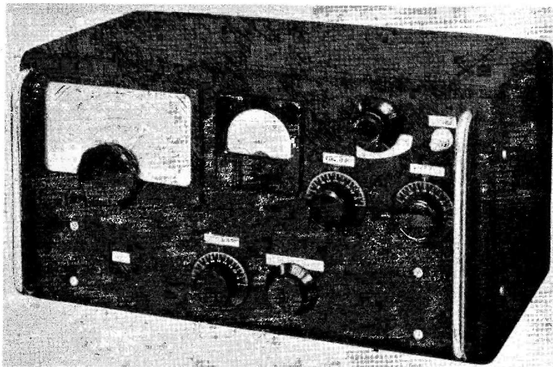
Exterior view of the VFO-controlled band-switched 14/21 mc transmitter. It gives about 60 watts of RF output with 500v. HT on the plates of the KT66's in the PA stage.
