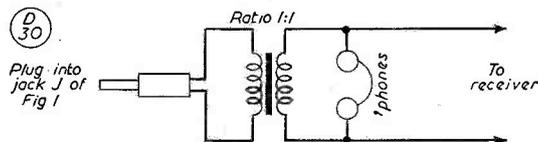
Fig. 2. Alternative output coupling circuit, permitting simultaneous monitoring and listening.
