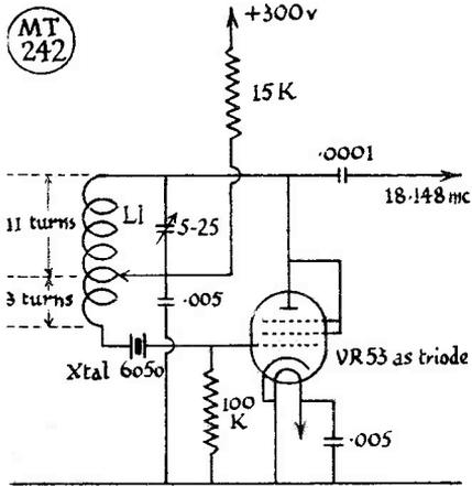
Fig. 2. This is the circuit to use for getting out the 3rd overtone of the crystal, proper choice of which will eliminate the possibility of generating harmonic frequencies falling in the various TV channels, as explained in detail in G2JU's article. Assuming this oscillator is required to drive a 2-metre transmitter, the final frequency could be about 145.18 mc. Coil data : L1, 7/8-in. former, wound with 14 turns of 26 SWG over 3/8-in. and tapped at the 3rd turn.
