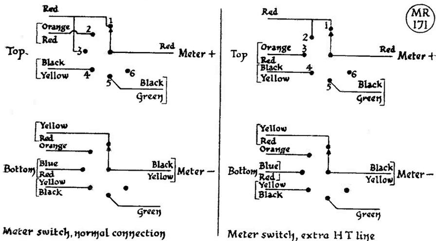
Fig. 4. The switching detail referred to in the text. The colour codings will identify the leads.
