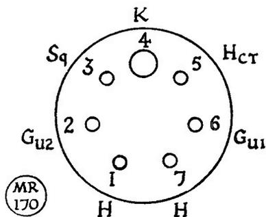
Fig. 3. Base connections of the 832 used in the BC625A.
