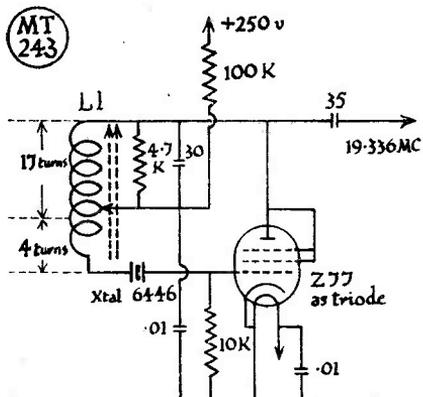
Fig. 3. It is just as necessary to choose the right frequency for the CO stage of the 2-metre converter. With an oscillator frequency of 19.336 mc, multiplied to approximately 116 mc, a tunable IF of 28-30 mc would be produced in the 2-metre receiver. In this case L1 is a 3/8-in. former wound with 21 turns of 26 SWG over 1/2-in., tapped at the 4th turn. The coil is fitted with an adjustable dust-iron core.
