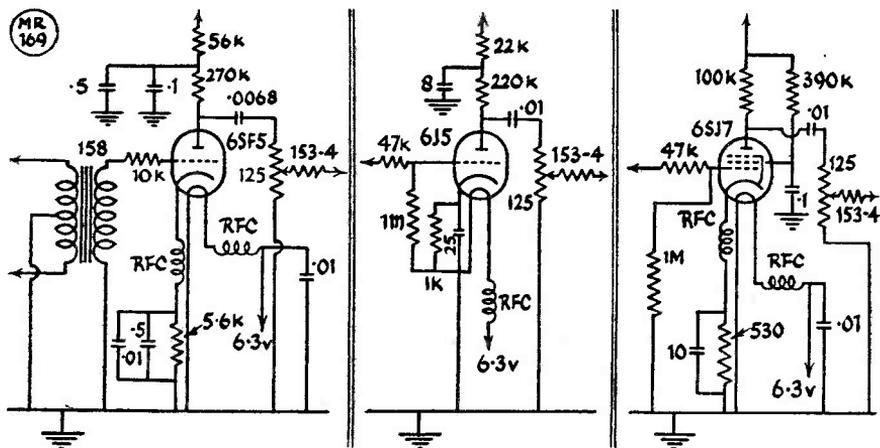
Fig. 2. Three possible methods of wiring in the additional speech amplifier, depending upon what type of microphone and 1st audio stage valve are to be used. In each case, RFC is 20 turns of No. 28 SWG enamelled wire on a 1-watt resistor as former.
