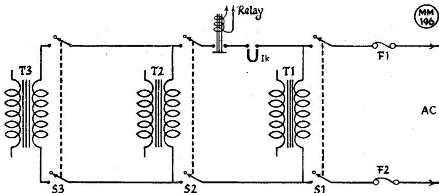
A simple switch-for-safety wiring diagram for the power supply units. Each transformer—filament, exciter HT and PA HT—is controlled through DPDT switches S1, S2 and S3, which can only be made in that order. Additional safety is ensured by the mechanical interlock Ik, while the relay can be wired for remote switching of the HT supplies from the operating position.
