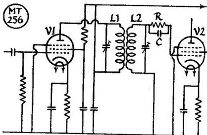
Fig. 3. An alternative circuit to that of Fig. 1, suitable for broad-band couplers used in intermediate stages. R can be 22,000 ohms and C 100  $\mu$ F.
