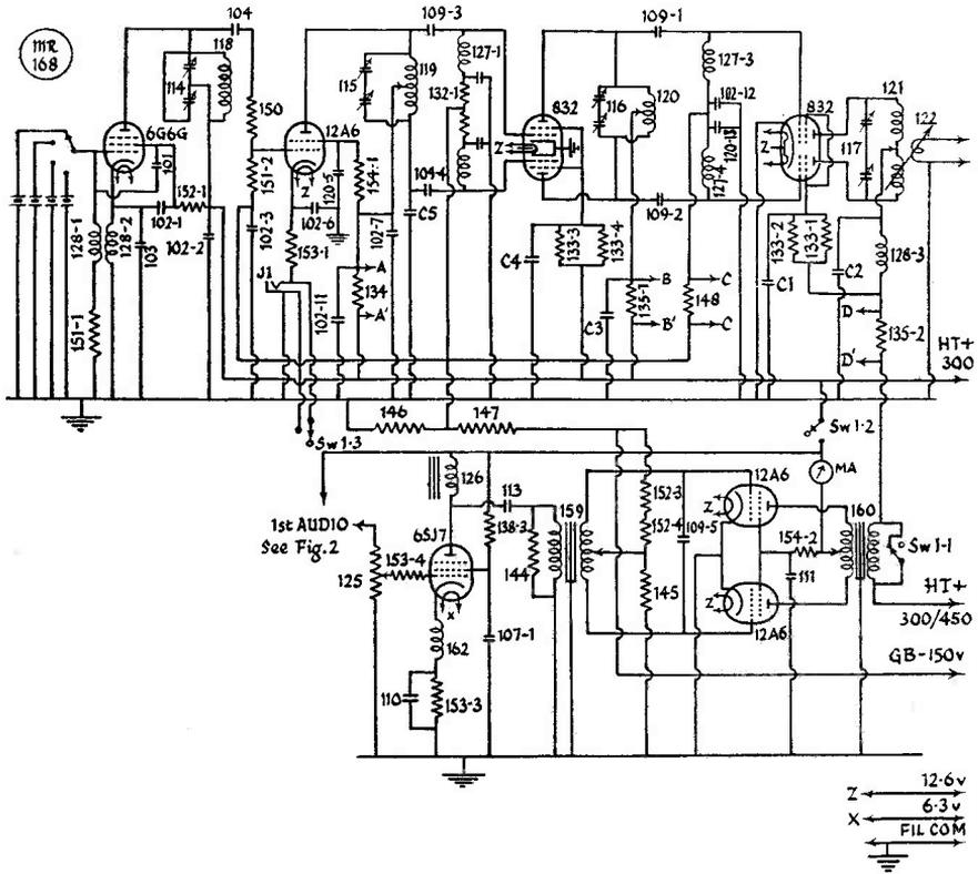
Fig. 1. Circuit complete of the BC-625A, transmitter unit of the SCR-522, with circuit elements numbered in accordance with the original Service annotation, except where stated. All values can be checked by reference to the accompanying table.
